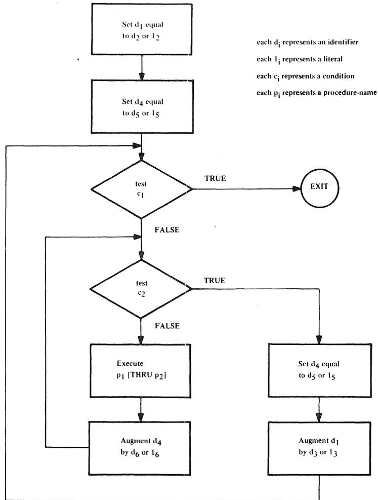
The following flow chart illustrates the logic of the PERFORM cycle when three identifiers are varied.
