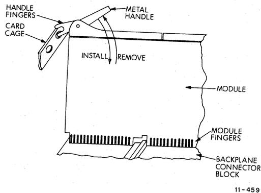
**Figure 2-2 Module Installation**
