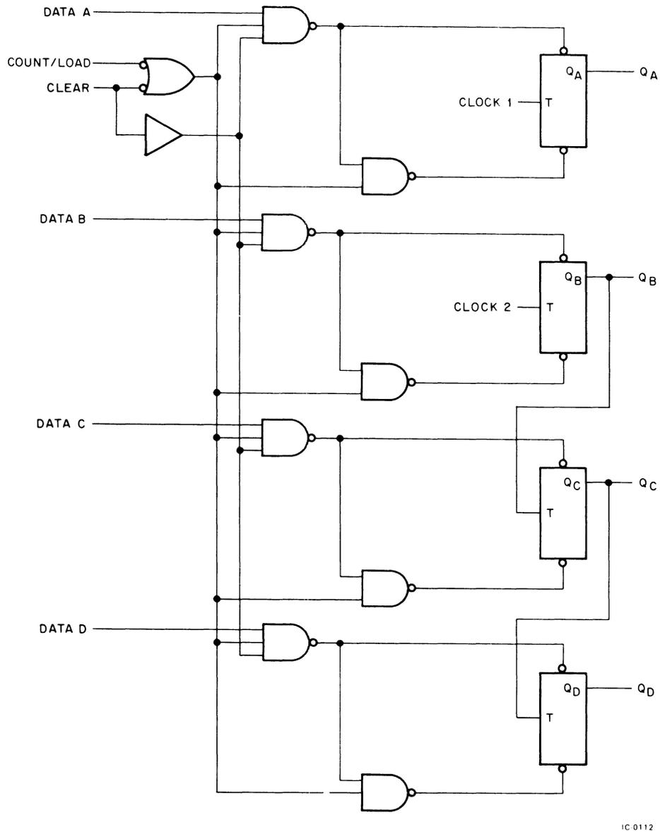
Figure B-4 74197 Logic Diagram (Sheet 1 of 2)
