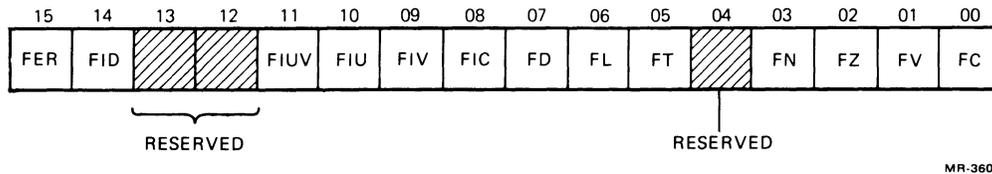
Figure 7-4 Floating-Point Status Register
