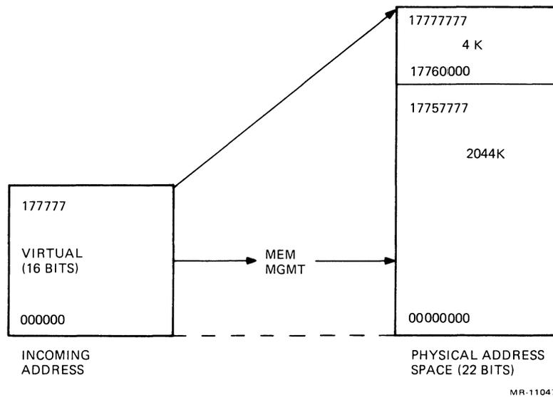
Figure 1-9 22-Bit Mapping
