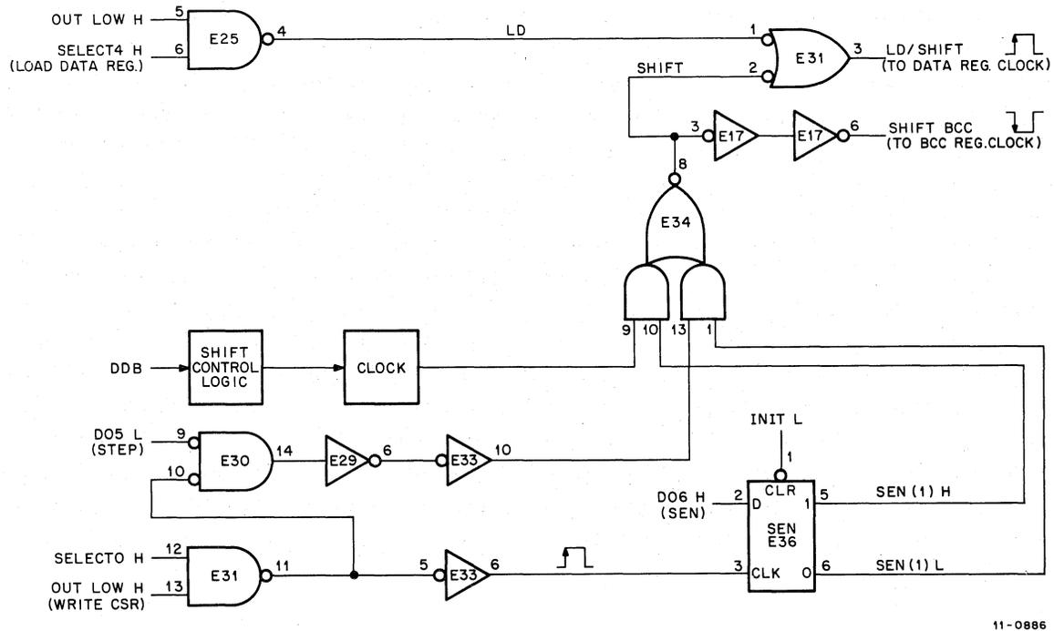
Figure 3-12 STEP and SEN Control Signals, Logic Diagram
