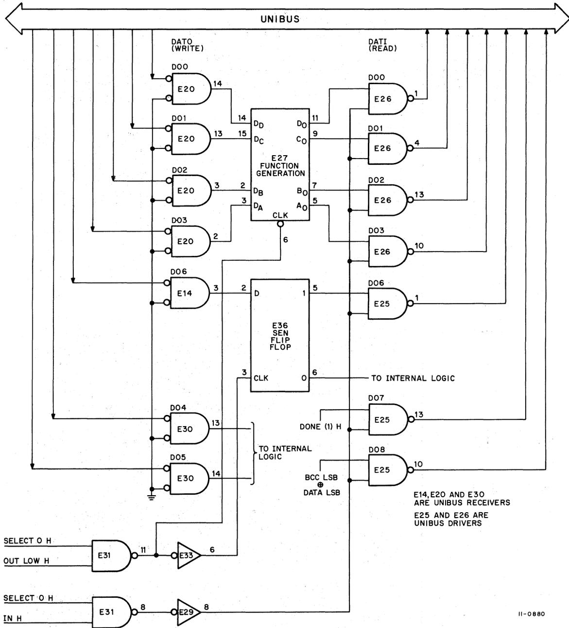
Figure 3-6 Control and Status Read/Write Functions, Logic Diagram
