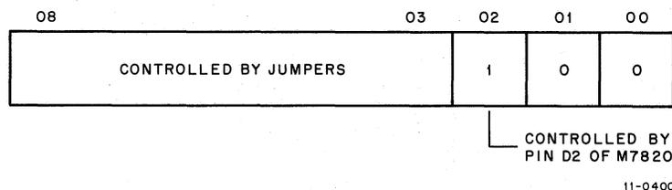
Vector address bits (08:03) are determined by jumpers on the M7821 (a jumper "in" indicates a 1 for the M7821 and for the M7820 in earlier models a jumper "in" indicates a 0). Bit 02 of the address is controlled by pin D2 of the M7821; because this input is at a high level whenever the interrupt operation is occurring, bit 02 of the vector address will be a 1. Pin D2 can be rewired and a ground applied to it, thereby causing bit 02 of the address to be a 0.
