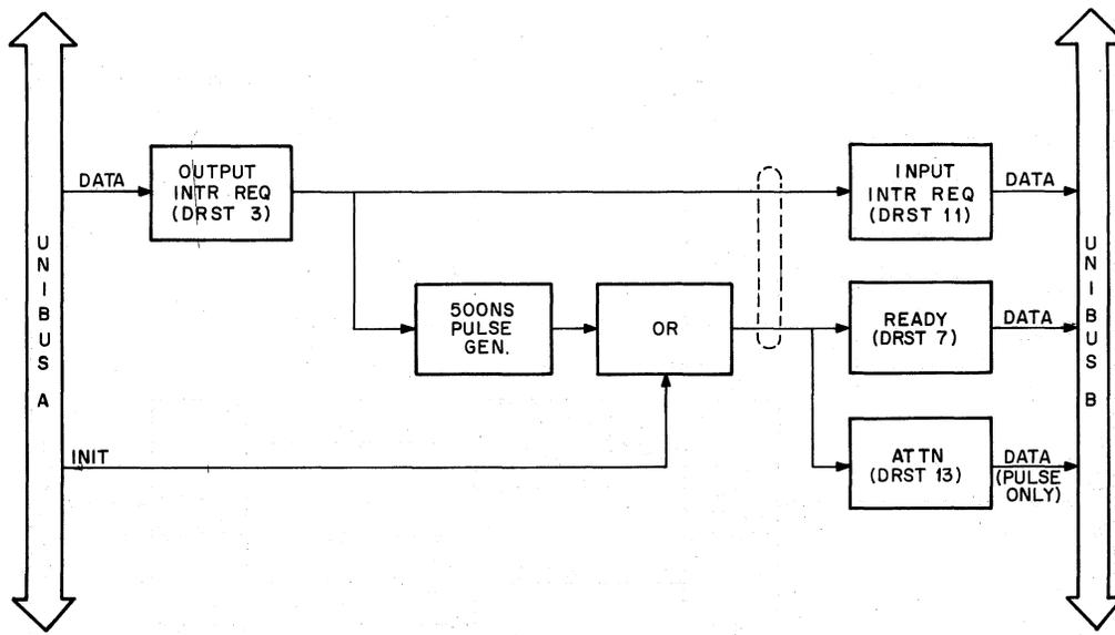
Figure C-3 Cross-Interrupt Block Diagram
