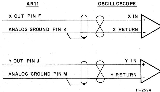
Figure 4-2 Connection to Oscilloscope with Differential Input
