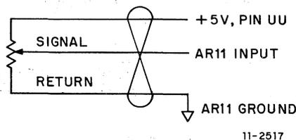
Figure 2-3 Use of +5 V Supply Output
