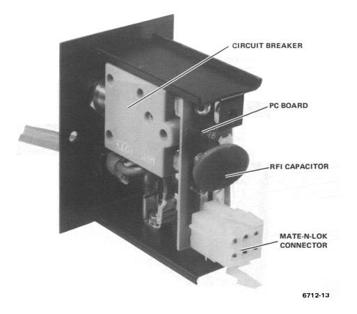
Figure 3-7 BC05T Line Set, Cover Removed
