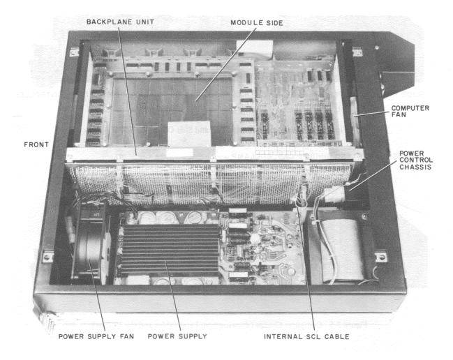
Figure 3-3 Computer Box With Top Cover Removed
