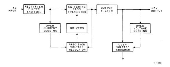
Figure 3-20 +5 V Regulator (PS2) Functional Block Diagram
