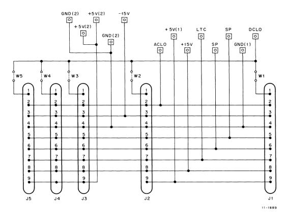
Figure 3-13 Power Distribution Board Circuit Schematic
