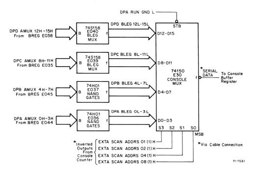
Figure 8-13 Console Multiplexer Block Diagram
