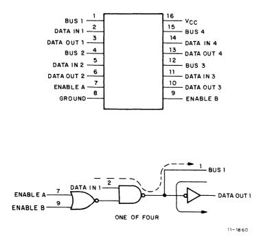
Figure 2 8838 Quad Bus Transceivers
