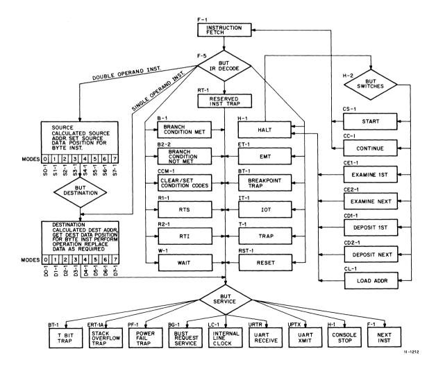
Figure 9-2 KD11-B Simplified Flow Diagram
