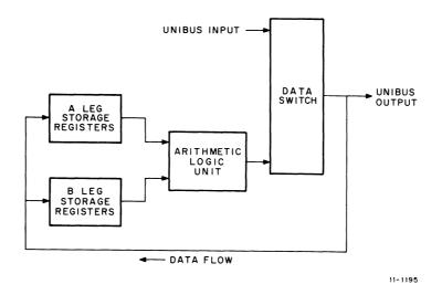
Figure 8-3 KD11-B Simplified Data Path Block Diagram
