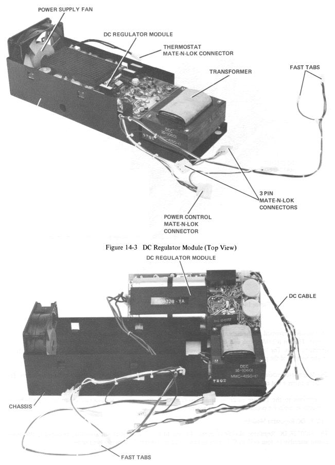
Figure 14-4 DC Regulator Module (Bottom View In Mounting Box)
