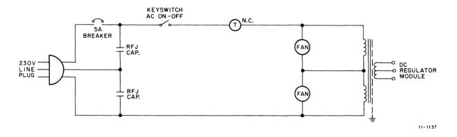
Figure 15-3 230V Connection Diagram
