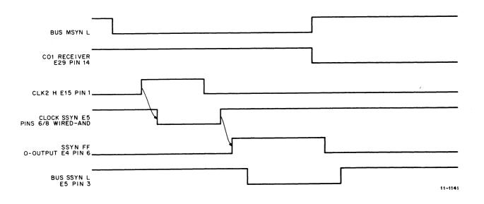
Timing Diagram for SSYN Circuit During DATO and DATOB
