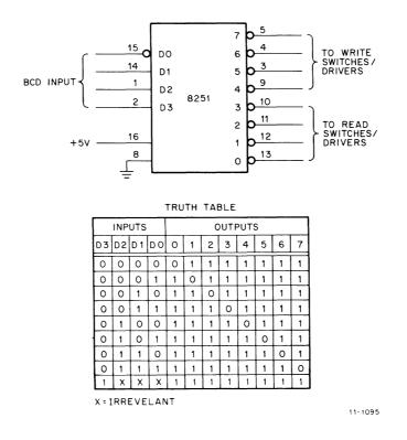
Figure 12-9 Type 8251 Decoder, Pin Designation and Truth Table
