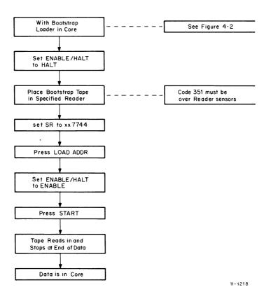
Figure 4-3 Loading Bootstrap Tapes Into Memory
