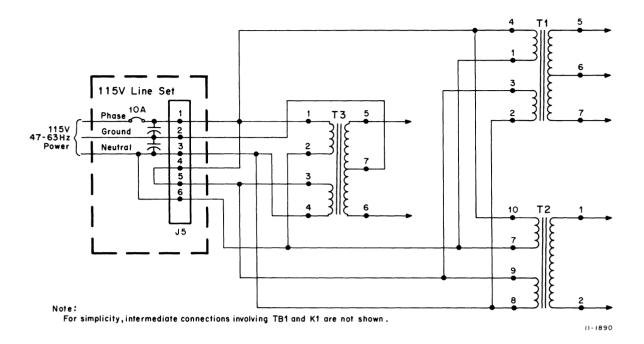
Figure 3-11 Power Application Using 115 V Line Set
