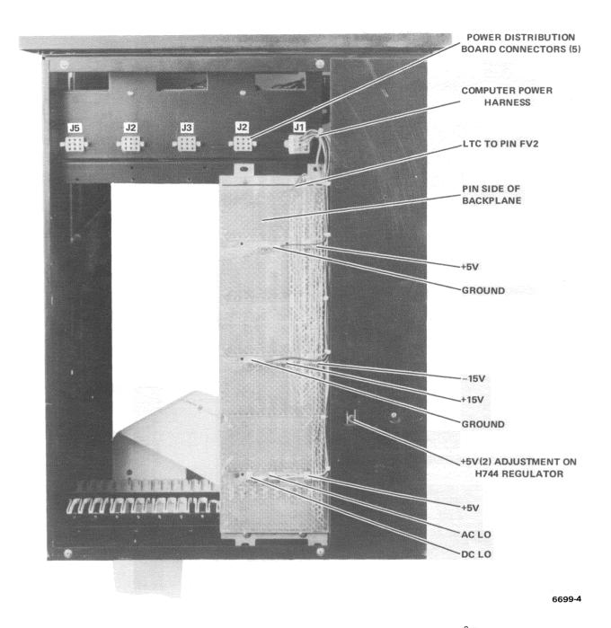
Figure 1-3 PDP-11/05 NC Computer Extended and Locked In Front Up 90° Position
