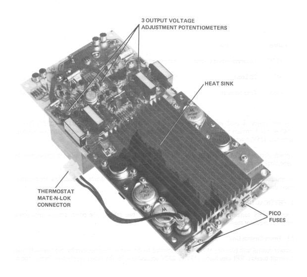
Figure 14-1 Power Chassis Assembly (with DC Regulator Module)
