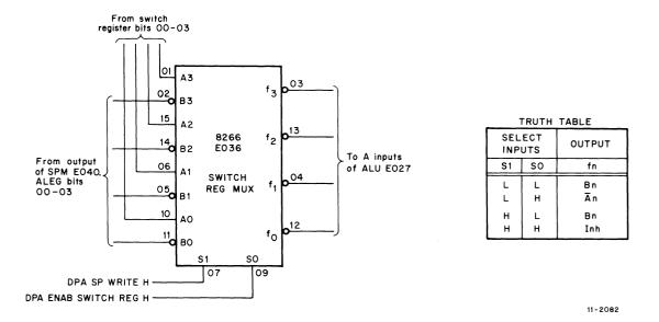
Figure 3 Typical Switch Register Multiplexer
