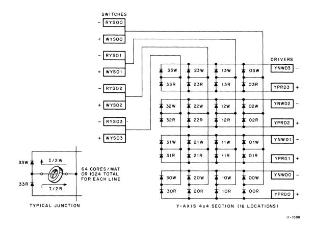
Figure 12-12 Y-Line Selection Stack Diode Matrix
