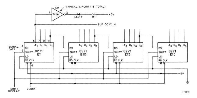
Figure 7-4 Display Buffer and Driver, Simplified Logic Diagram
