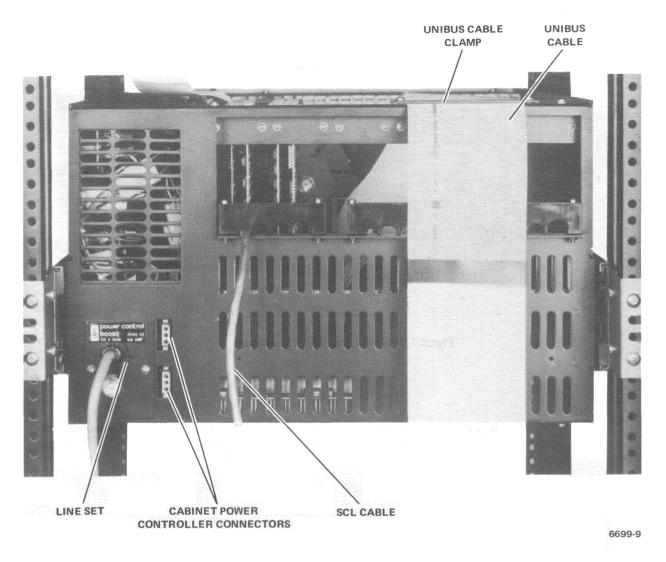
Figure 1-4 PDP-11/05 NC Computer, Rear View
