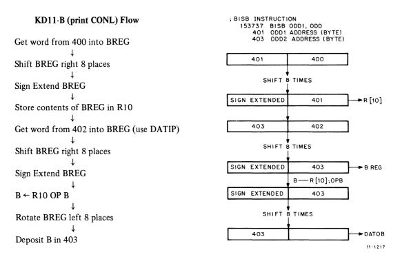
Figure 8-10 Byte Format for Shifting Instructions
