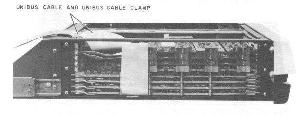
Figure 3-5 Computer Chassis (showing peripheral cables and the Unibus)
