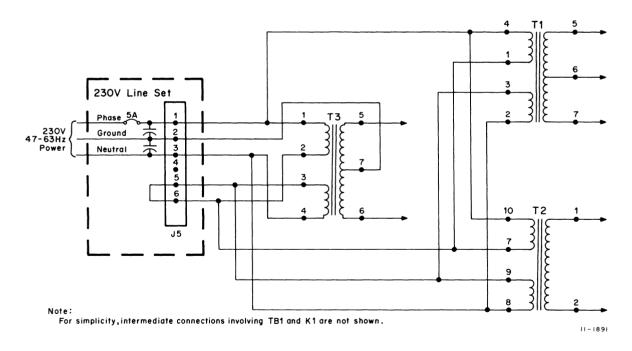
Figure 3-12 Power Application Using 230 V Line Set
