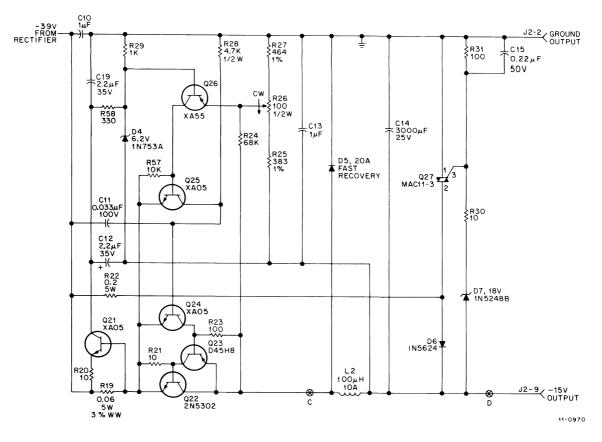
Figure 3-19 -15 V Regulator Circuit
