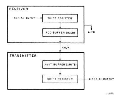
Figure 8-18 Double-Buffering Data Flow
