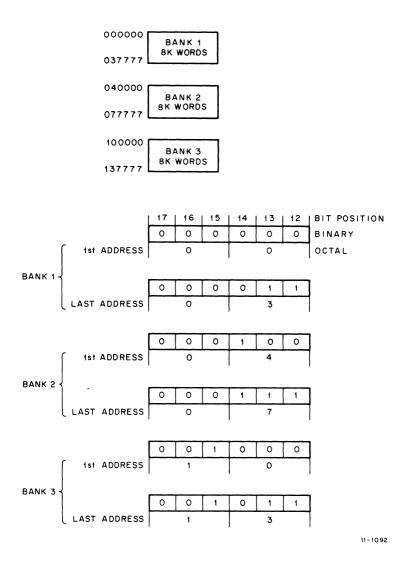
Figure 12-6 Address Assignments For Three Banks of 8K Words Each
