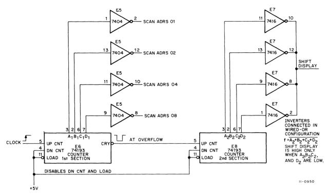
Figure 7-3 Counter, Simplified Logic Diagram
