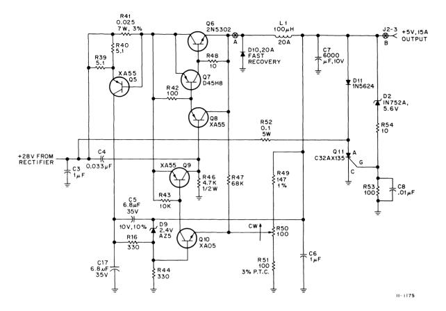
Figure 15-8 +5V Regulator Circuit
