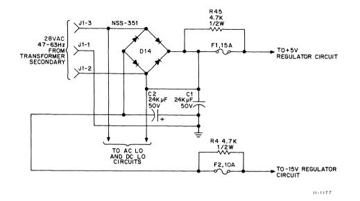
Figure 3-15 Rectifier and LTC Circuits
