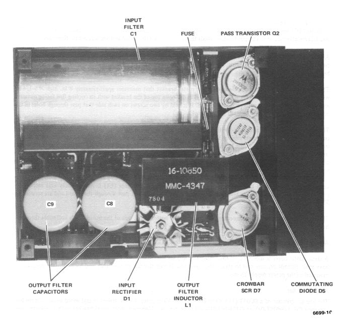
Figure 3-5 +5 V Regulator, Side View
