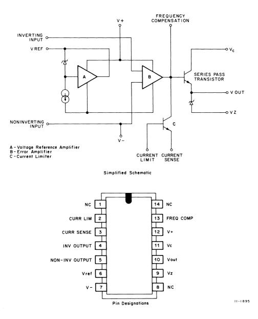
Figure 3-22 Voltage Regulator (E1) Equivalent Circuit and Package Configuration
