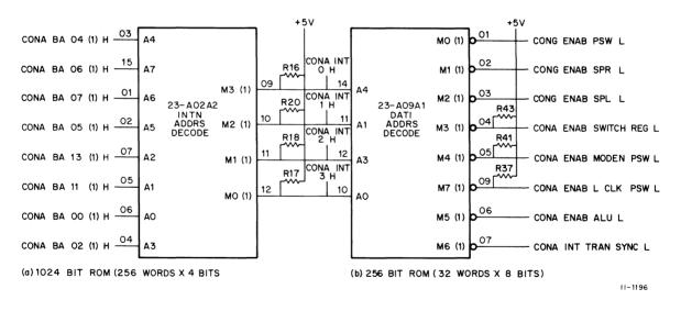
Figure 8-1 1024-Bit and 256-Bit ROMs
