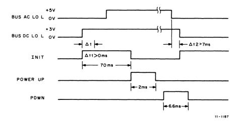
Figure 8-19 BUS AC LO and BUS DC LO Timing Diagram
