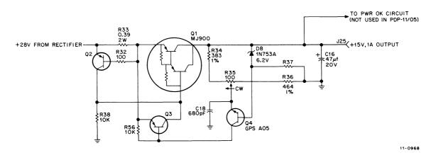
Figure 15-7 +15V Regulator Circuit
