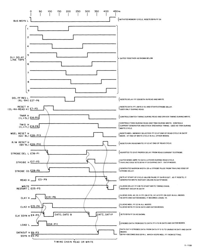
Figure 12-20 Basic Timing and Control Signal Functions
