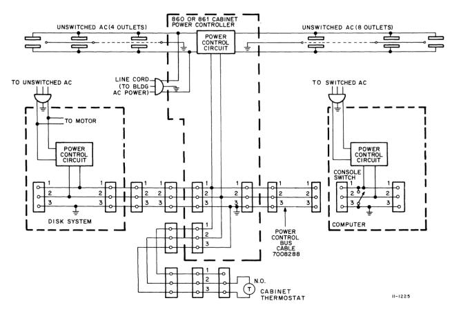
Figure 2-3 Typical Cabinet Power Control System Wiring Diagram
