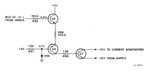
Figure 12-19 DC LO Circuit, Schematic Diagram
