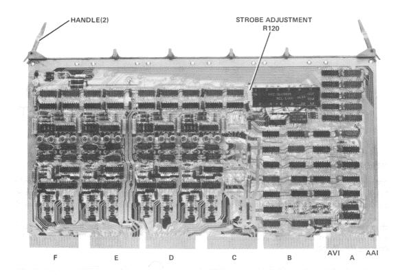
Figure 11-1 Component Side of G110 Control Module
