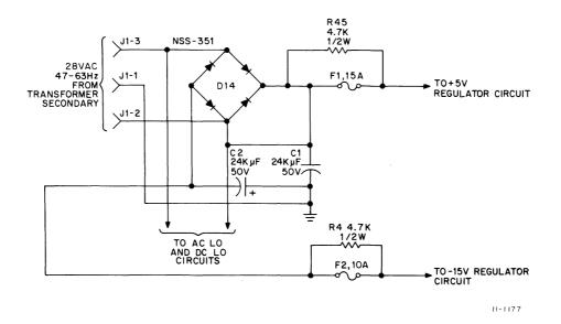
Figure 15-5 Rectifier and LTC L Circuits
