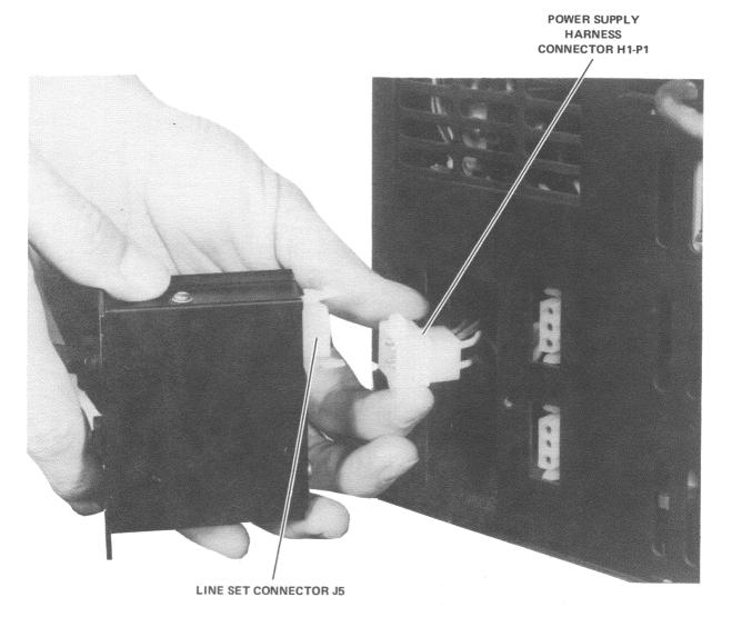
Figure 3-25 Disconnecting Line Set From Power Supply
