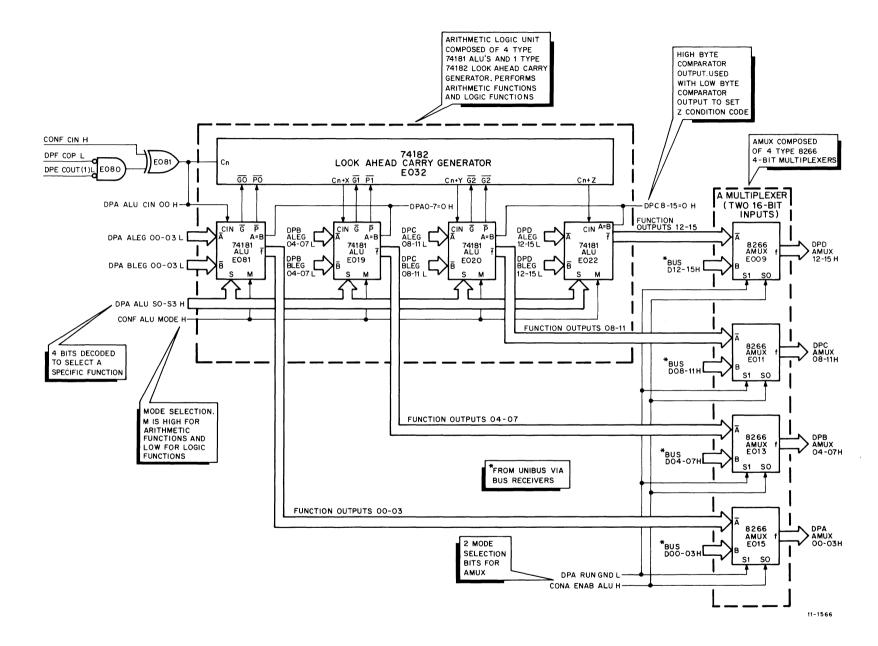
Figure 8-7 Arithmetic Logic Unit Block Diagram
