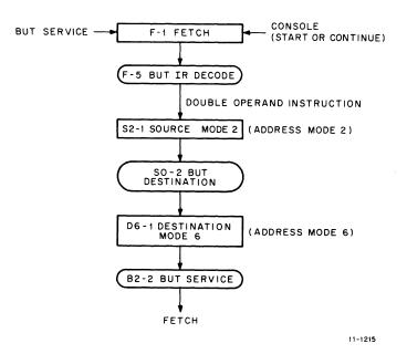
Figure 9-4 CMP #15, CHAR (022767), Simplified Flow Diagram
