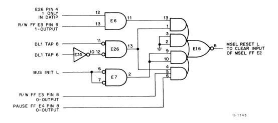
Figure 12-22 Generation of MSEL RESET L
