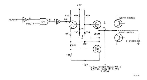
Figure 12-18 Stack Discharge Circuit
