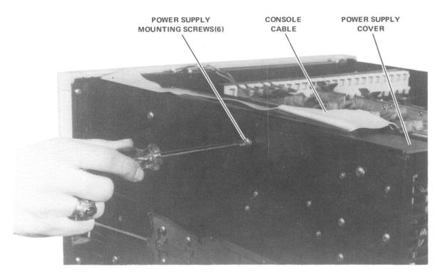
Figure 3-26 Removing Power Supply Mounting Screws
