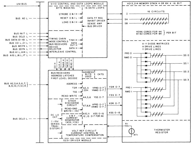
Figure 11-4 MM11-K, L Memory Block Diagram
