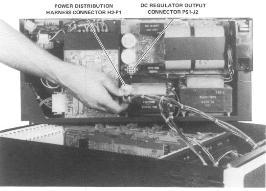
Figure 3-28 Lifting Power Supply From Mounting Box
