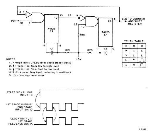
Figure 7-2 Console Clock, Schematic and Timing Diagram
