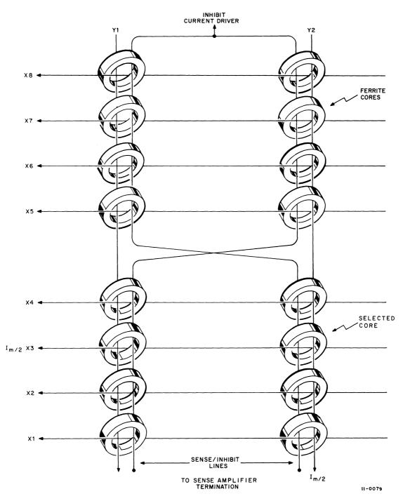
Figure 12-1 Three-Wire Memory Configuration
