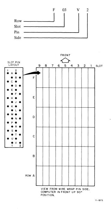
Figure 1-7 Computer Backplane Connector and Pin Designations
