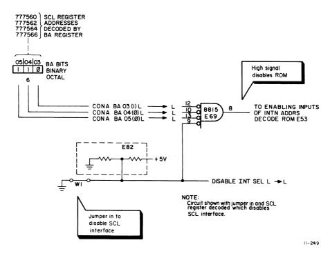
Figure 2 SCL Interface Disabling Circuit
