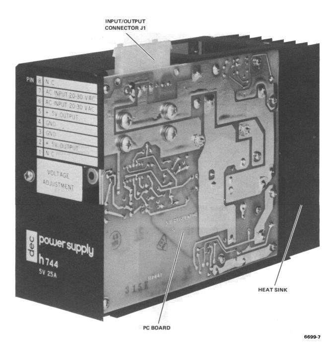
Figure 3-6 +5 V Regulator, 3/4 Bottom View
