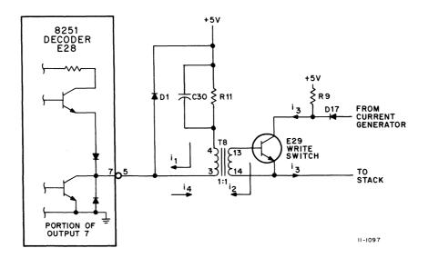
Figure 12-11 Switch or Driver Base Drive Circuit
