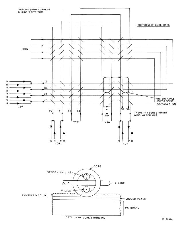
Figure 12-3 Three-Wire 3D Memory, Four Mats Shown for a 16-Word 4-Bit Memory
