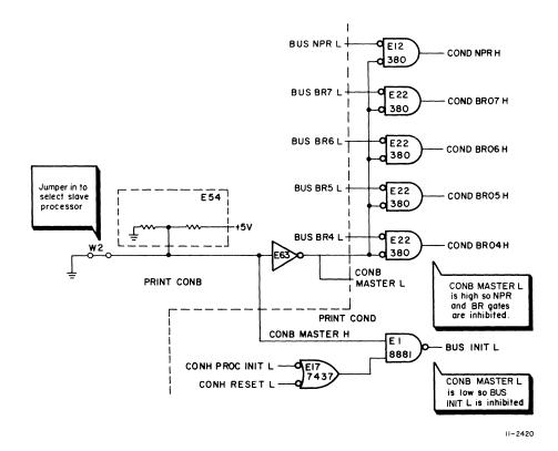
Figure 3 Slave Processor Selection Circuit
