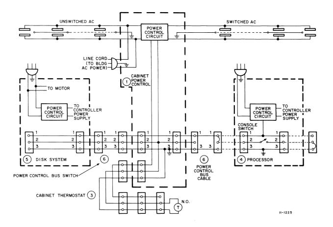
Figure 3-8 Typical Cabinet Power Control System Wiring Diagram
