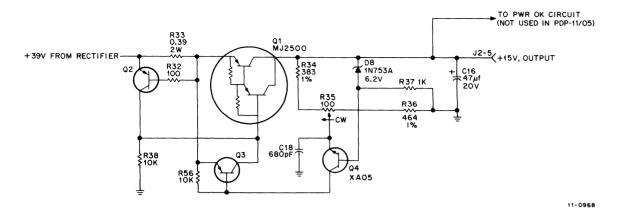
Figure 3-17 +15 V Regulator Circuit
