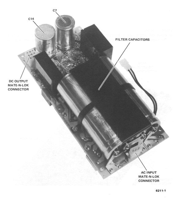
Figure 3-4 DC Regulator, Bottom View
