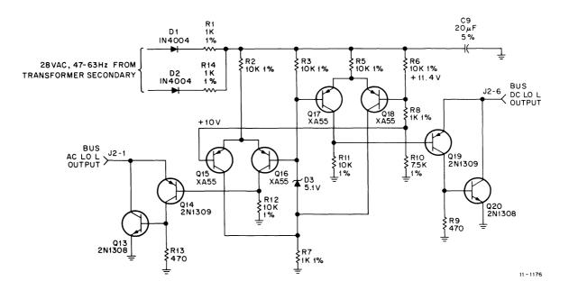
Figure 3-16 BUS AC LO and BUS DC LO Circuits
