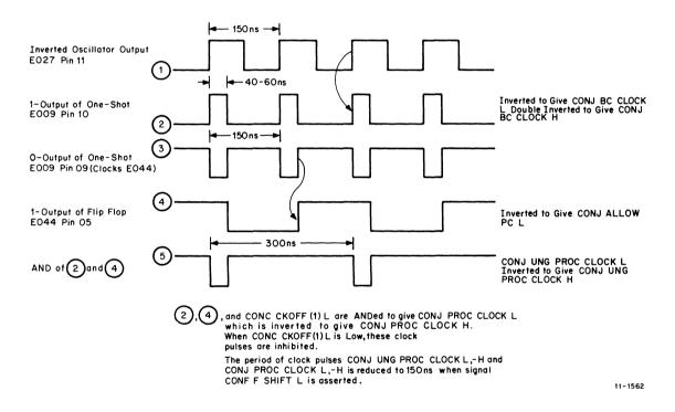
Figure 8-14 Processor Clock Timing Diagram
