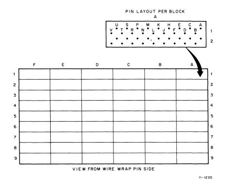
Figure 1-3 Computer Backplane Connector and Pin Designations
