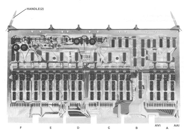
Figure 11-2 Component Side of G231 Driver Module
