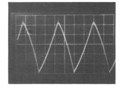
f) Point D, 5A load, 50 μs/div, and 50 mV/div.
