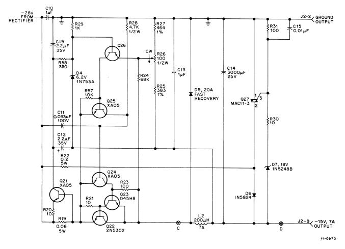
Figure 15-9 -15V Regulator Circuit
