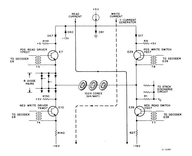
Figure 12-13 Typical Y-Line Read/Write Switches and Drivers
