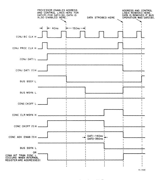
Figure 8-15 DATI and DATO Timing
