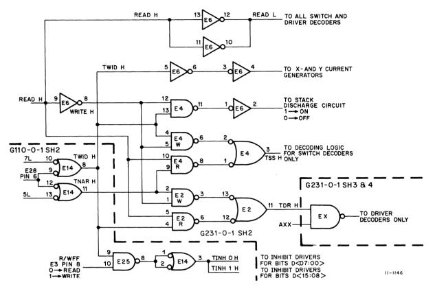
Figure 12-21 TWID H and TNAR H Control Logic
