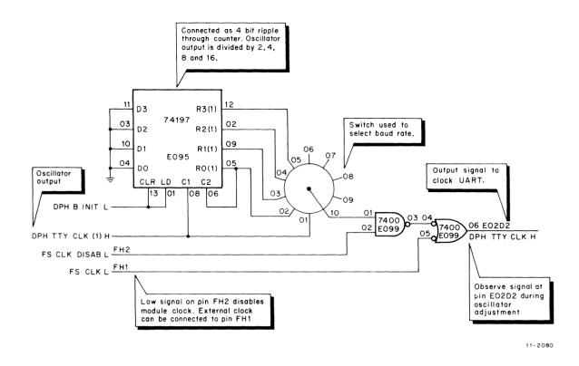
Figure 6 Baud Selection Logic
