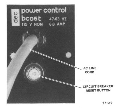
Figure 3-8 BC05T Line Set, Rear View
