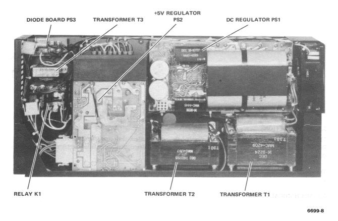
Figure 3-1 Power Supply Side View
