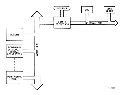
Figure 5-1 KD11-B With Interconnections to Memory and Peripherals
