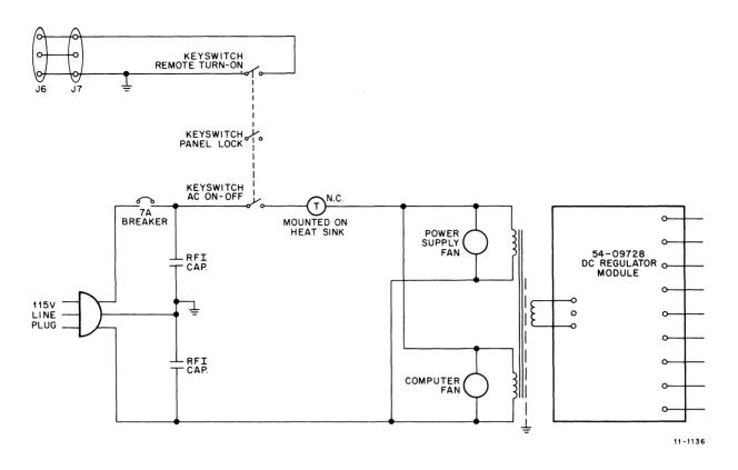
Figure 15-2 115V Connections – Simplified Schematic Diagram
