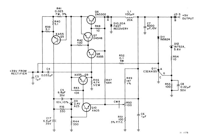
Figure 3-18 +5 V Regulator Circuit
