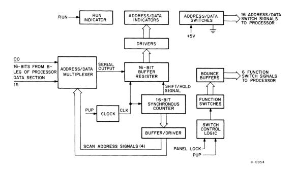
Figure 7-1 Console Functional Block Diagram
