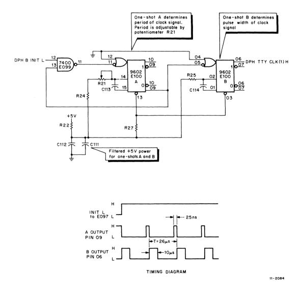
Figure 5 SCL Oscillator Schematic and Timing Diagram
