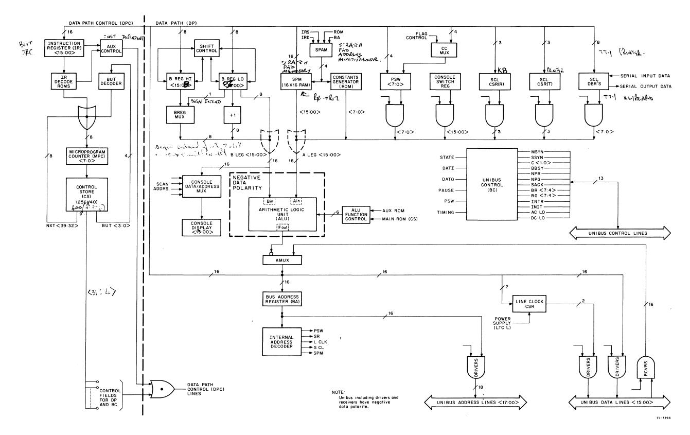
Figure 8-4 KD11-B Detailed Block Diagram
