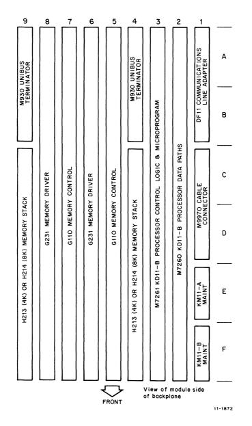
Figure 1-9 Module Utilization Diagram
