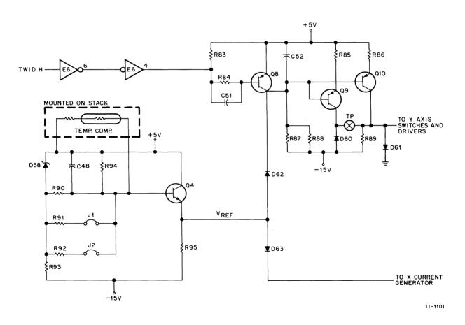
Figure 12-15 Y-Current Generator and Reference Voltage Supply
