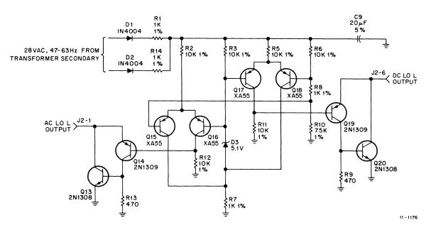
Figure 15-6 BUS AC LO and BUS DC LO Circuits
