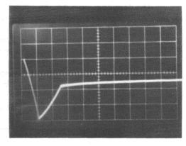
e) Point D, No load, 50 μs/div, and 50 mV/div.
