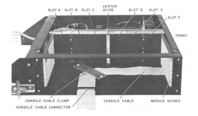
Figure 3-6 Mounting Box Without Modules
