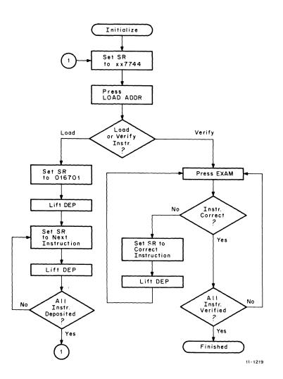
Figure 4-2 Loading and Verifying the Bootstrap Loader
