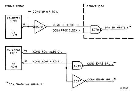
Figure 9-7 Generation of SPM Enabling Signals
