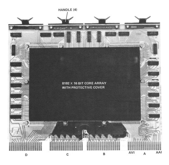
Figure 11-3 Component Side of 8K H214 Stack Module
