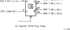
Figure 5-4 Typical Small Scale Integrated Circuit Representations
