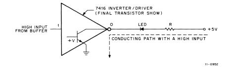
Figure 7-5 LED Driver Circuit
