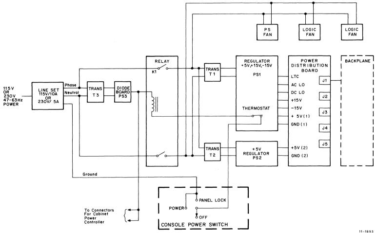
Figure 3-9 Power System Functional Block Diagram
