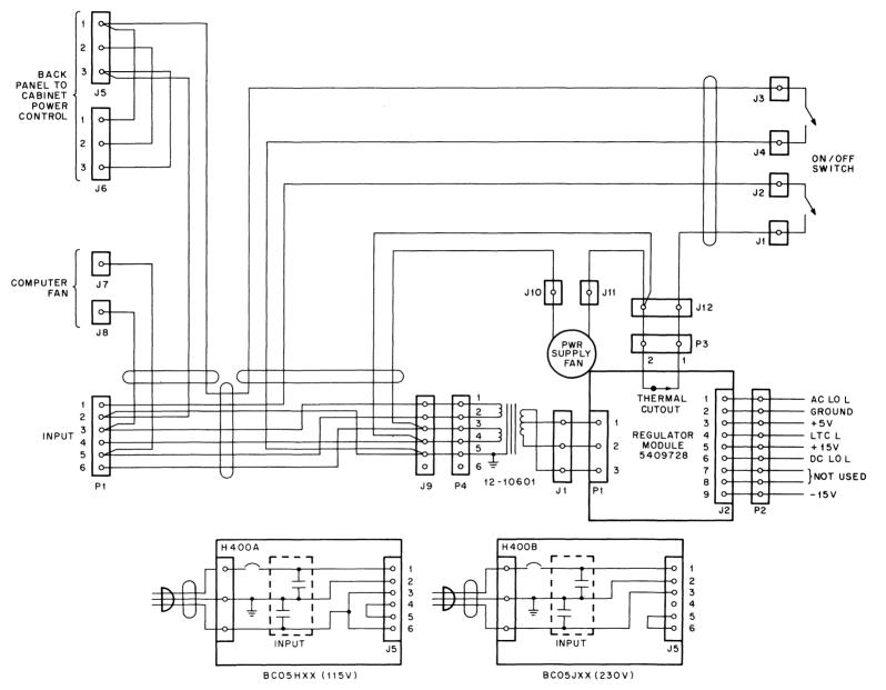
Figure 15-1 Detailed AC Interconnection Diagram
