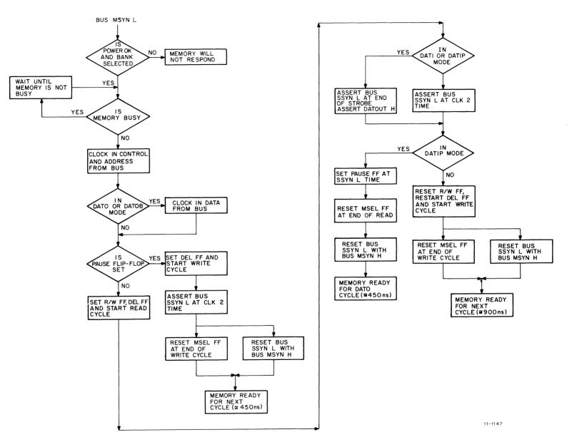
Figure 12-26 Flow Chart For Memory Operation
