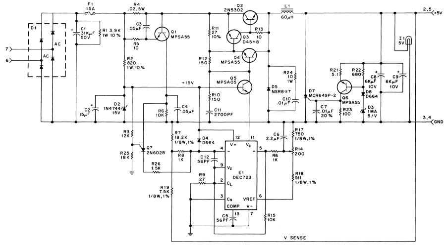
Figure 3-21 +5 V Regulator (PS2) Circuit Schematic
