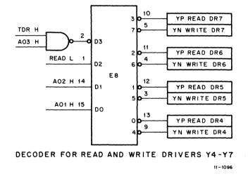
Figure 12-10 Decoding of Read/Write Switches and Drivers Y4-Y7
