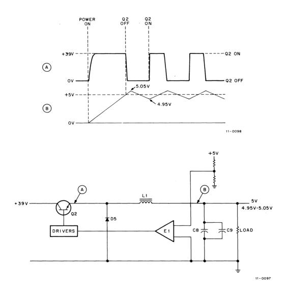
Figure 3-23 Simplified 5 V Switching Regulator Schematic and Waveforms
