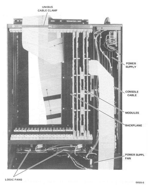
Figure 1-2 PDP-11/05 NC Computer Extended and Locked In Front Down 90° Position
