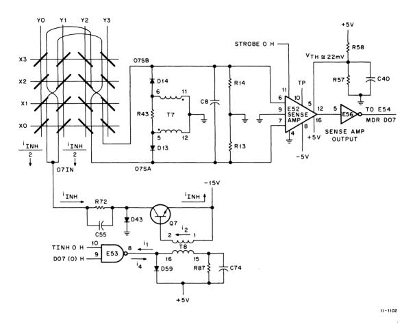
Figure 12-16 Sense Amplifier and Inhibit Driver
