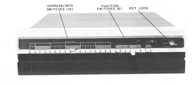
Figure 4-1 Console Illustrating Switch Movements
