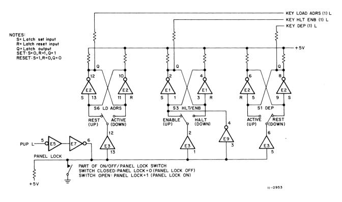
Figure 7-6 Control Switches and Bounce Buffers, Logic Diagram
