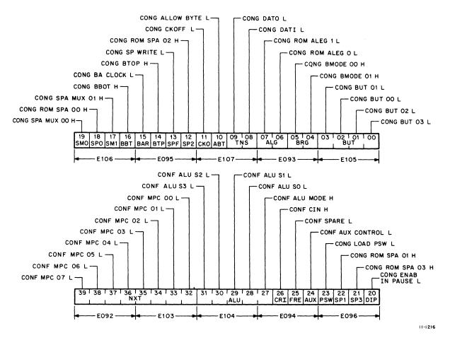
Figure 9-1 Control Store Word Bit and Field Format
