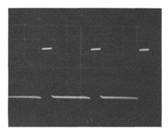
f) Point B, 20A load, μs/div, and 50 mV/div.
