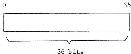
This function allows the programmer to 'lift' a byte of any length from any position in a source word. The value of the result of the function is the value of the destination word with the specified byte from the source word inserted in the required position. The values of all the arguments are unchanged.
