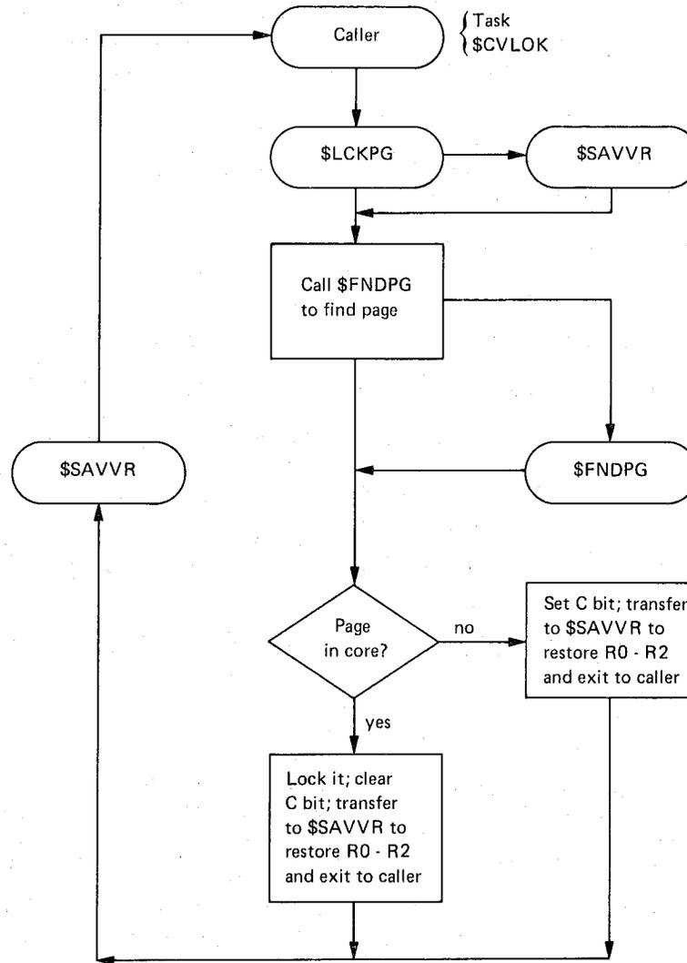
Figure 8-14 General Block Diagram of the \$LCKPG Routine
