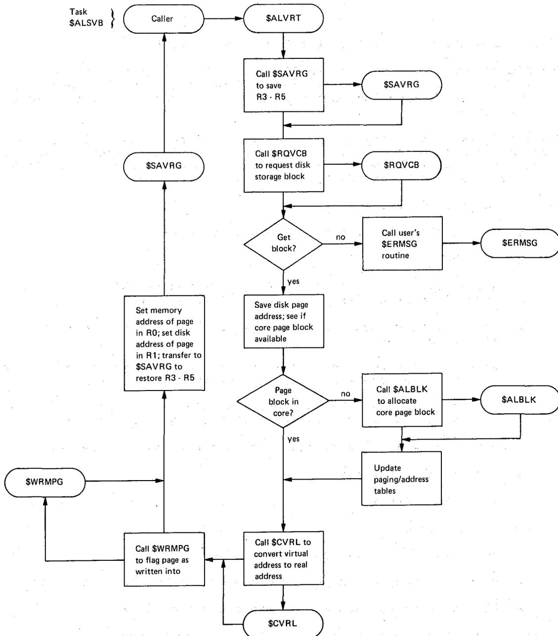
Figure 8-6 General Block Diagram of the \$ALVRT Routine
