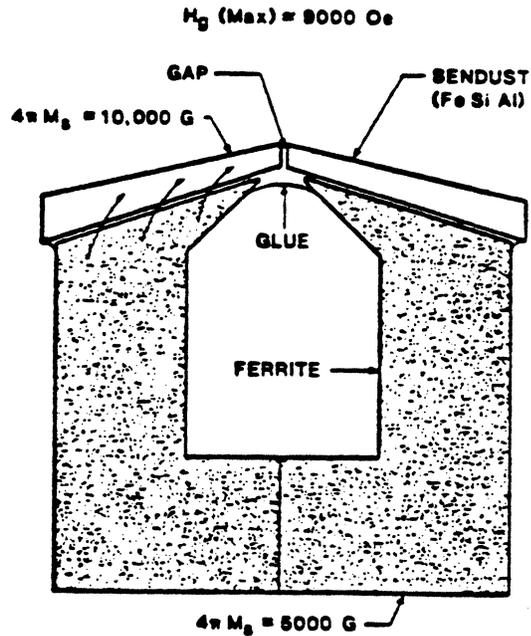
FIG. 5 SENDUST TIPPED BENCHMARK HEAD CROSS SECTION
