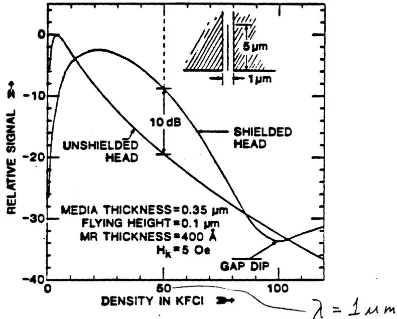
FIG. 35 Comparison of shielded and unshielded MR head response curves.
