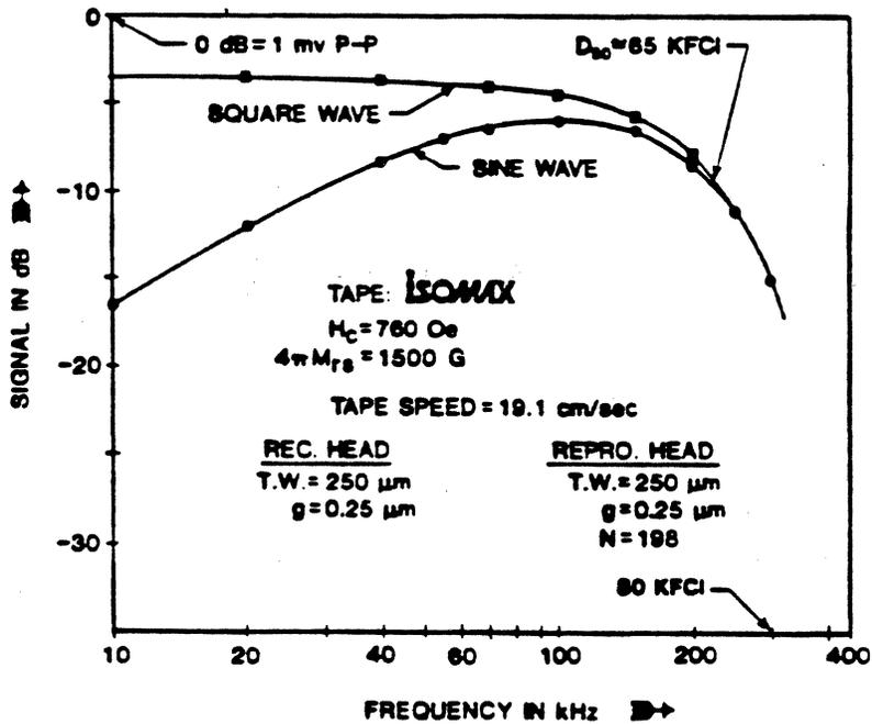
FIG. 20 COMPARISON OF SINEWAVE AND SQUAREWAVE RECORDING. RECORD AND REPRODUCE HEADS ARE SENDUST TIPPED.
