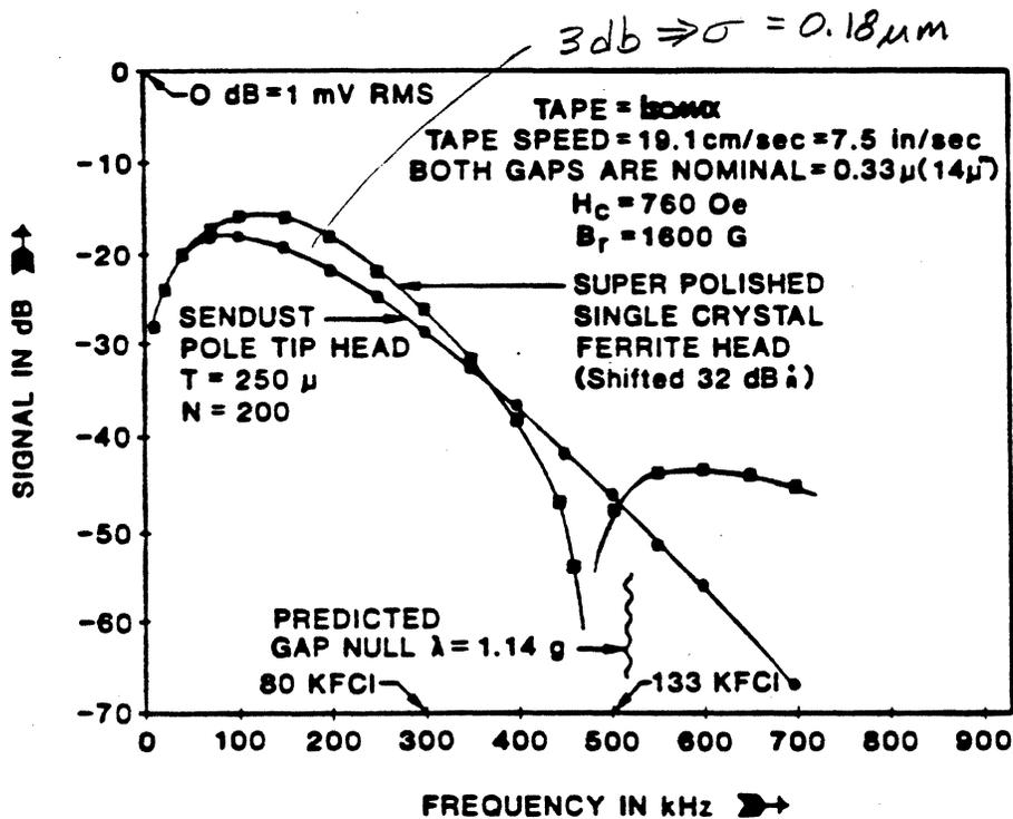
The ferrite head curve was shifted up to compensate for differences in track width, turns, and core efficiency. The ferrite head shows the expected gap null because its gap surface was "superpolished" using a colloidal  $\text{SiO}_2$  lap,<sup>19</sup> which results in a surface finish as shown in Fig. 25. Nearly all of the artifacts visible are dust in the microscope optical path.
