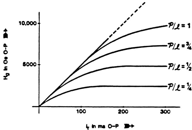
FIG.12  $H_g$  versus  $i_r$  for single turn record head with  $g = 0.25 \mu\text{m}$  and various  $P/l$  values.
