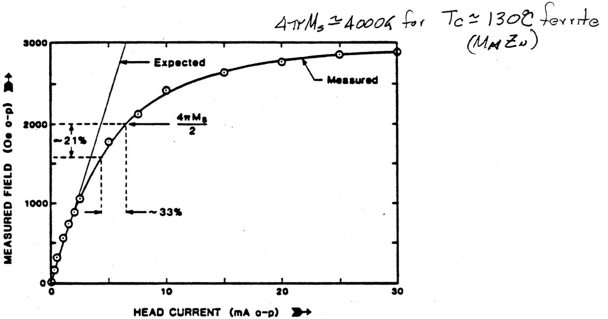
FIG. 7 FIELD VERSUS CURRENT FOR A 5  $\mu\text{m}$  GAP FERRITE AUDIO CASSETTE HEAD.
