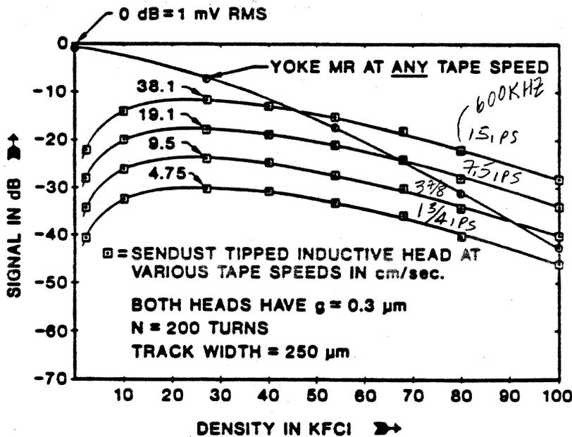
FIG. 37 YOKE MR & INDUCTIVE HEADS COMPARED
