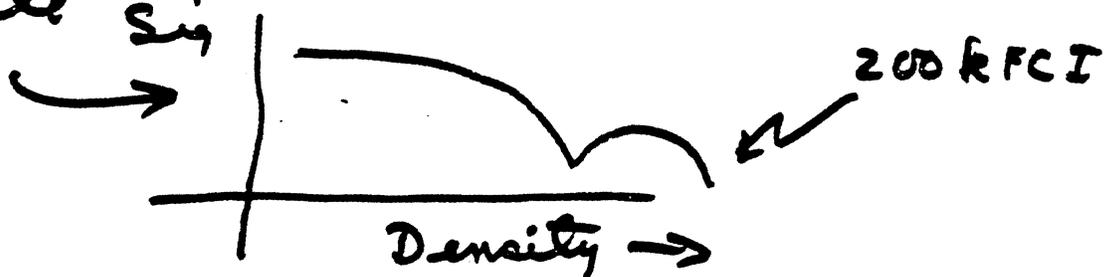
"proper"  $\equiv$  small gap heads and record current set to peak very short  $\lambda \leq 0.75 \mu\text{m}$  signal.
