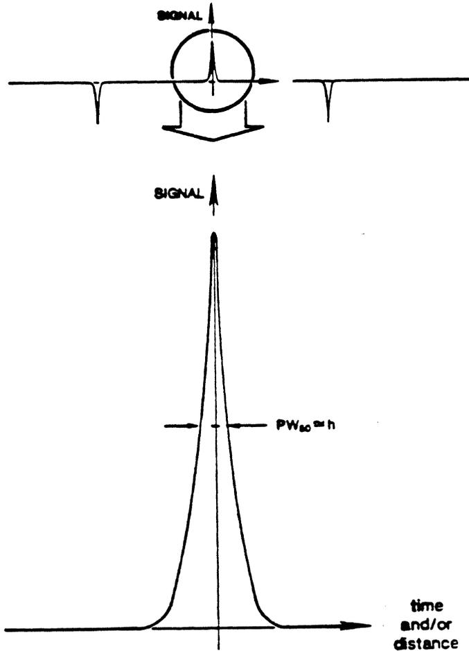
The full width at half maximum  $PW(50) = h$  for small head-medium separation. As a result, the signal spectrum covers a very large range as shown by Fig. 34, where spectra for several elements are shown.<sup>25</sup>
