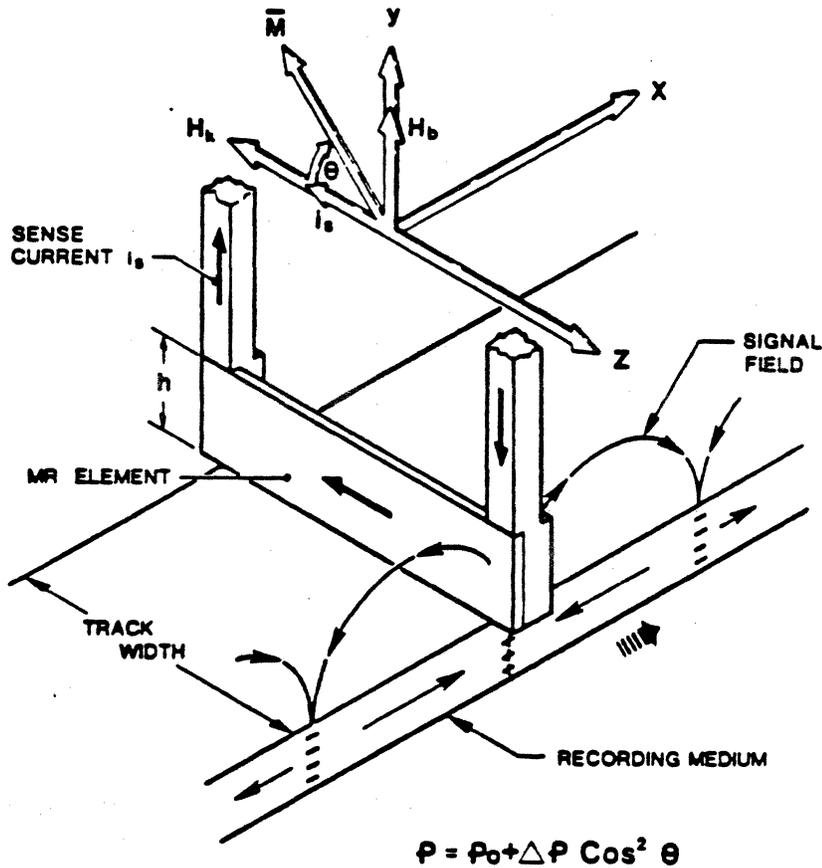
The height must be more than - 4-5 $\mu$ m or so, because of wear considerations. As a result, it detects approaching digital transitions before they are under the sensor. The isolated pulse shape is as shown in Fig. 33
