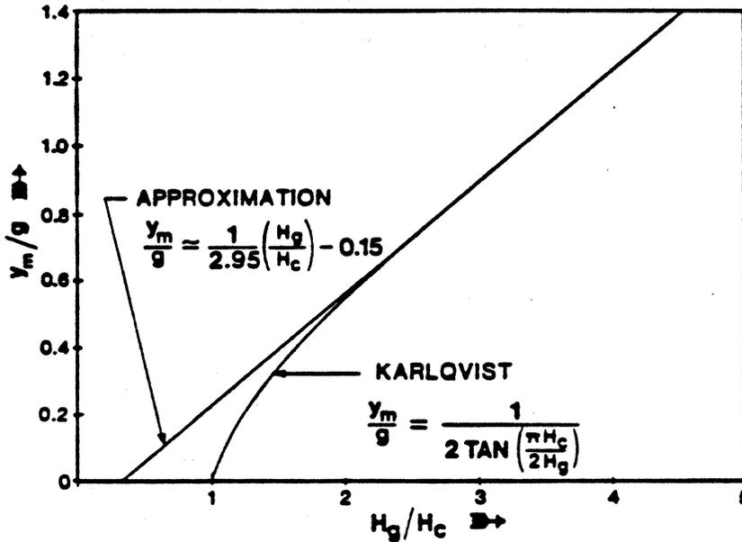
FIG. 17 PLOT OF  $\frac{Y_m}{g}$  VERSUS  $\frac{H_c}{H_g}$
