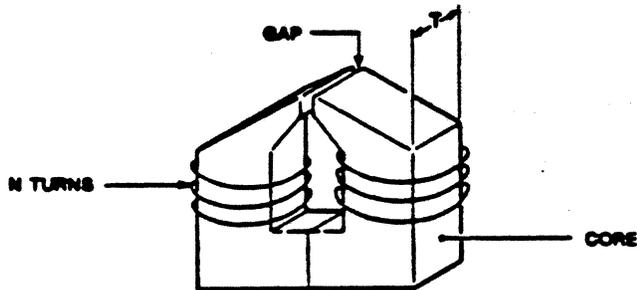
FIG. 2b CROSECTION OF RECORD GAP & HEAD FIELD CONTOURS
