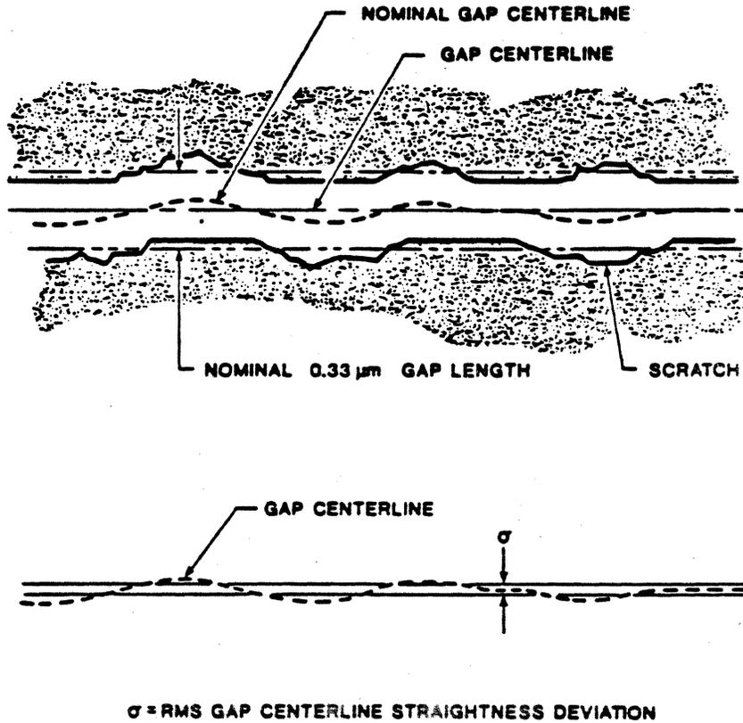
The gap length variation shown in Fig. 23 washes out the gap null. Figure 24 shows a 250 $\mu$ m track width Sendust pole tip reproduce head spectrum, which is linear where the gap null should be. Also shown in Fig. 24 is the reproduce spectrum of a 36 $\mu$ m track width single-crystal MnZn video head with the same gap.
