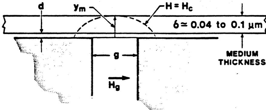
FIG. 15 RECORD CONTOUR FOR THIN FILM MEDIA.
