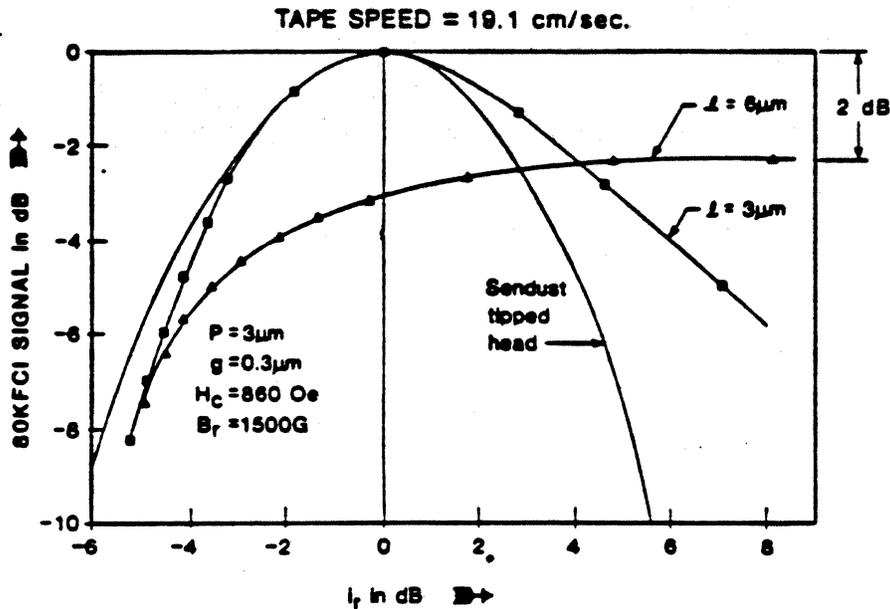
FIG. 13 80 KFCI or  $\lambda = 0.635\mu\text{m}$  signal level versus record current for a single turn head.
