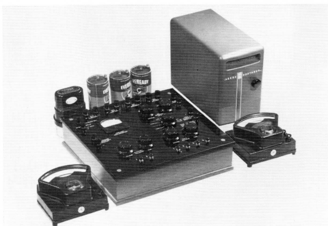
Slide 10—Weston Standard Cell Comparator with associated equipment.
