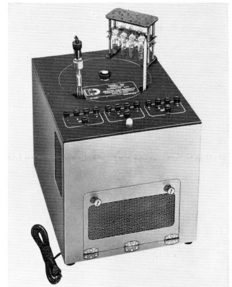
Slide 8—Weston Model 66 Standard Cell Temperature Bath for saturated standard cells.
