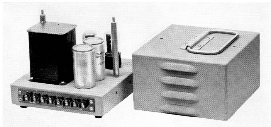
Figure 5—Weston Model 1446 Inductronic Control Unit—cover removed.
