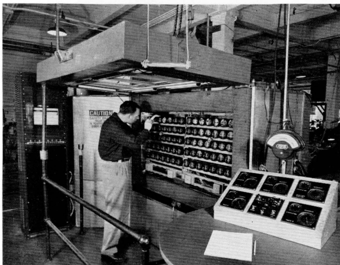
Figure 5—Extreme Temperature Test Cabinet. Temperature range: -75 C to +85 C (-103 F to +185 F).
