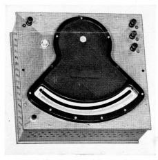
Figure 5-The Weston Model 326 Voltmeter.
