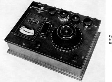
Figure 4—Leeds and Northrup Model 7 Brooks Deflection Potentiometer.
