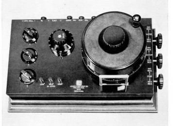
are made so that even values of potential can be read directly. Figure 3 shows a Leeds and Northrup Type K-2 precision potentiometer. indicating instrument although it has greater precision. Fundamentally, however, it is not as flexible as the null-type potentiometers,
