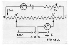
Figure 2—Diagram of a simplified potentiometer circuit.
