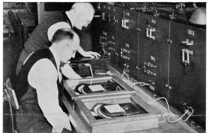
Courtesy The Detroit-Edison Co. Alternating Current Standardizing Table. Note the heavy, well-insulated supports used to minimize leakage currents and vibration.
