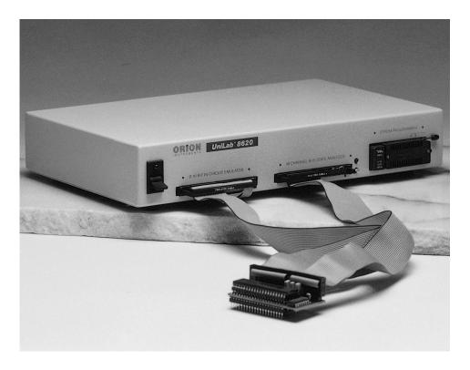
The 8620 also features a real-time Program Performance Analyzer. The PPA can track up to 15 separate areas for program activity and update the display while the target is running. A time histogram display allows you to analyze the varying amounts of time your program spends in a particular sub-routine or function.
