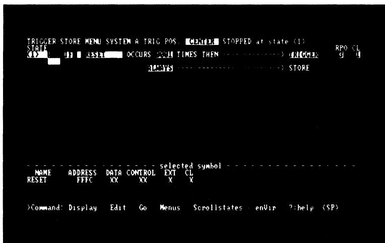
■ Figure 4-4. Trigger on Reset at power up.
