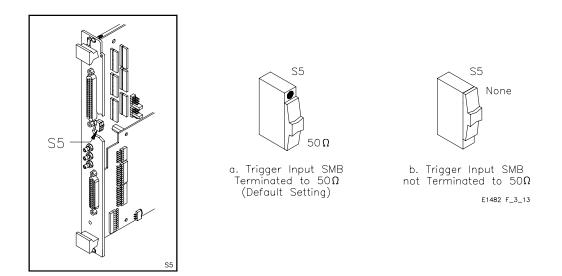
Figure 3-13. Trigger Input Termination Option Settings.
