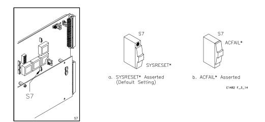
Figure 3-14. Pushbutton System Reset Settings.
