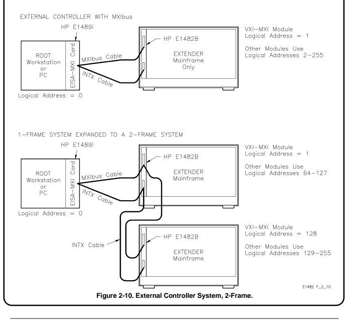
Configuring/Installing the VXI-MXI Module 31
