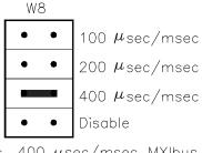
c. 400  $\mu$ sec/msec MXIbus System Controller Timeout
