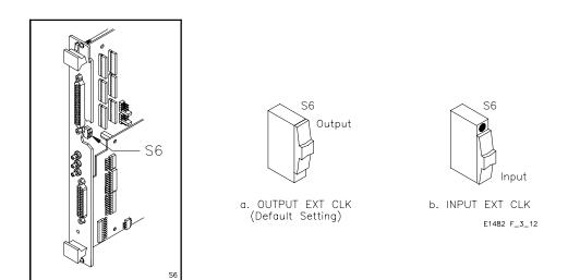
Figure 3-12. EXT CLK SMB Input/Output Setting.
