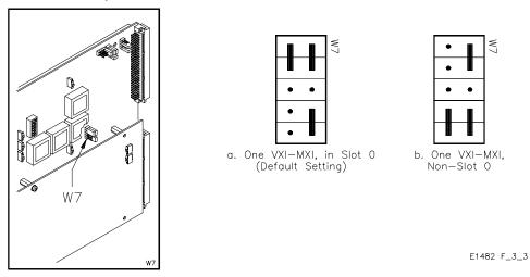
Figure 3-3. VMEbus Timeout; One VXI-MXI in Mainframe.
