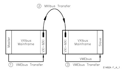
Figure 4-1. Master to Slave VMEbus/MXIbusTransfers.
