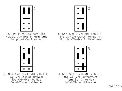
Figure 3-4. VMEbus Timeout; Multiple VXI-MXIs.
