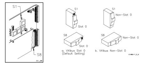
Figure 2-6. VXIbus Slot 0 Selection
