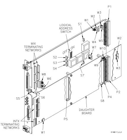
Figure 2-2. VXI-MXI Parts Locator Diagram.
