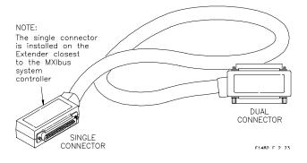
Figure 2-23. MXIbus Cable Configuration.
