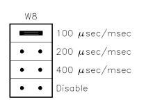
a. 100  $\mu$ sec/msec MXIbus System Controller Timeout
