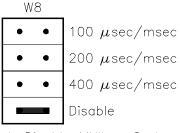
d. Disable MXIbus System Controller Timeout Generation (Default setting)
