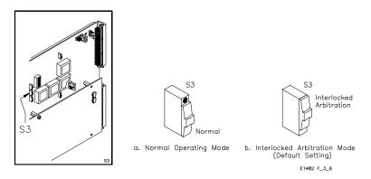
Figure 3-6. Interlocked Arbitration Mode Selection.
