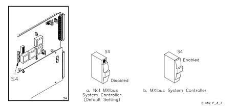
Figure 3-7. MXIbus System Controller Selection.
