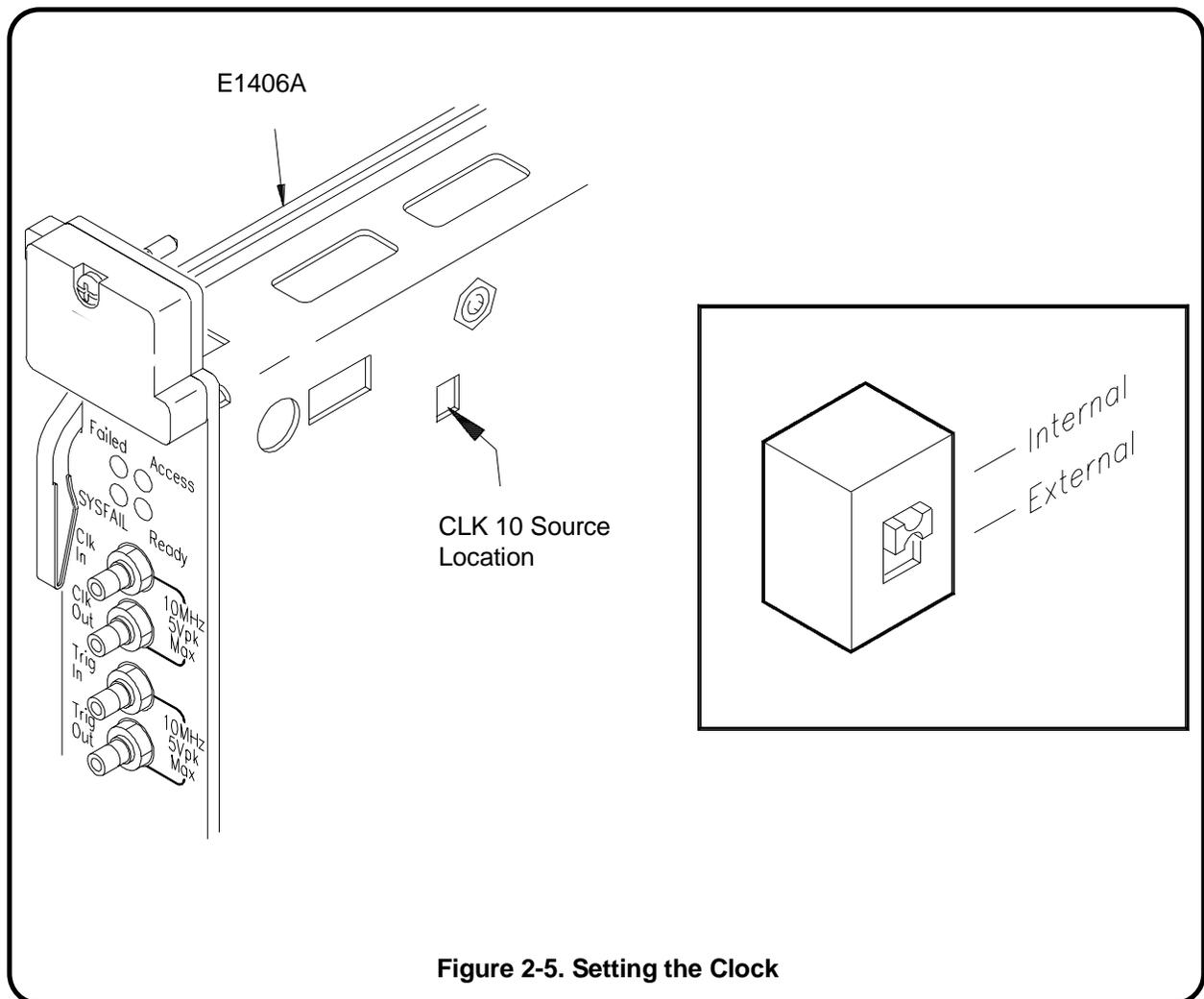
The clock is distributed to every slot along the VXIbus backplane. Disabling the slot 0 and (VME) System Controller functions removes the internal clock or external clock from the VXIbus backplane. However, the clock from either source is still present at the 'Clk Out' SMB connector.
