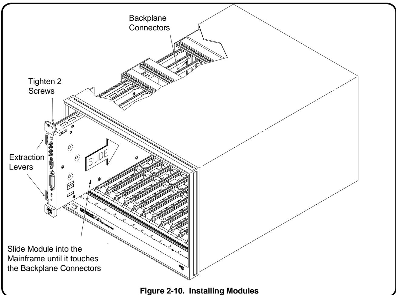
Figure 2-10. Installing Modules
