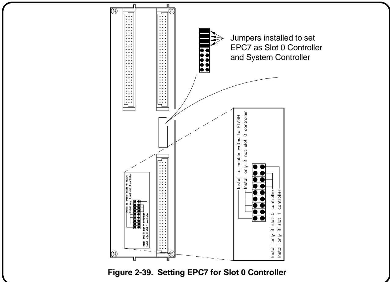
Slot 0 functionality is used during operation for the following purposes:
