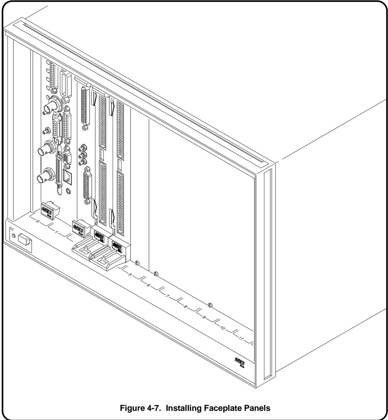
**Figure 4-7. Installing Faceplate Panels**
