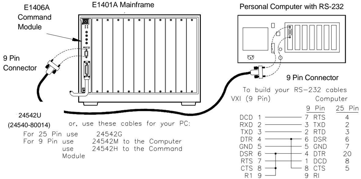
**Figure 2-10. Connecting a PC to the Command Module**
