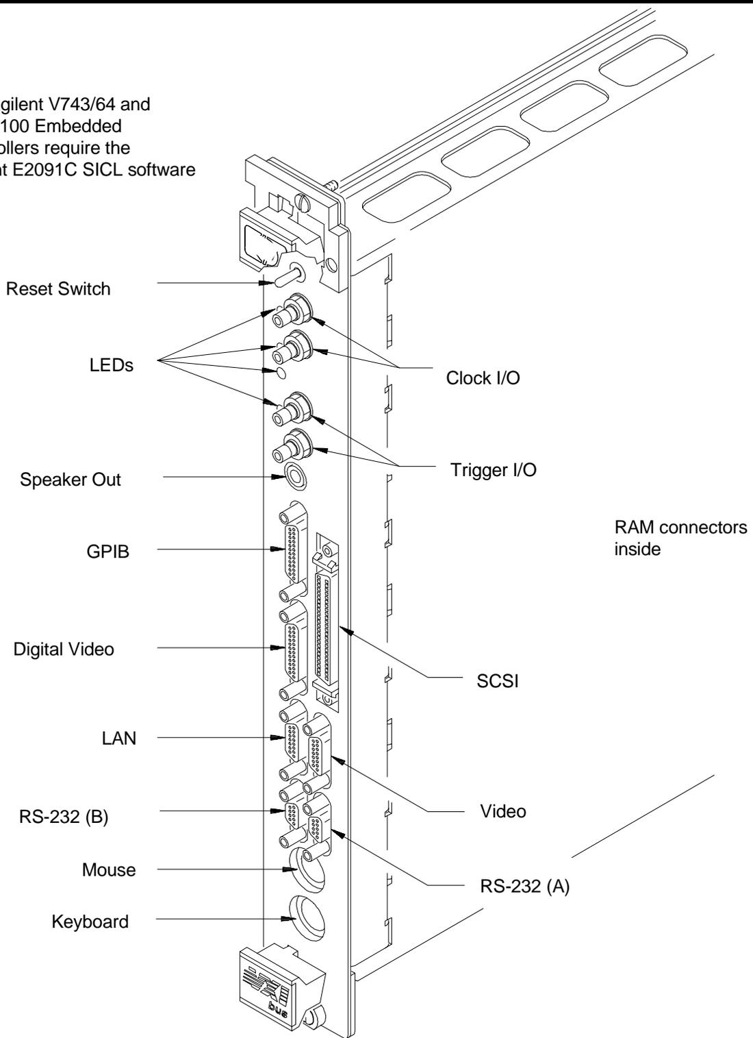
Figure 2-31. The V743 Embedded Controller
