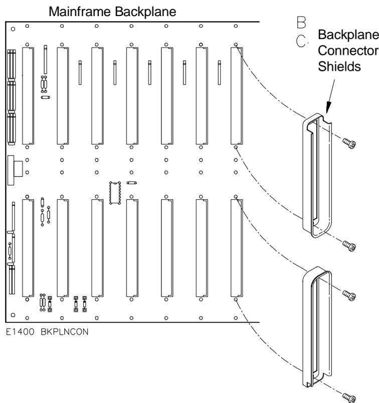
**Figure 4-6. Installing the Backplane Connector Shields**
