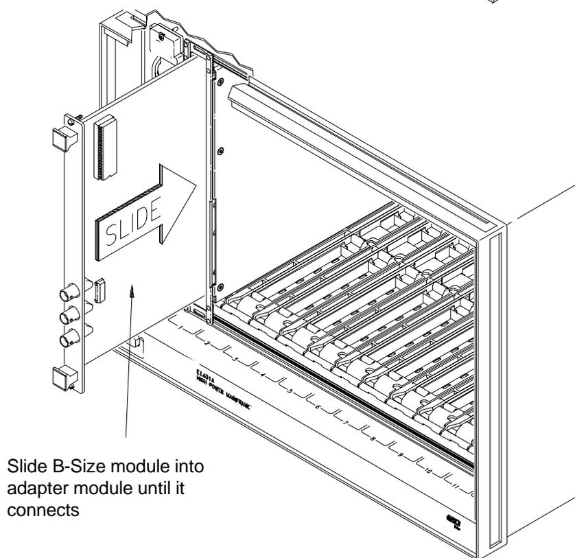
**Figure 4-2. Installing B-Size Module**
