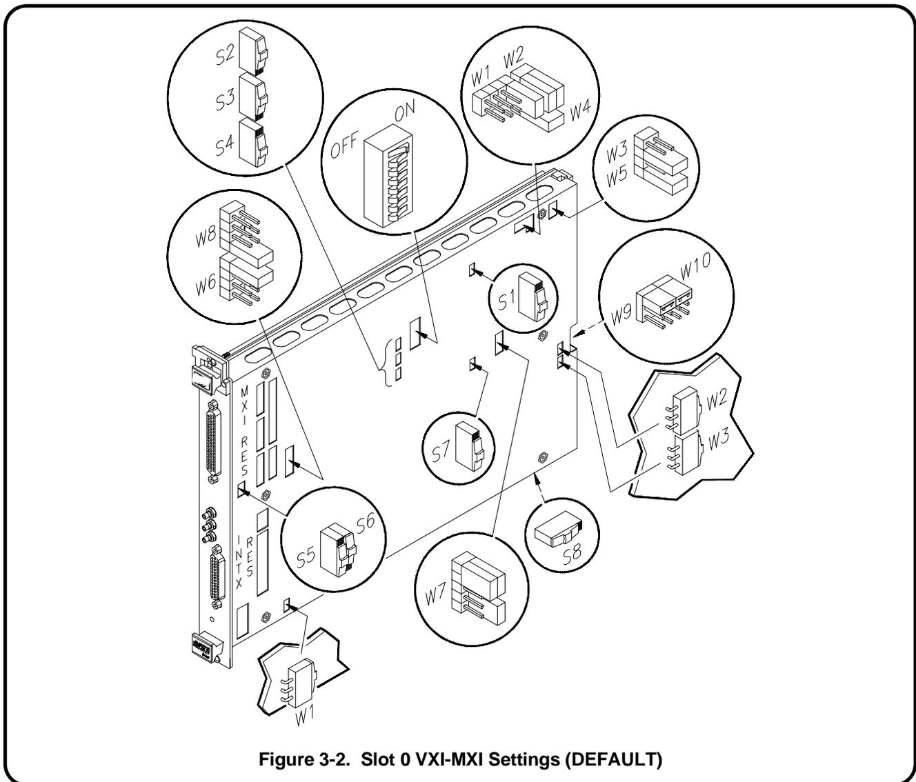
Figure 3-2. Slot 0 VXI-MXI Settings (DEFAULT)
