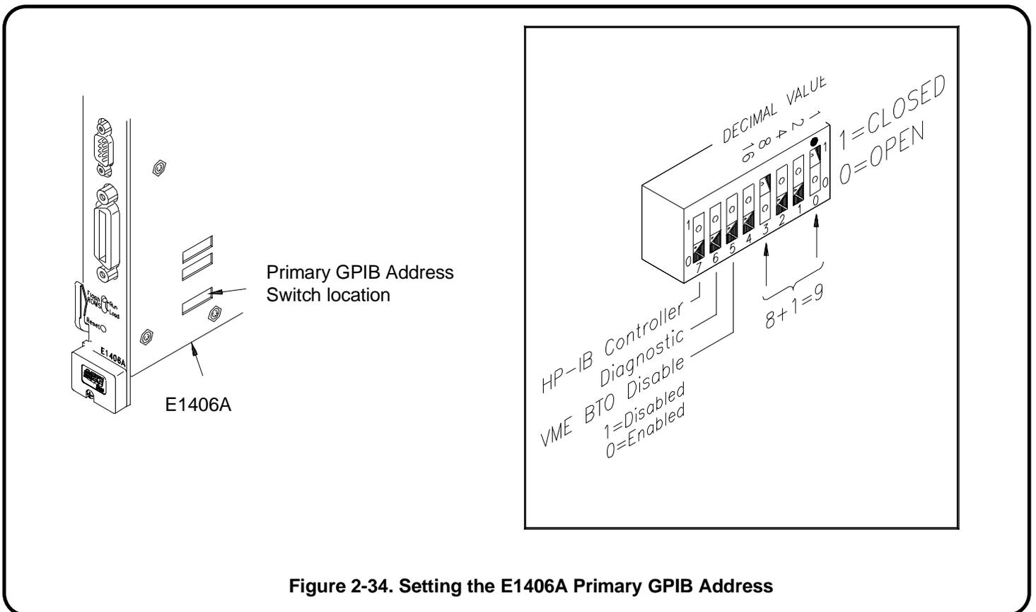
Figure 2-34. Setting the E1406A Primary GPIB Address
