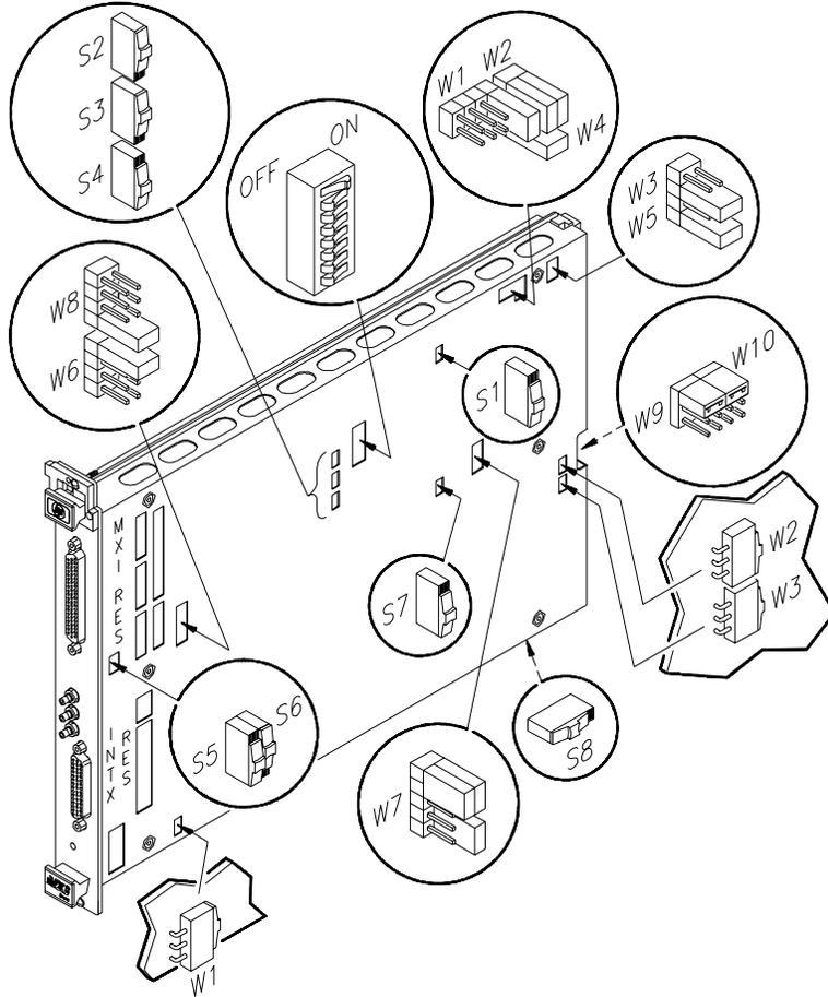
**Figure 2-14. E1482B VXI-MXI Extender Slot 0 Configuration**
