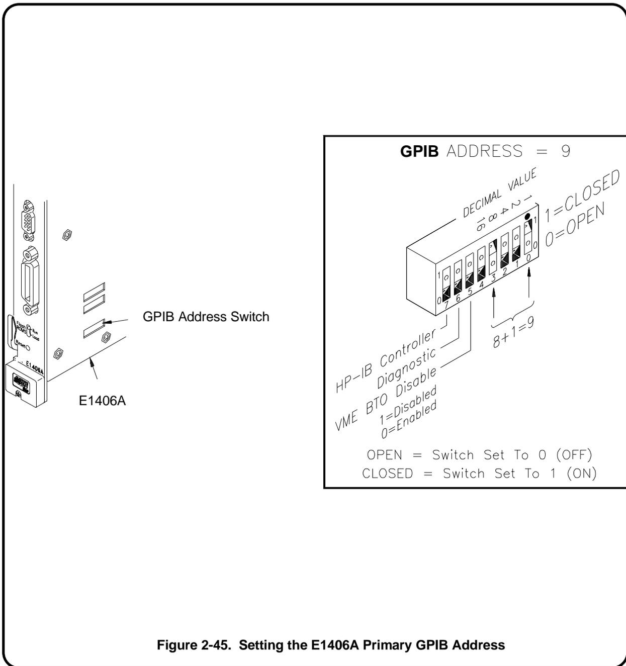
Figure 2-45. Setting the E1406A Primary GPIB Address
