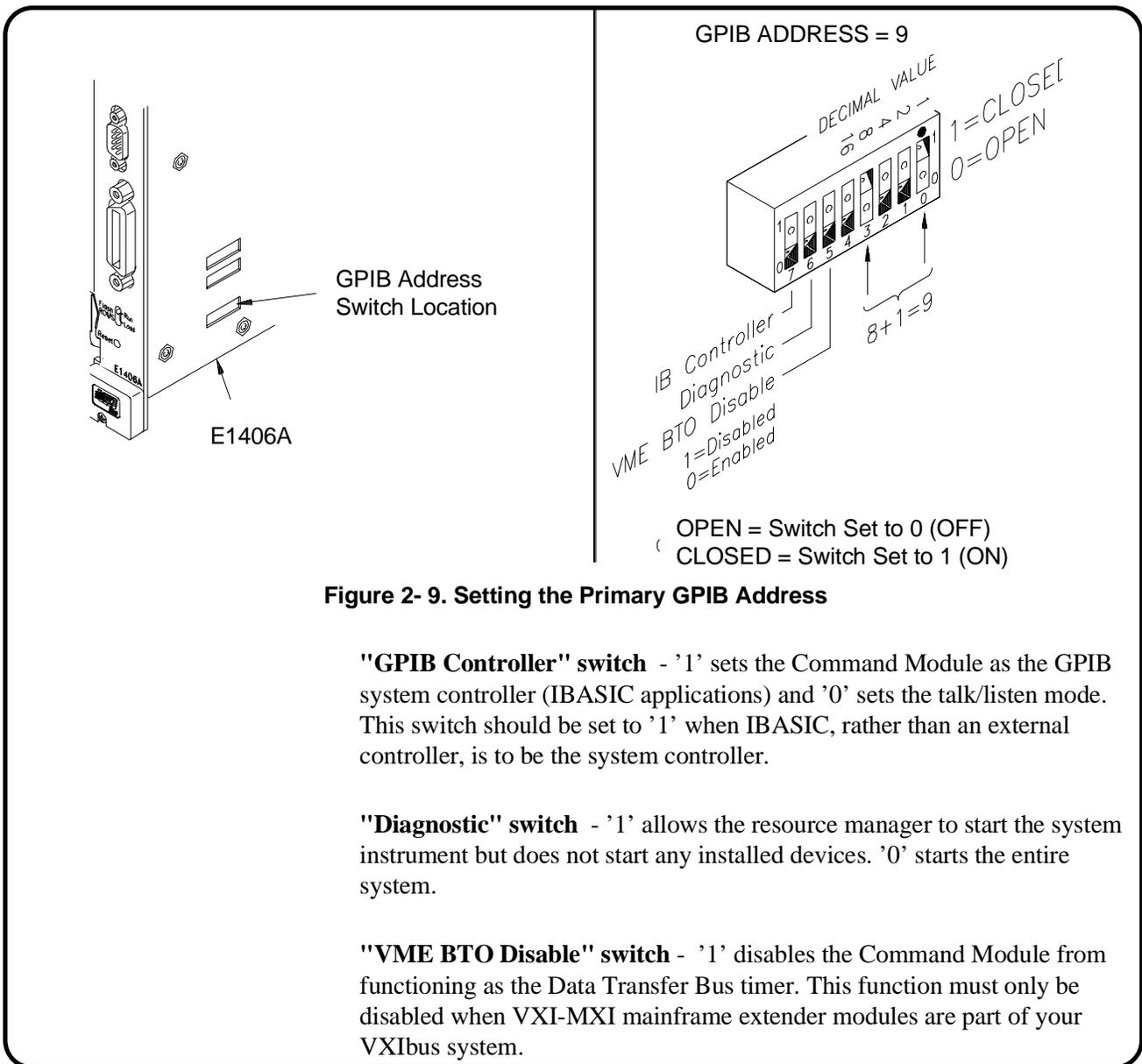
Figure 2- 9. Setting the Primary GPIB Address
