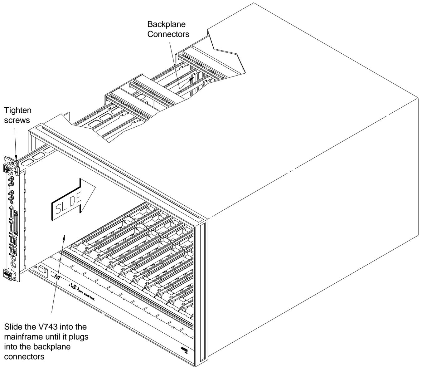
Figure 2-36. Installing the V743 Embedded Controller
