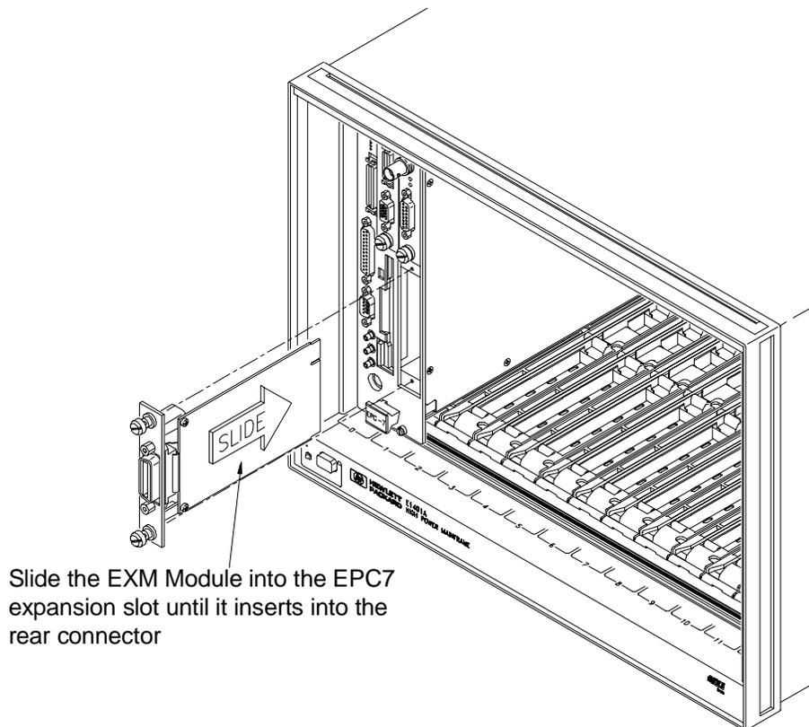
**Figure 2-42. Installing an EXM Module**
