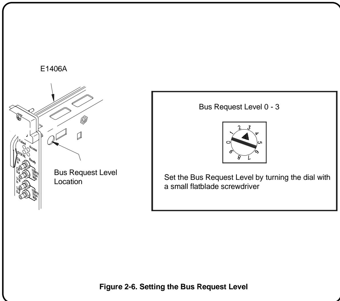
**Figure 2-6. Setting the Bus Request Level**
