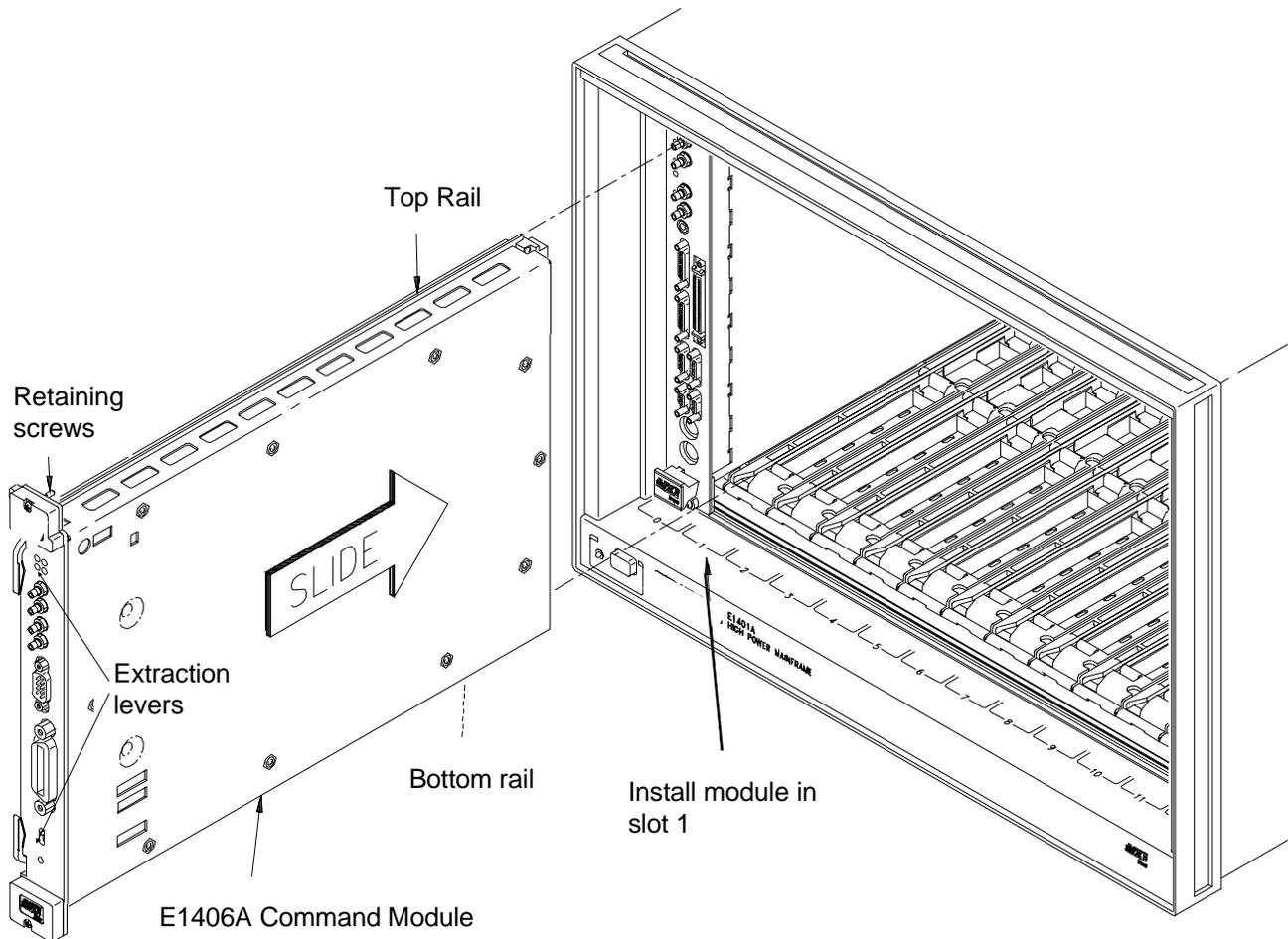
Figure 2-37. Installing the E1406A with the V743
