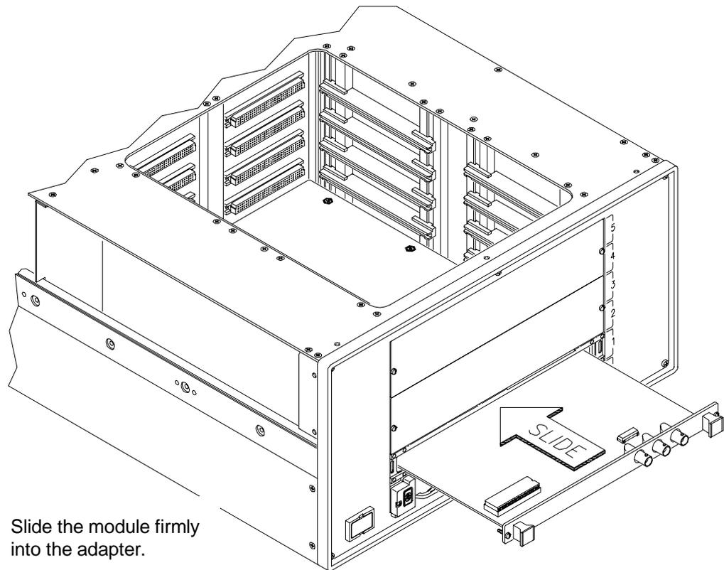
**Figure 4-3. Installing B-Size Modules in the E1421**
