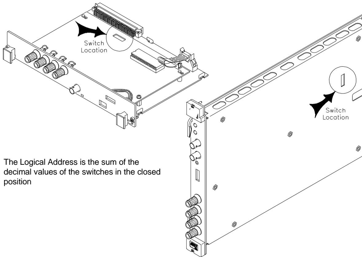
The Logical Address is the sum of the decimal values of the switches in the closed position
