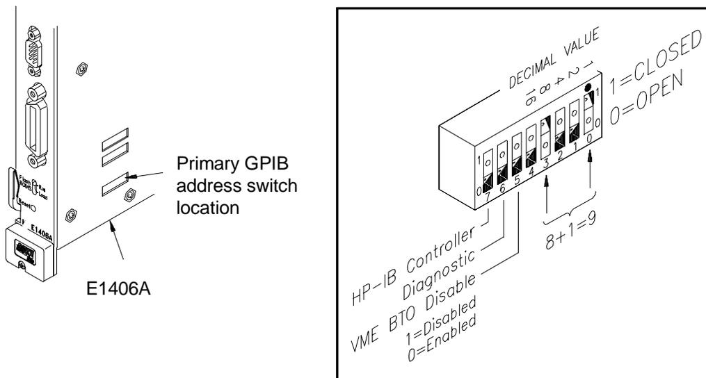
**Figure 2-17. Setting the E1406A Primary HP-IB Address**
