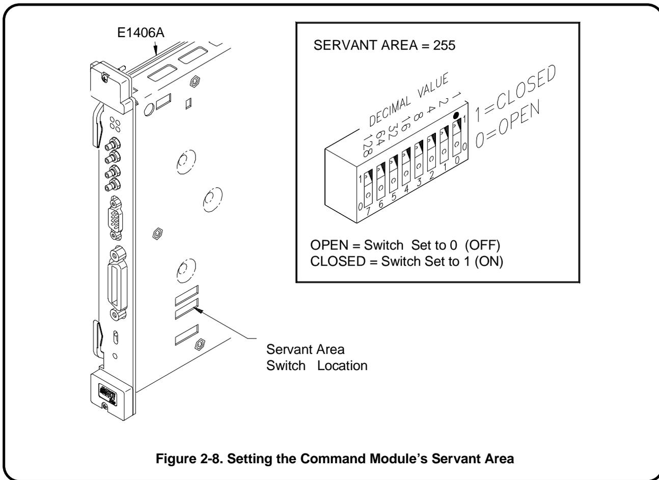
In a VXIbus system, modules in the "servant area" of another module are servants to that module (the commander). The commander module controls servant modules by translating Standard Commands for Programmable Instruments (SCPI) commands for register-based modules, or by serving as the GPIB interface to message-based modules. The concept of the servant area and commander/servant hierarchies is discussed more in Appendix A, "Terms and Definitions."
