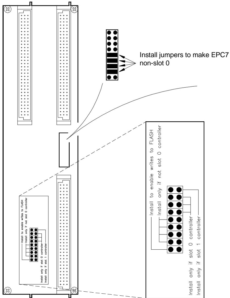
**Figure 3-21. Disabling VMEbus Timeout, HP RADI-EPC7**
