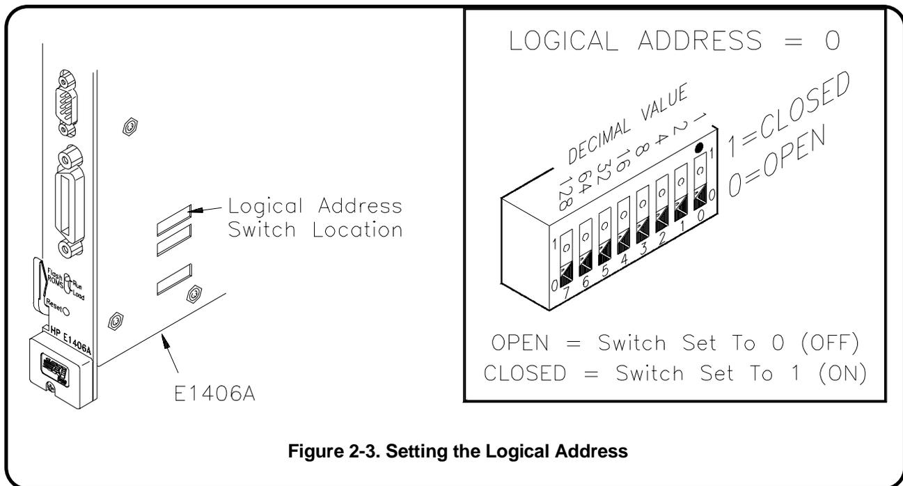
**Figure 2-3. Setting the Logical Address**
