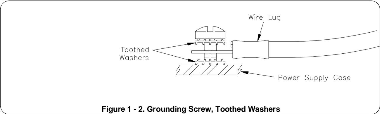
**Figure 1 - 2. Grounding Screw, Toothed Washers**
