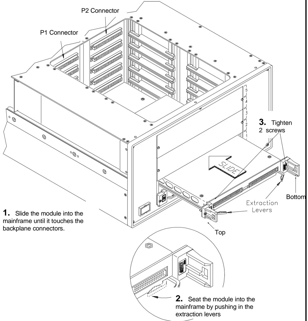
Figure 4-5. Installing C-Size Modules in the E1421
