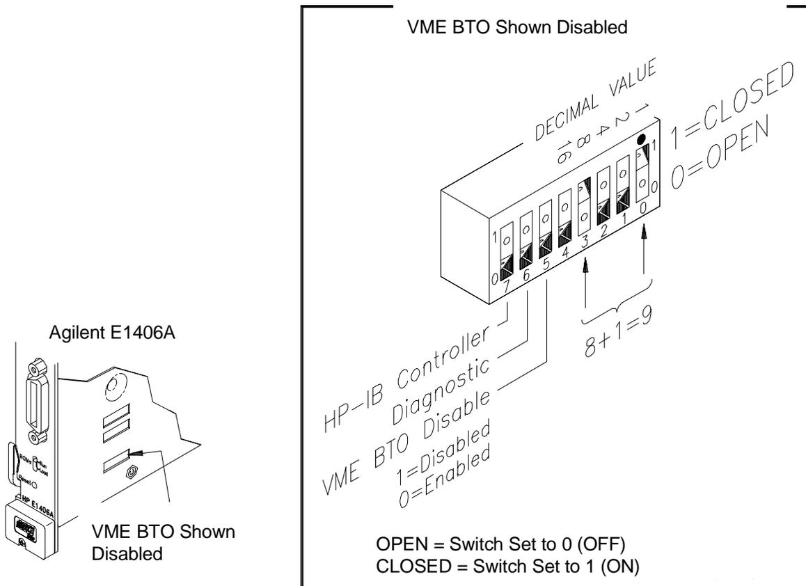
Figure 3-20. Disabling VMEbus Timeout, Command Module
