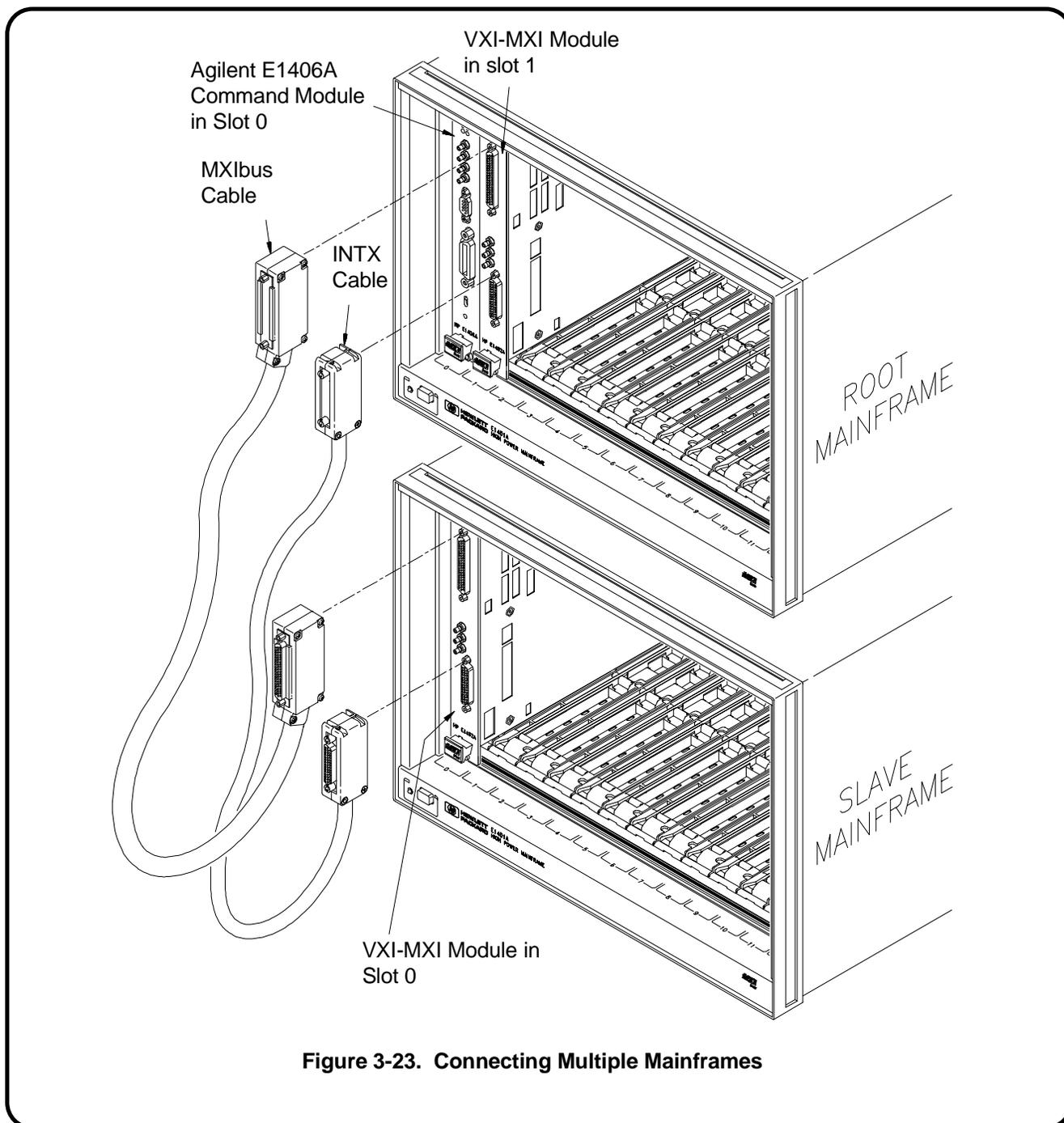
Figure 3-23. Connecting Multiple Mainframes
