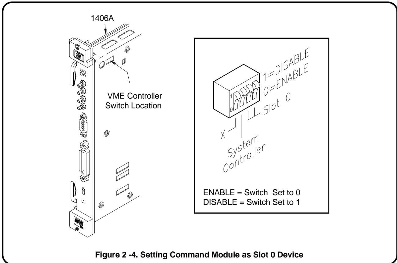
**Figure 2 -4. Setting Command Module as Slot 0 Device**
