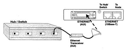
Figure 2-17: Connecting as a Node to AUI
