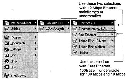
Figure 2-9: Selecting 10 Mbps Ethernet from the Start Menu
