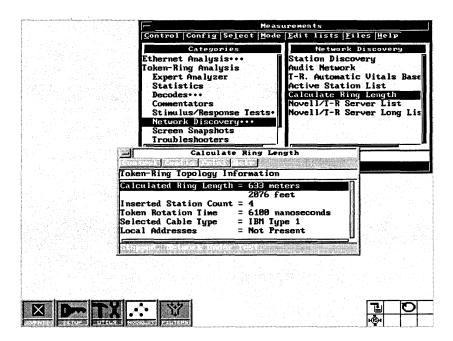
Figure 5-8: Calculate Ring Length window
