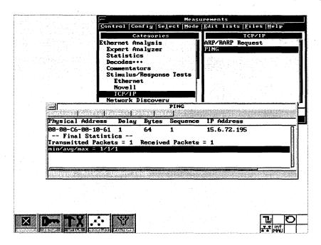
Figure 5-5: PING Configuration window
