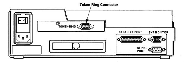
Figure 2-28: Connecting to a Token-Ring network
