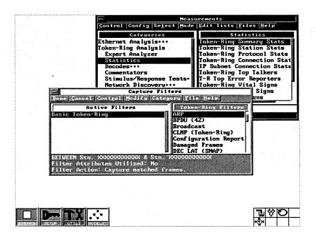
Figure 8-2: Capture Filters window with an activated filter
