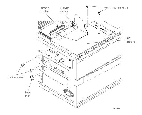
**5** Gently lift up the edge of the board that is toward the front of the instrument.
