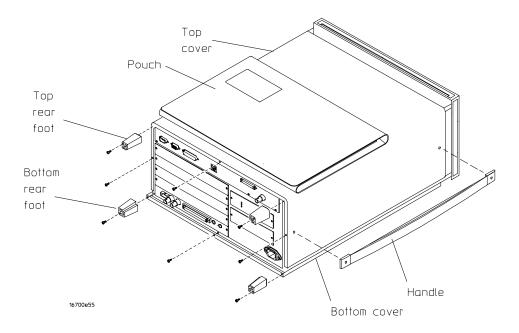
Complete steps 8 through 11 only if it necessary to remove the bottom cover.
