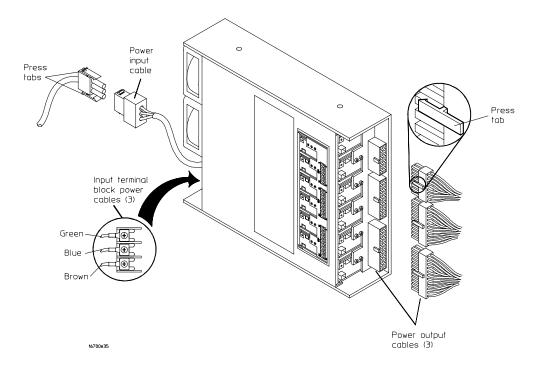
4 Using a #1 Posidrive screwdriver, remove the power input cable from the power supply input terminal block.
