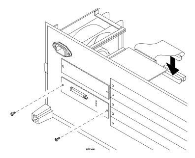
**3** Disconnect the emulation module cables from the emulation module.
