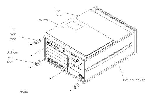
**5** Using a Torx T15 screwdriver, remove the one screw at the center rear of the cover that secures the top cover to the frame.
