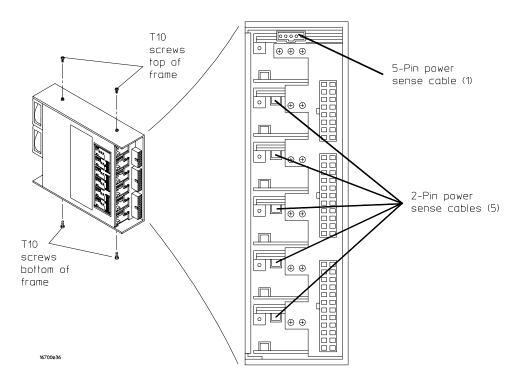
**8** Reverse this procedure to install the power supply. Use the preceding illustration to install the power sense cables.
