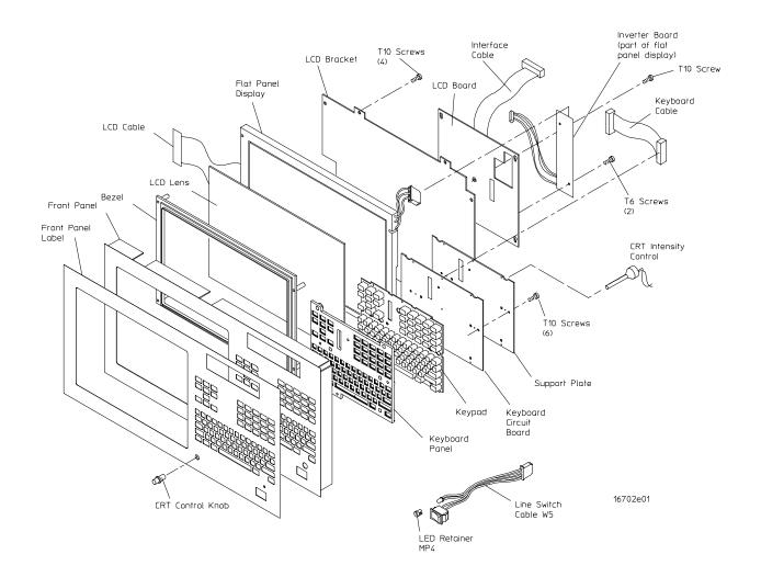
**Exploded View of the 16702A Front Panel Assembly**
