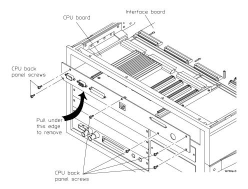
**3** Slide the CPU board out the rear of the instrument. As you remove the CPU board, it will disconnect from the interface board.
