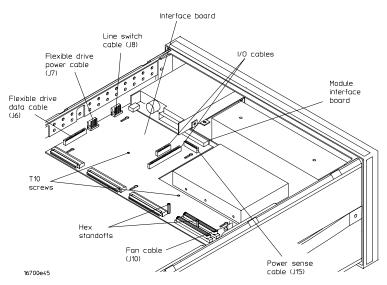
3 Using a Torx T10 screwdriver, remove the two screws that secure the interface
