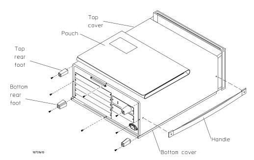
7 Slide the top cover toward the rear of the instrument and away.
