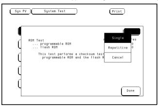
For a Single run, the test runs one time, and the screen shows the results.
