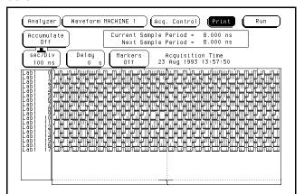
**6** On the logic analyzer, press the Run key. The display should be similar to the figure below.
