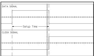
**d** Adjust the pulse generator channel 2 Delay until the pulses are aligned according the the setup time of the setup/hold combination selected, +0.0 ps or -100 ps.
