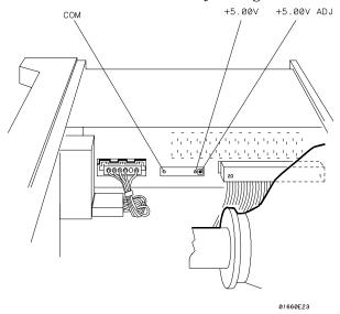
**6** Check for the voltages on the power supply cable using the values in the following table.
