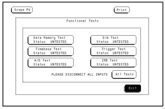
17 In the Data Memory Test menu, select Run, then select Single. The test runs one time, then the screen shows the results. When the test is finished, select Done.
