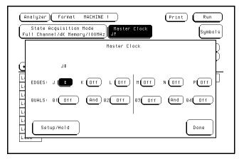
**d** In the Master Clock menu, select Setup/Hold, then select 4.0/0.0 ns for the pod being tested. Select Done. Select Done again to exit the Master Clock menu.
