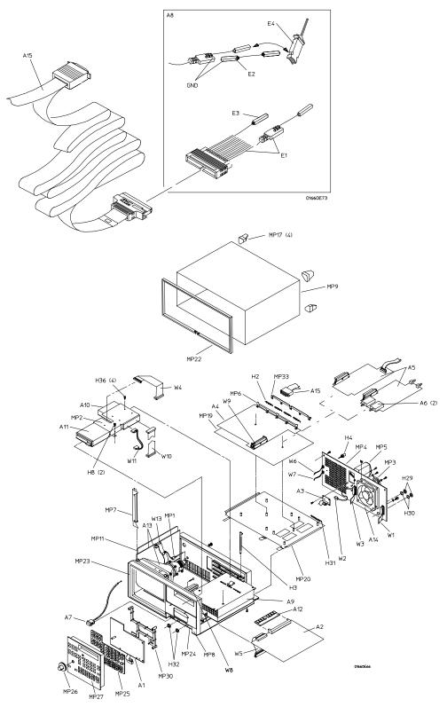
Exploded view of the HP 1660 logic analyzer.
