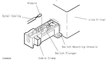
4 Remove the switch actuator assembly from the front of the cabinet.
