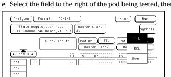
e Select the field to the right of the pod being tested, then select TTL.
