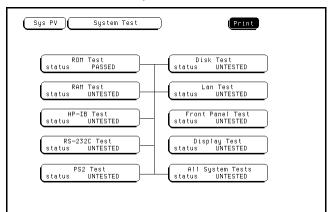
7 To exit the ROM Test, select Done. Note that the status changes to Passed or Failed.
