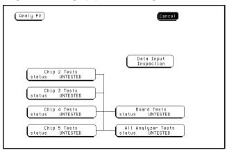
12 In the Chip 2 Tests menu, select Run, then select Single. The test runs one time, then the screen shows the results. When the test is finished, select Done. Then, perform the other Chip Tests.
