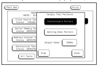
3 Using an oscilloscope, verify the existence of logic-level transitions by touching the oscilloscope probe to each channel of Data Pod 1 and doing an Autoscale. The signal levels that appear on the oscilloscope display should correspond with the logic levels represented by the 10460-series pod being used.
