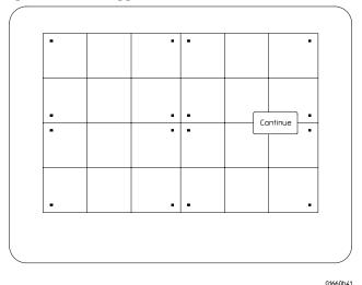
5 If the display is tilted (rotated), adjust the CRT yoke by rotating it to straighten the display.
