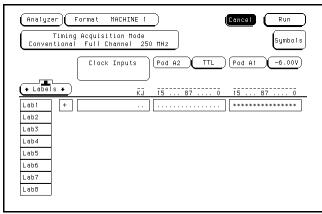
4 Using the Modify up arrow on the function generator, increase offset voltage in 1-mV increments until all activity indicators show the channels at a logic high. Record the function generator voltage in the performance test record.
