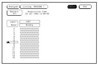
**9** If the display looks like the figure, then the cable passed the test.
