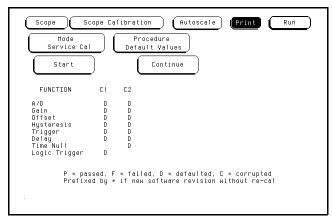
After you select the Start field, you can abort the calibration procedure by selecting either the Mode or Procedure fields if the Continue field is still displayed on the screen.
