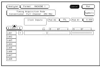
4 Using the Modify up arrow on the function generator, increase offset voltage in 1-mV increments until all activity indicators for pod 1 show the channels at a logic high. Record the function generator voltage in the performance test record.
