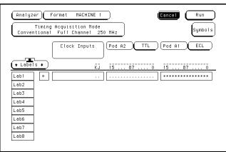
4 Using the Modify up arrow on the function generator, increase offset voltage in 1-mV increments until all activity indicators for pod 1 show the channels are at a logic high. Record the function generator voltage in the performance test record.
