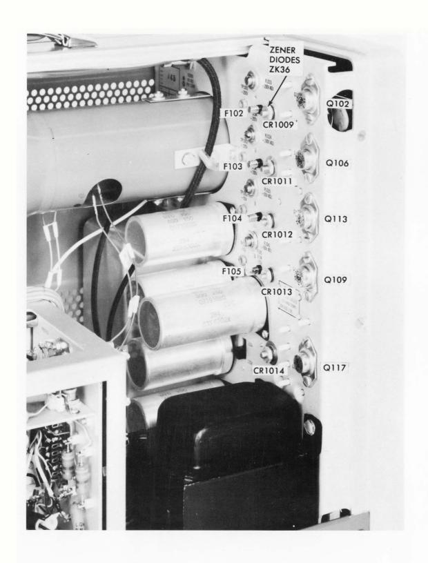
FIGURE 3-3. IDENTIFICATION OF REPLACEABLE PARTS (RIGHT SIDE VIEW)
