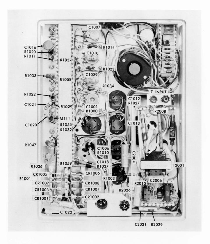
FIGURE 3-5. IDENTIFICATION OF REPLACEABLE COMPONENTS ON REAR CHASSIS
