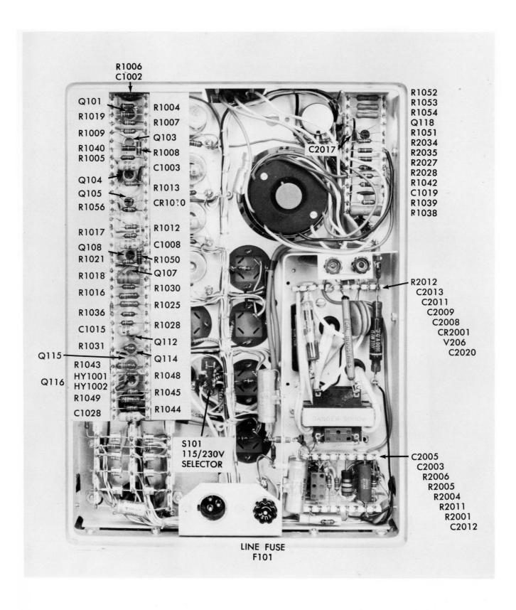
FIGURE 3-4. IDENTIFICATION OF REPLACEABLE COMPONENTS ON REAR CHASSIS
