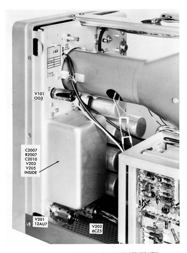
FIGURE 3-2. IDENTIFICATION OF REPLACEABLE PARTS (LEFT SIDE VIEW)
