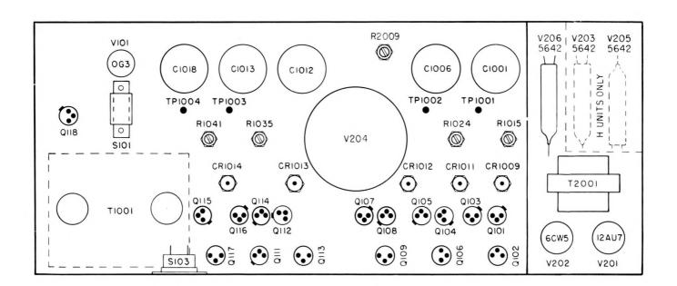
FIGURE 3-6. LOCATION OF COMPONENTS FOR RACK AND PORTASCOPE MODELS (REAR VIEW)
