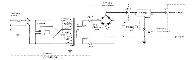
Figure 7.7 Power Supply Schematic 0271-0026
