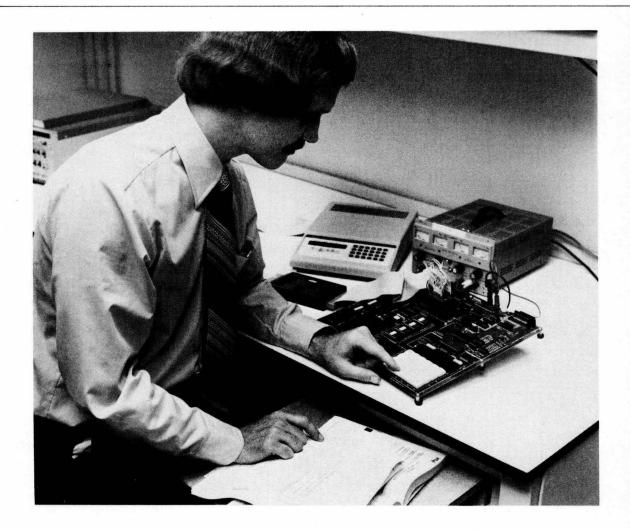
The above photograph shows the Model 2710 Logic Analyzer being used with its companion accessory, the Model 2710 MPU Adapter, on an Intel SDK 8085A board.
