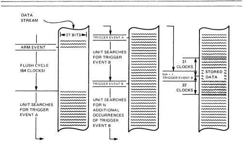
Figure 3.2. Illustration of Delay by Events (DLY E) = N (range: 0-9999 Decimal). This feature allows you to isolate specific iterations of a loop in your program.
