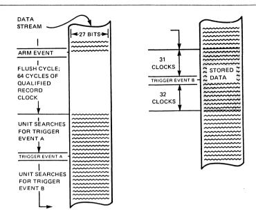
Figure 3.4. Illustration of Nested Triggering. This feature allows you easy access to otherwise difficult-to-isolate data by making it simple to trigger into specific sub-routines in your program.
