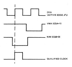
Figure 3.3 Illustration of Selective Qualification of the Record Clock. This feature allows you to achieve effective data compression by eliminating unwanted or repetitive data from a recording. The three parameters selected are as follows: active edge = rising edge, CQA = 1, and CQB = 0. The lines selected for the illustration are typical of the Motorola 6800 microprocessor.
