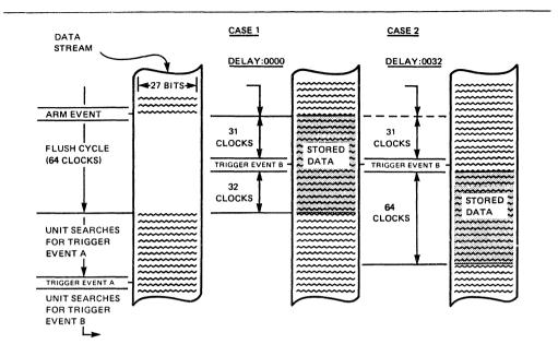
Figure 3.1. Illustration of Delay by Clocks. Case 1: DLYC = 0000. Case 2: DLYC = 0032 (range: 0-9999 Decimal). This feature allows you to slide the memory window downstream of the trigger event.
