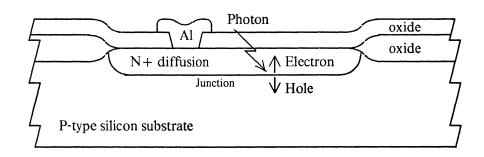
Figure 3. An NMOS Photo-Diode.
