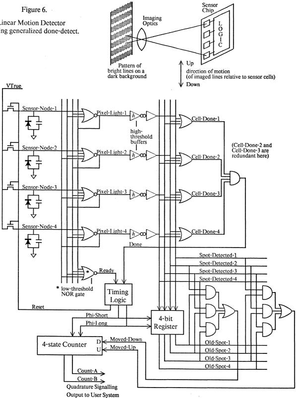
Note that we do not use the inhibition NOR gate output itself for done-detection, but a buffered version of it after a high threshold buffer (inverter pair); this is the easiest way to prevent false done-detection during a metastable condition [Seitz 1980]. The buffered signal is not used for inhibition, since that would make it participate in the metastable condition, and because the extra delay would cause oscillatory metastable states.
