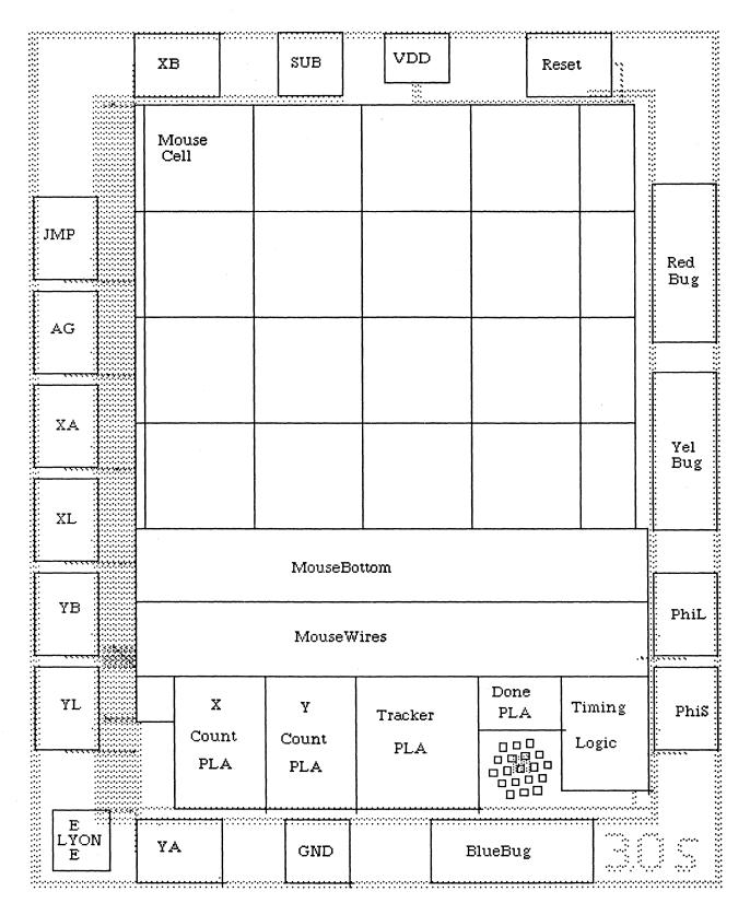
Figure 12. Floorplan of the Optical Mouse Chip
