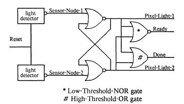
Figure 5. Two-Pixel Digital Imager
