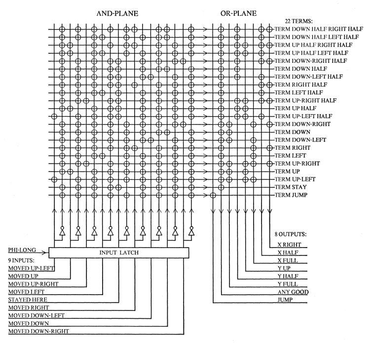
CIRCLES INDICATE GATE INPUTS TO AND-GATES (TERMS) AND OR-GATES (OUTPUTS). LOGIC EQUATIONS CAN BE READ OFF BY INSPECTION.
