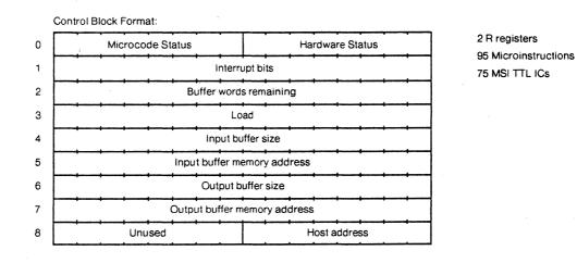
Figure 12. The Ethernet controller.
