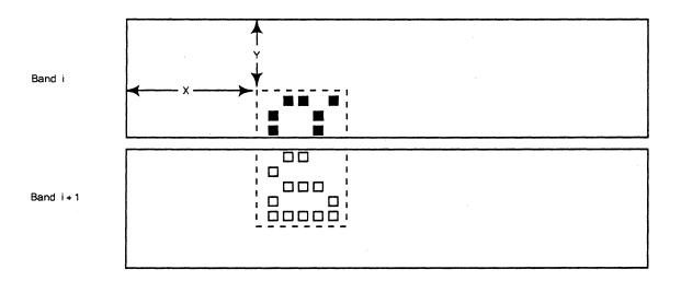
Figure 13. Schematic diagram of the image-generation process for printing a page. The band buffers show a character that does not completely fit in band i. It has a "left over" part extending into the next band.
