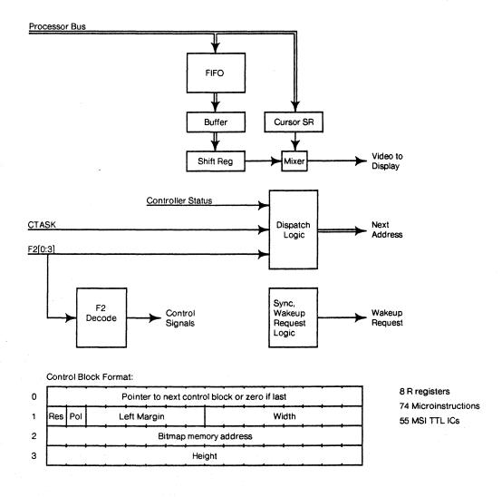
Figure 9. The display controller.
