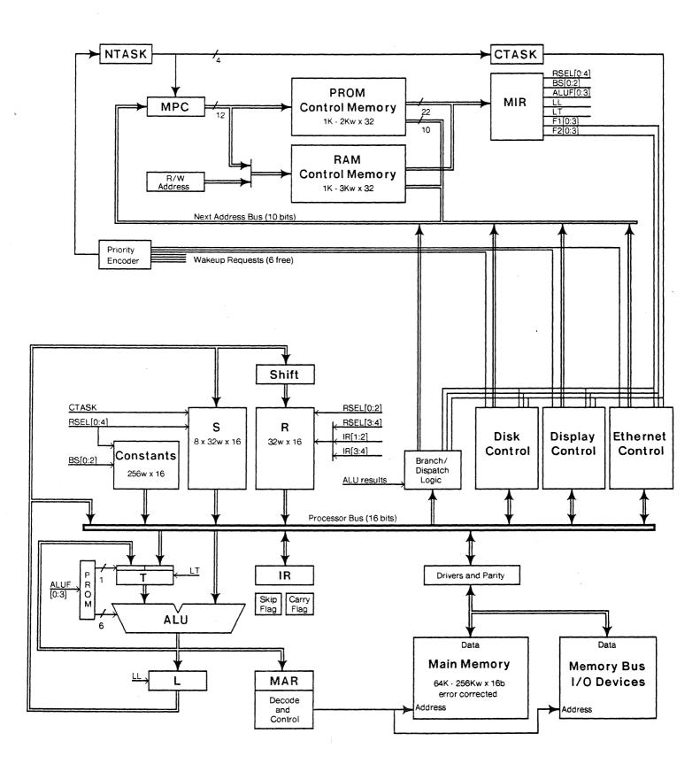
Figure 6. Alto micromachine structure.
