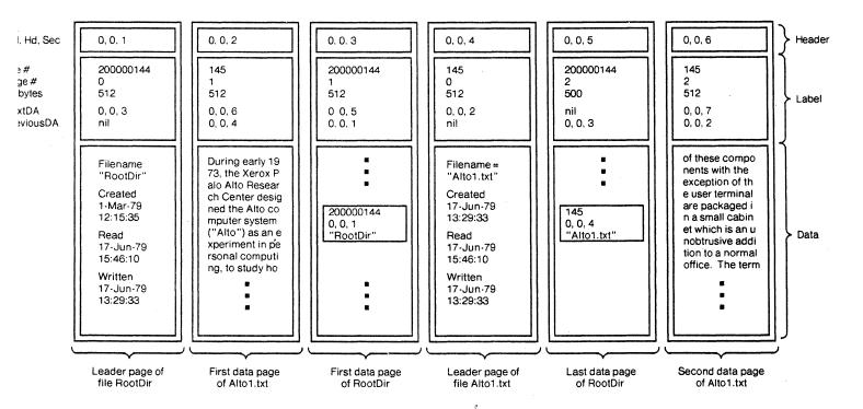
Figure 10. The Alto file system structure.
