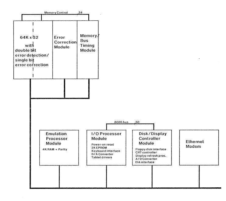
Figure 1 - NoteTaker System Block Diagram
