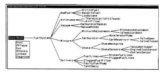
The CSRL programmer can examine his system using a specially built browser to display, edit. and run the system. The browser is a subclass of the ClassBrowser class.
