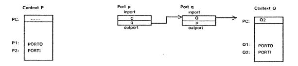
(a) Q has transferred to P via the PORTO at Q1.Control is in P, but not yet at P1Q is pending on q.
