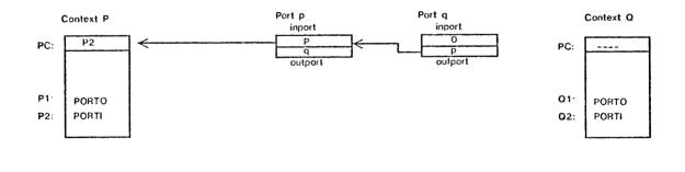
(c) Q has executed the PORTL at Q2, saving the link (an indirect link) in q outport. Any attempt to transfer to Q through q will fault, since q inport = O P is pending on p.
