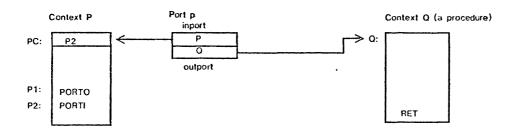
(b) P has executed the PORTO at P1, and control is in Q The link saved in Q's frame is p (an indirect link)
