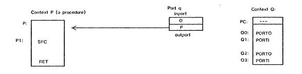
(b) Control has passed to Q, and the PORTI at Q1 has been executed. q.outport contains P (a frame pointer)
