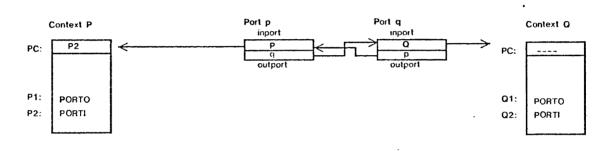
(b) P has executed the PORTO at P1, and control has passed to Q. Q has not yet executed the PORTI at Q2.
