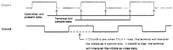
Figure 7.1.3 Terminal Interface Timing
