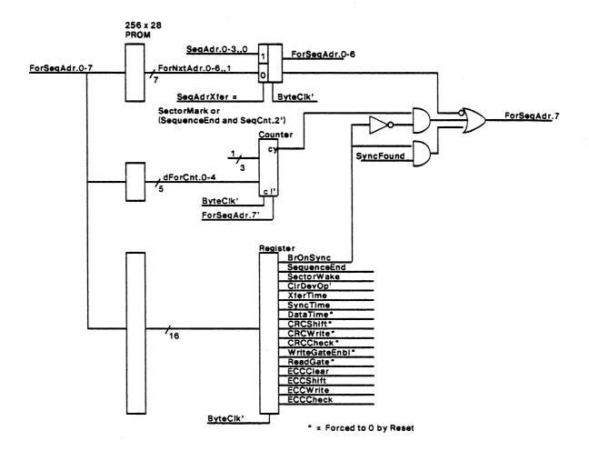
Figure 8.4.3: RDC Format Sequencer
