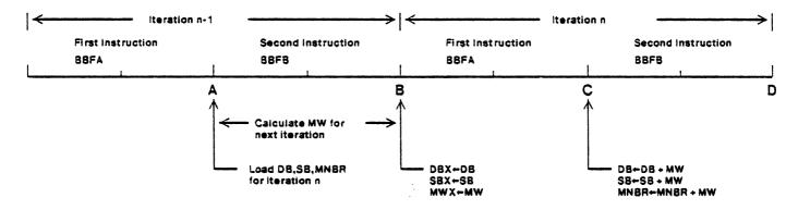
Figure 3.6.1 BitBLT Inner Loop Timing
