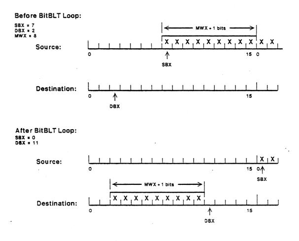
Figure 3.6.2 BitBLT Shifts and Masking
