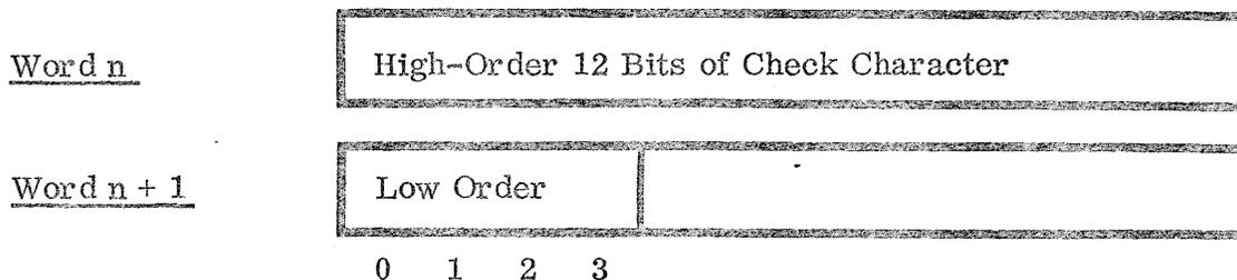
If this bit is set when a Read operation is requested (OP = 0) the two words containing the check character are transferred into memory after the data words of the sector.
