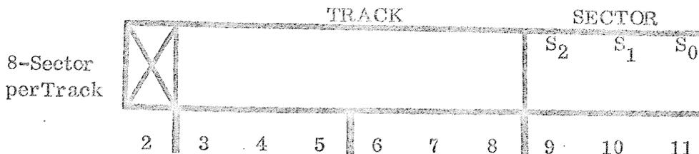
For the 10-sector/track system, no such simple correspondence holds, but the sectors are still sequentially addressed.
