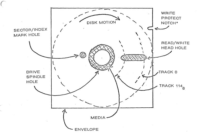
\*The WRITE PROTECT NOTCH is used only when the Write Protect option of the drive is used. Otherwise, a switch on the unit designates a write protected unit.
