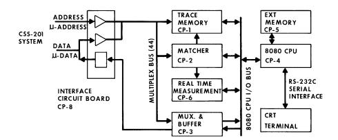
Figure 11-2 - SWAT Bus Structure (CSS 201L Interface)
