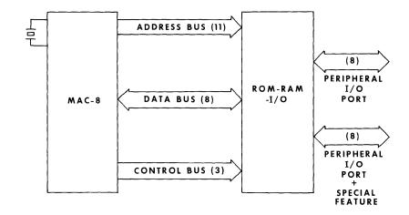
Figure 27-1 - Interconnection of a Single ROM-RAM-I/O Device
