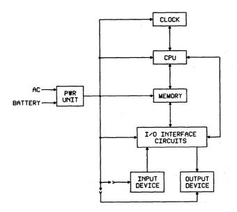
Figure 24-1 - Typical Microprocessor System
