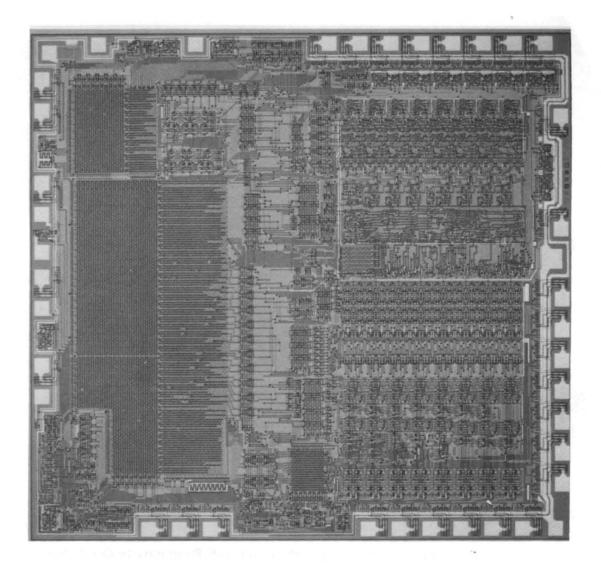
Figure 3-6 - The MAC-8 Microprocessor Chip
