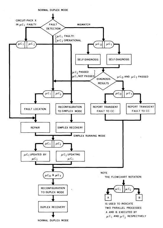
Figure 15-3 - Maintenance Functions
