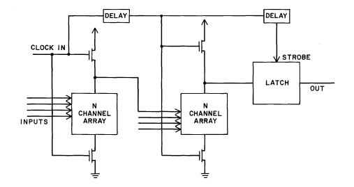
Figure 3-5 - PLA Block Diagram
