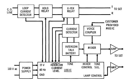
Figure 23-2 - SLS Controller Block Diagram
