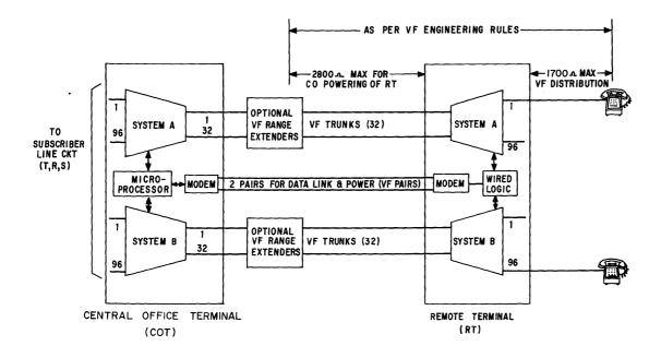
Figure 12-1 - Typical LSS System Layout - One RT
