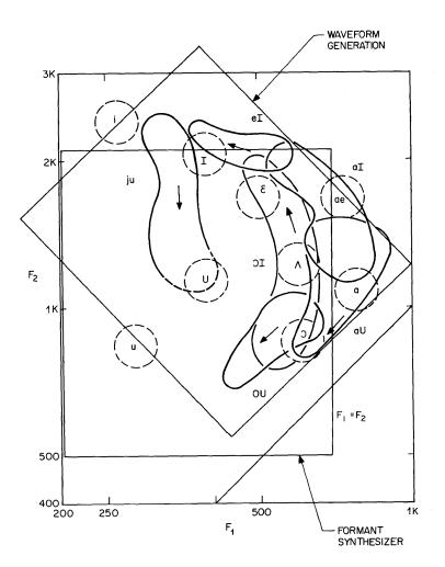
Figure 17-4 - Frequency Span of Formants One and Two in Vowels and Diphthongs
