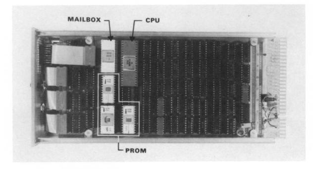
Figure 18-2(c) - Processor "One": CPU Board
