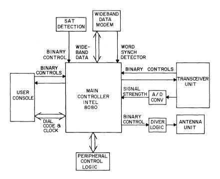
Figure 14-1 - Mobile Logic System
