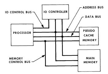
Figure 16-1 - System Structure
