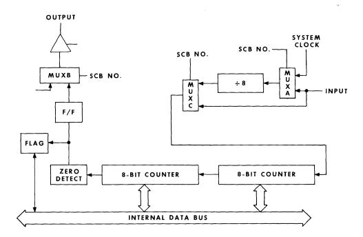
Figure 27-3 - Internal Timer Functions
