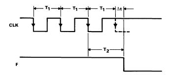
Figure 15-6 - Clock Fault Detection
