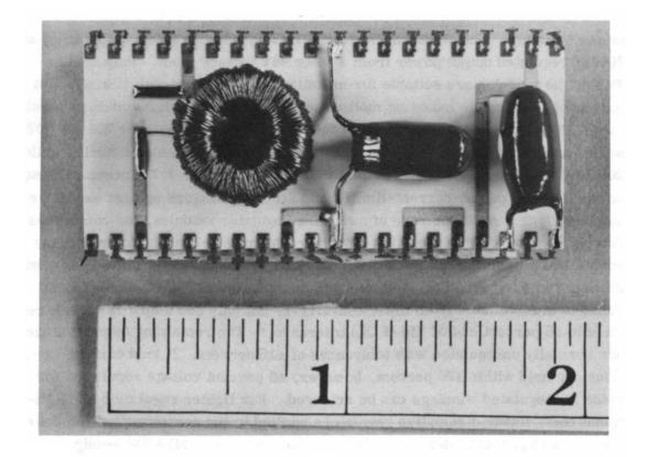
Figure 24-4 - 12V 70 mA DIP-Switching Regulator
