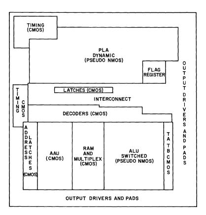
Figure 3-1 - Block Diagram of Chip
