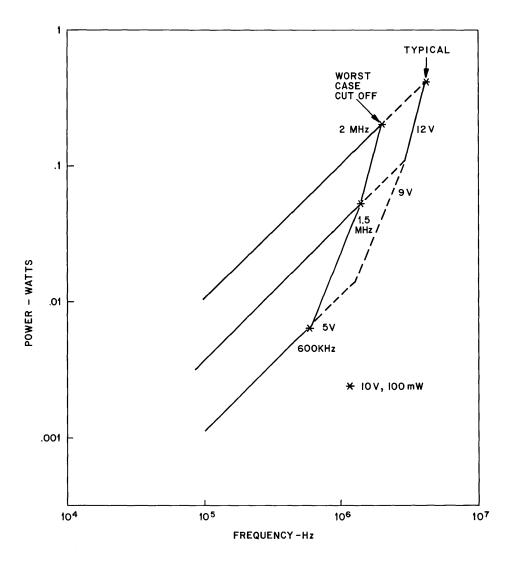
Figure 3-8 - Power vs. Frequency, Showing Worst Case and Typical Frequency Cutoffs
