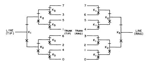
NOTE: WHEN NO TRUNK IS CONNECTED, THE  $\kappa_1,\kappa_2,$  and  $\kappa_3$  relays are latched: i.e., make contacts are closed
