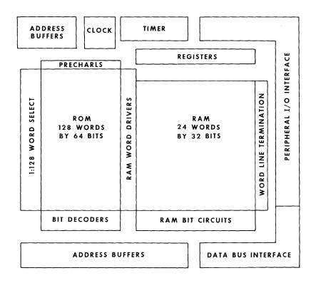
Figure 27-2 - Preliminary Placement of ROM-RAM-I/O Functions on LSI Chip
