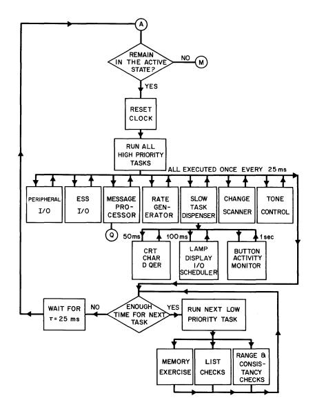
Figure 22-3 - RDI Software Flow Diagram
