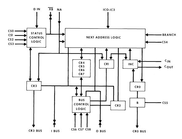
Figure 16-3 - Microprogram Control Function
