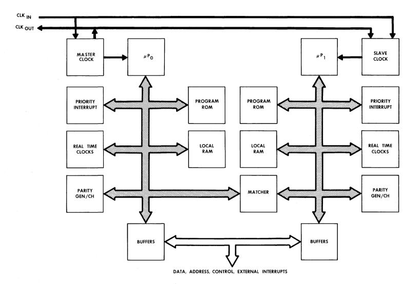
Figure 15-4 - Hard Core Block Diagram
