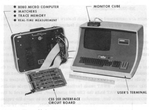
Figure 11-1 - CSS 201 Switch Analysis Tool (SWAT)
