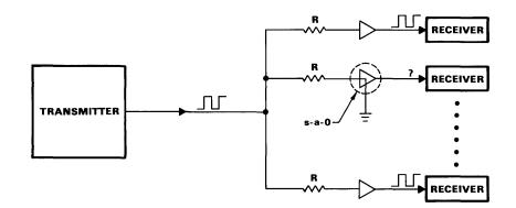
Figure 15-7 - Isolation of Input Faults
