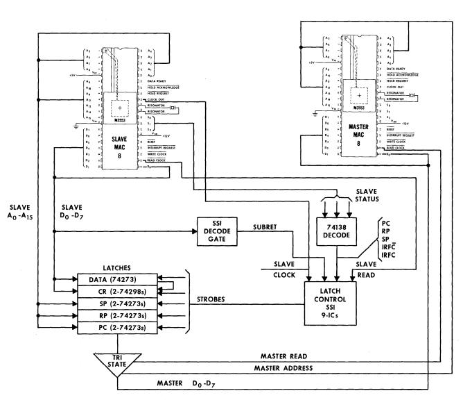
Figure 5-7 - Snapshotting MAC-8 Registers
