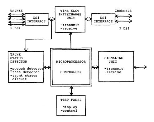
Figure 13-1 - TASI-E Microprocessor Interfaces
