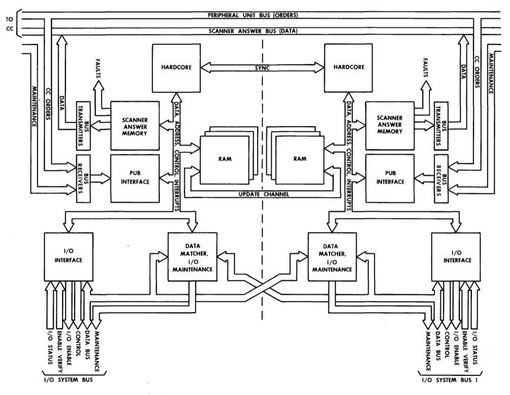
Figure 15-2 - Duplicated Microcomputer Block Diagram
