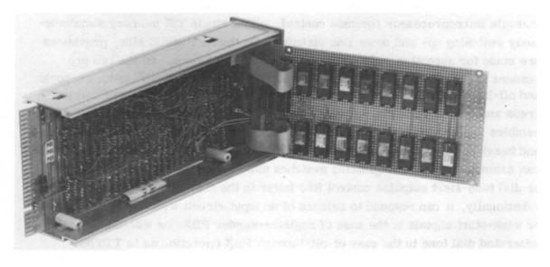
Figure 18-2(b) - Processor "One": RAM Board
