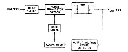
Figure 24-3 - Switching Regulator Block Diagram
