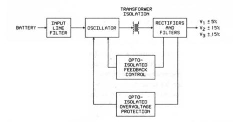
Figure 24-5 - DC-to-DC Converter Block Diagram
