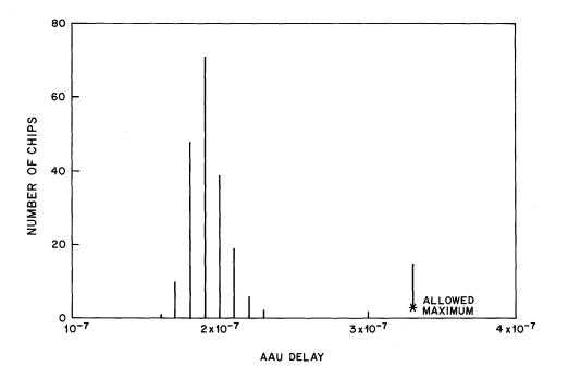
Figure 3-7 - AAU Delay for 16-Bit Increment for 196 Functionally Good Chips
