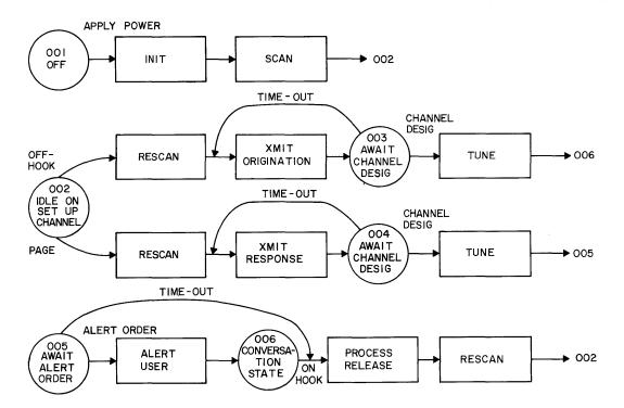
Figure 14-3 - Simplified State Diagram
