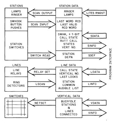
Figure 21-13 - System Data Buffering
