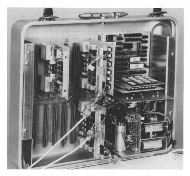
Figure 21-2 - Printed Circuit Card Arrangement
