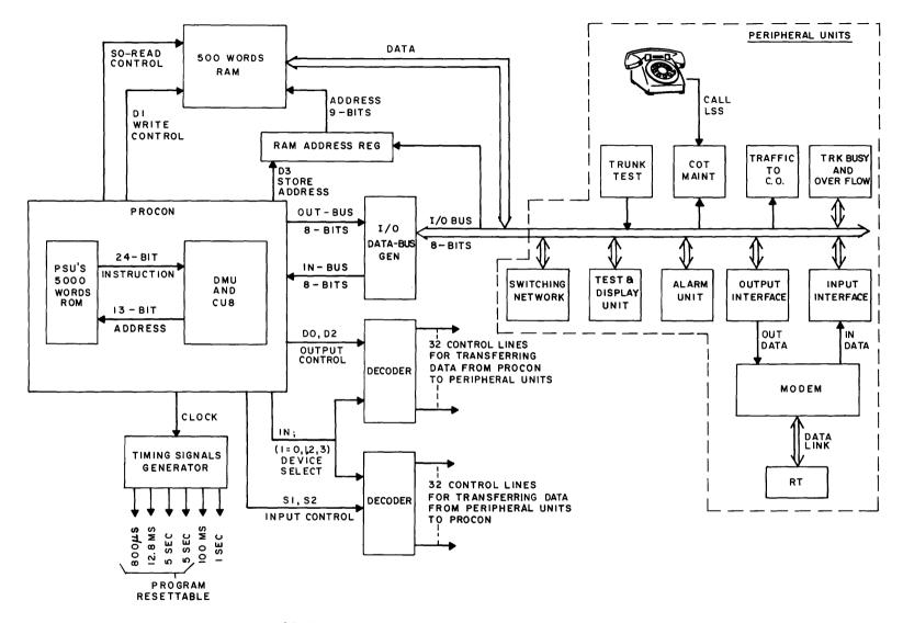
Figure 12-6 - Block Diagram Showing Communication Paths Between PROCON, COT Units, and the RT
