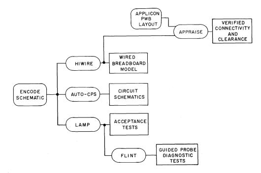
Figure 10-1 - CADRE System for Logic Circuit Pack Design
