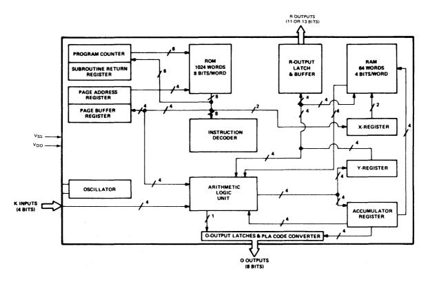
Figure 23-4 - TMS 1000 Computer Block Diagram
