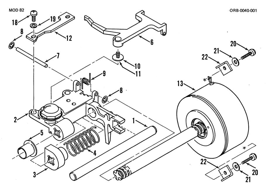
Figure D-3 Model 82 Microfloppy - Carriage Assembly
