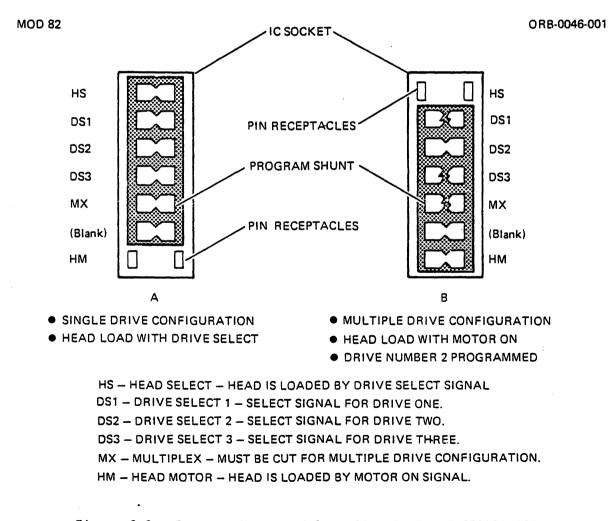
Figure 2-8. Program Shunt Module - Circuit Board 650191-001
