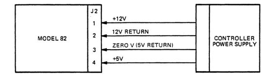
Figure 2-5. Interface Signals - Model 82
