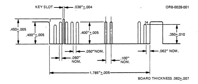
Figure 2-3. Connector Dimensions - J1
