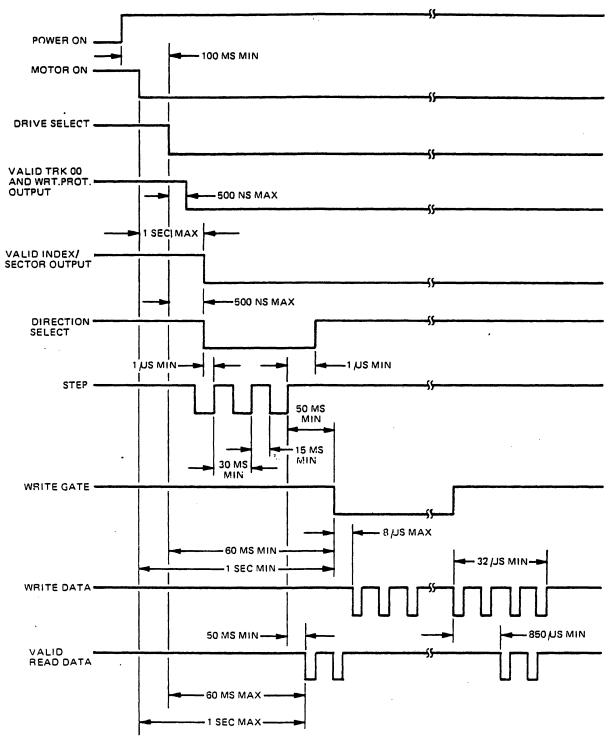
Figure 2-6. Model 82 Interface Timing Requirements
