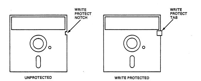
Figure 3-1. Write Protect Feature
