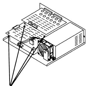
3 Remove four screws securing motherboard.
