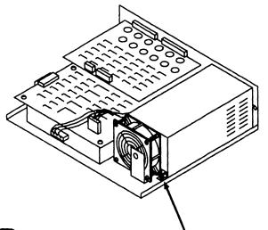
3 Remove screw securing power supply to chassis bottom.
