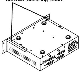
3 Remove two screws at bottom front.
