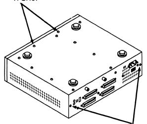
4 Remove two screws on rear panel.
