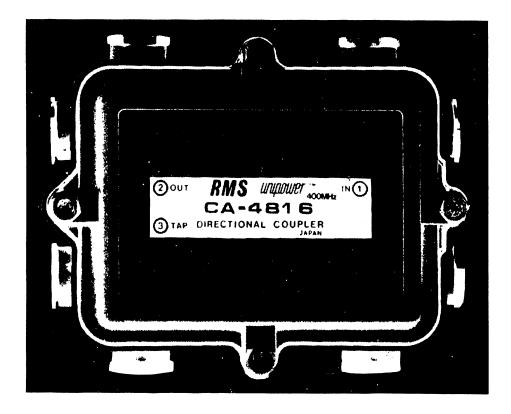
Figure 2-22 Typical Directional Coupler Exterior View
