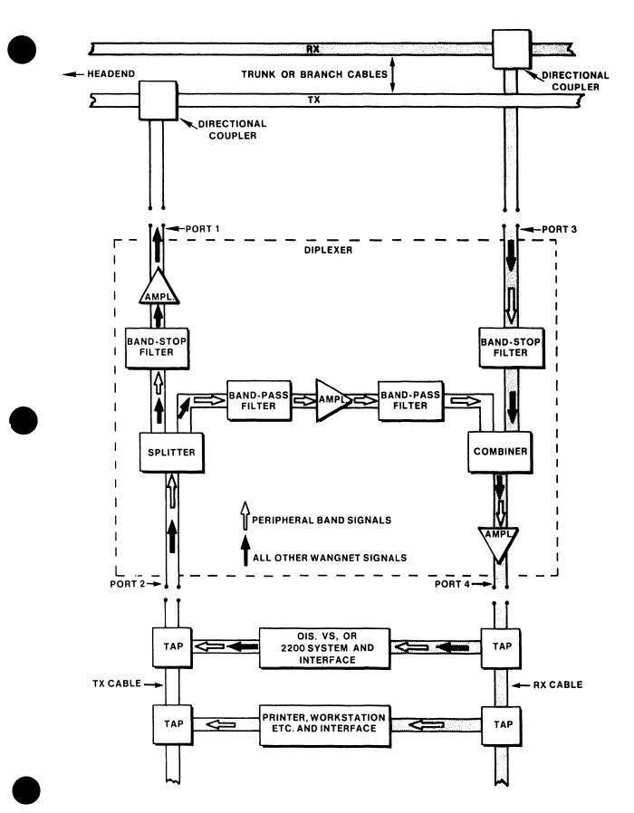
Figure 2-12 Diplexer Block Diagram
