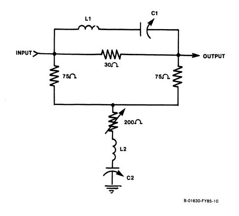
Figure 2-11 Adjustable Equalizer Schematic
