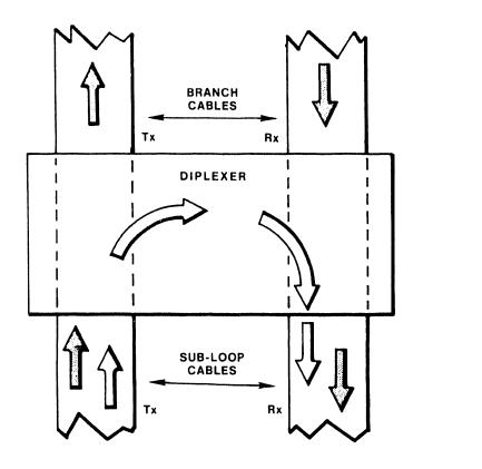
Figure 2-4 Diplexer Functional Diagram
