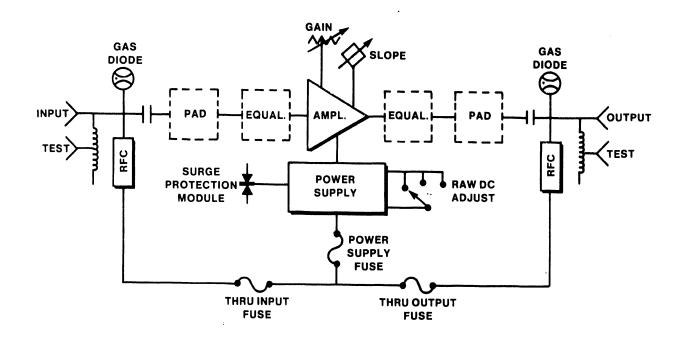
Figure 2-5 Amplifier Block Diagram
