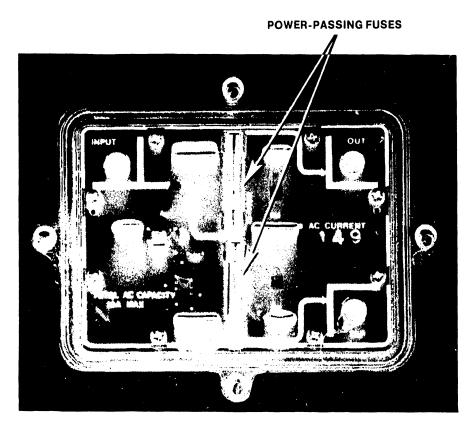
Figure 2-23 Typical Directional Coupler Interior View
