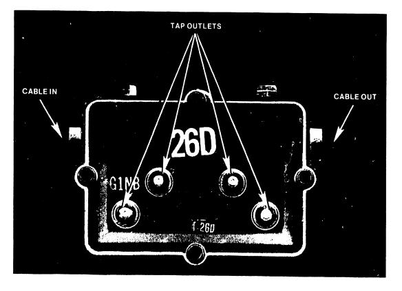
Figure 2-26 Typical Directional Tap Exterior View
