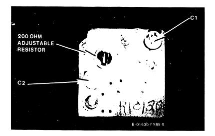
Figure 5-9 Adjustable Equalizer Controls
