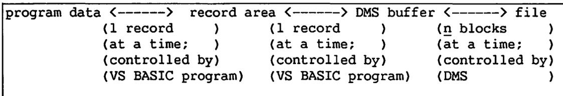
Figure 8-1. The Data Transfer Path
