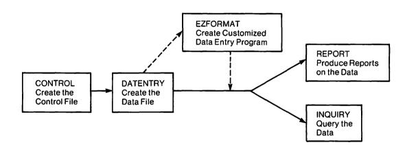
Figure 1-1. Data Processing With the Data File Management Utilities
