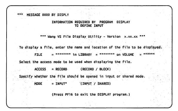
Figure 8-2. DISPLAY Input Definition Screen
