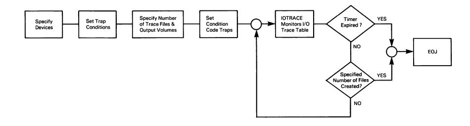
Figure 16-1. IOTRACE Processing
