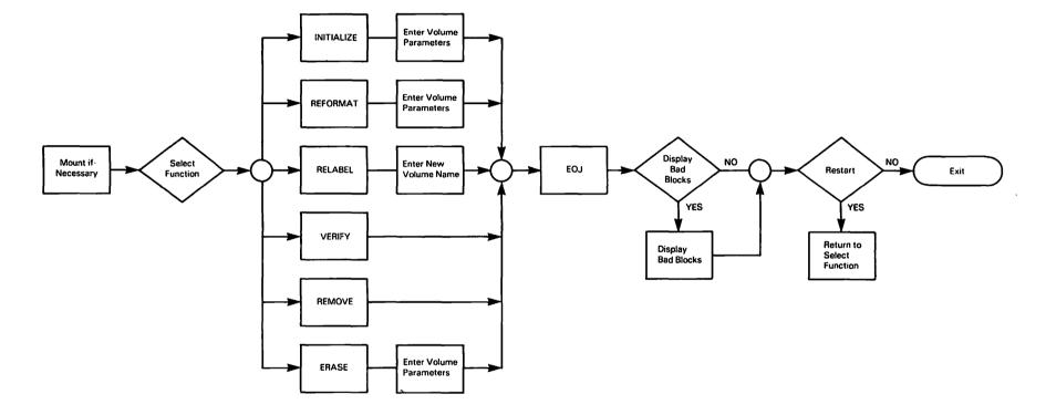
Figure 7-2. DISKINIT Processing
