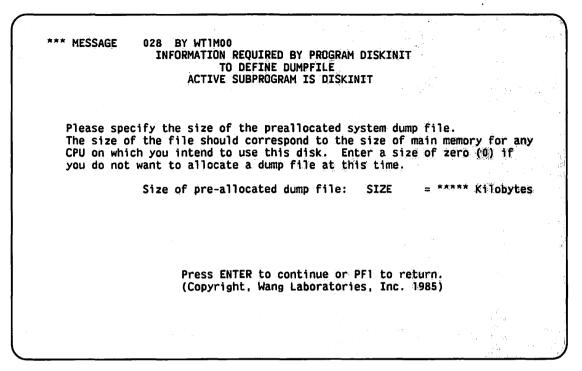
Figure 7-8. DISKINIT Dump File Size Definition Screen
