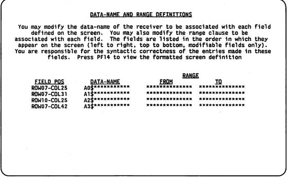
Figure 9-8. EZFORMAT BASIC Data-Name and Range Definitions Screen
