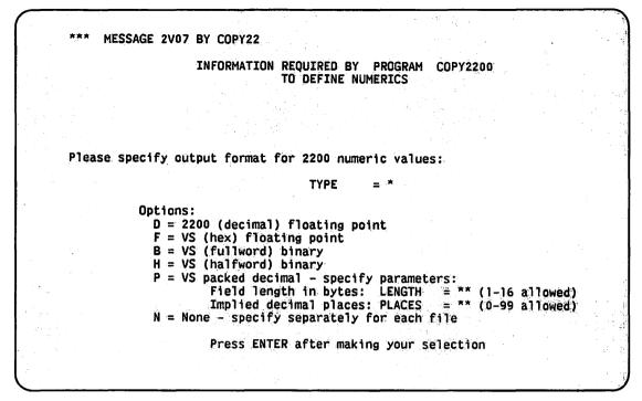
Figure 5-6. Numeric Data Format Screen
