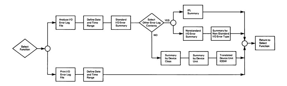
Figure 15-2. IOELOG Processing
