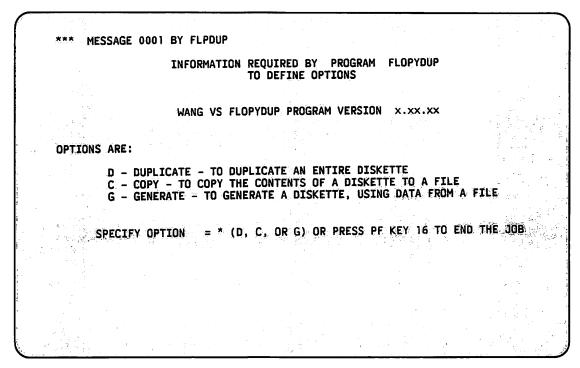
Figure 11-2. FLOPYDUP Function Selection Screen
