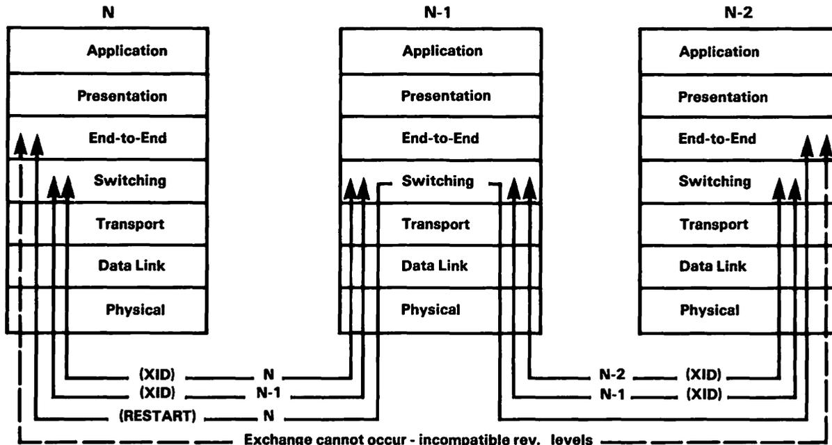
Figure 5-2. Path through a System with Incompatible CNS Revision
