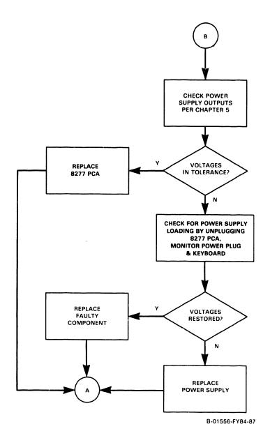
Figure 8-2. 4220 Workstation Troubleshooting Flowchart (Sheet 2 of 4)
