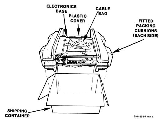
Figure 4-3. Unpacking the Electronics Base
