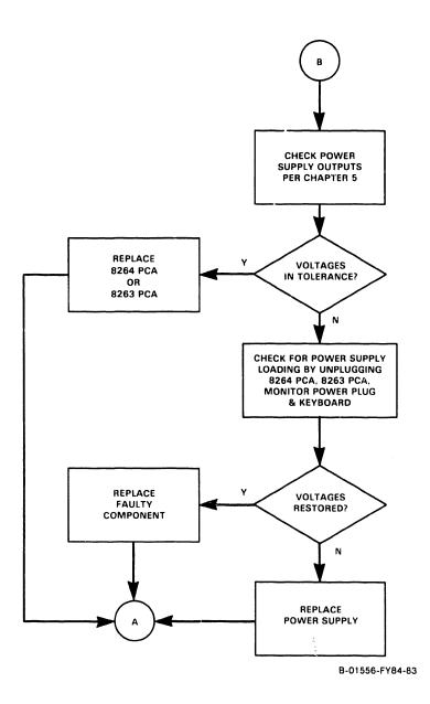
Figure 8-1. 4210 Workstation Troubleshooting Flowchart (Sheet 2 of 4)
