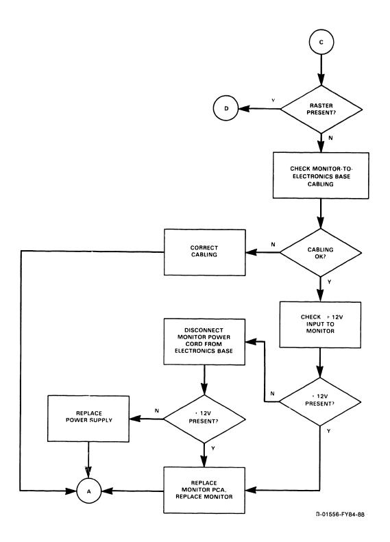
Figure 8-2. 4220 Workstation Troubleshooting Flowchart (Sheet 3 of 4)
