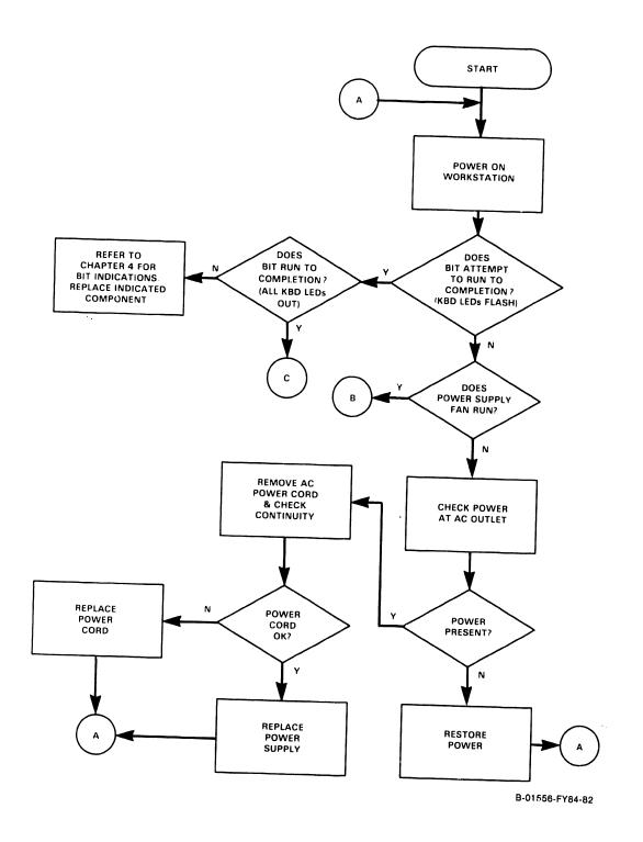
Figure 8-1. 4210 Workstation Troubleshooting Flowchart (Sheet 1 of 4) ۰,
