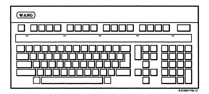
The Keyboard features the conventional typewriter format, cursor control and editing keys, and special function keys. The special function keys are those normally associated with Wang WP systems (INDENT, FORMAT, SRCH, COMMAND, etc.) and those normally associated with data processing systems (Program Function keys). The Keyboard is also equipped with a numeric keypad at the extreme right.
