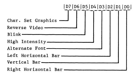
Bit 7 enables character set graphics. This causes the 8-bit wide character to expand horizontally to fill the 10-bit wide character cell. Figure 2-7 illustrates the normal 8 x 12 area defined by the font and shows how columns 2 and 7 are expanded to the edges of the character cell with character set graphics.
