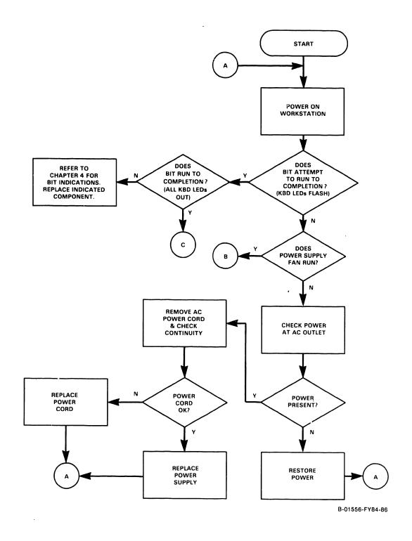
Figure 8-2. 4220 Workstation Troubleshooting Flowchart (Sheet 1 of 4)
