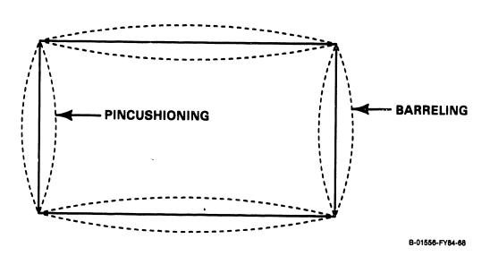
Figure 5-5. Pincushioning/Barreling Correction
