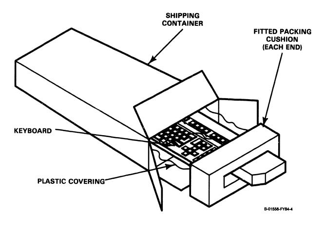
Figure 4-2. Unpacking the Keyboard
