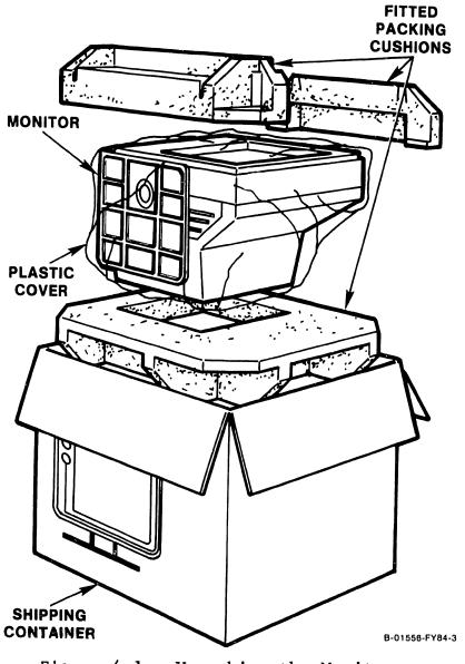
Figure 4-1 Unpacking the Monitor
