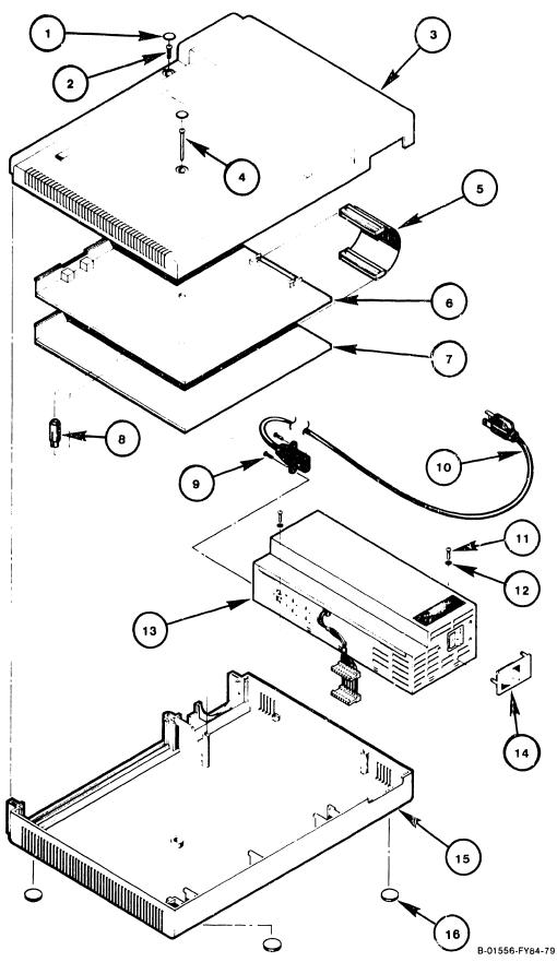
Figure 7-1. Electronics Base Assembly
