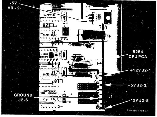
Figure 5-1. 4210 Power Supply Checks
