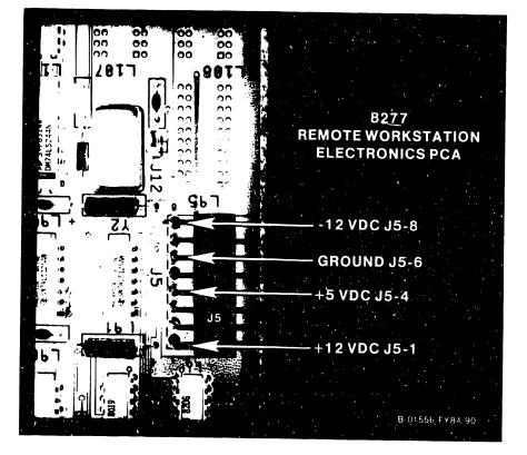
Figure 5-2. 4220 Power Supply Checks
