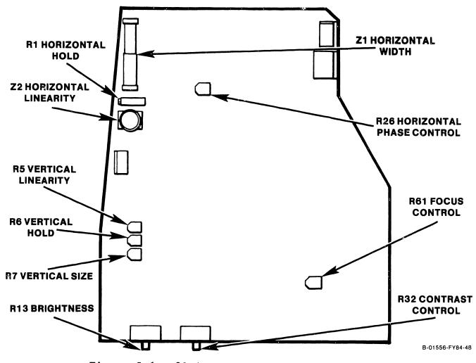
Figure 5-6. 8344 Test Points and Adjustments
