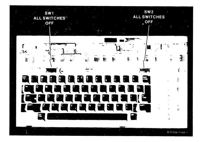
Figure 5-14. Keyboard Switch Settings (4210/4220)
