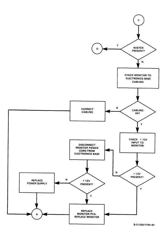
Figure 8-1. 4210 Workstation Troubleshooting Flowchart (Sheet 3 of 4)
