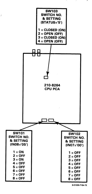
Figure 5-13. 210-8264 CPU PCA Switch Settings (4210)
