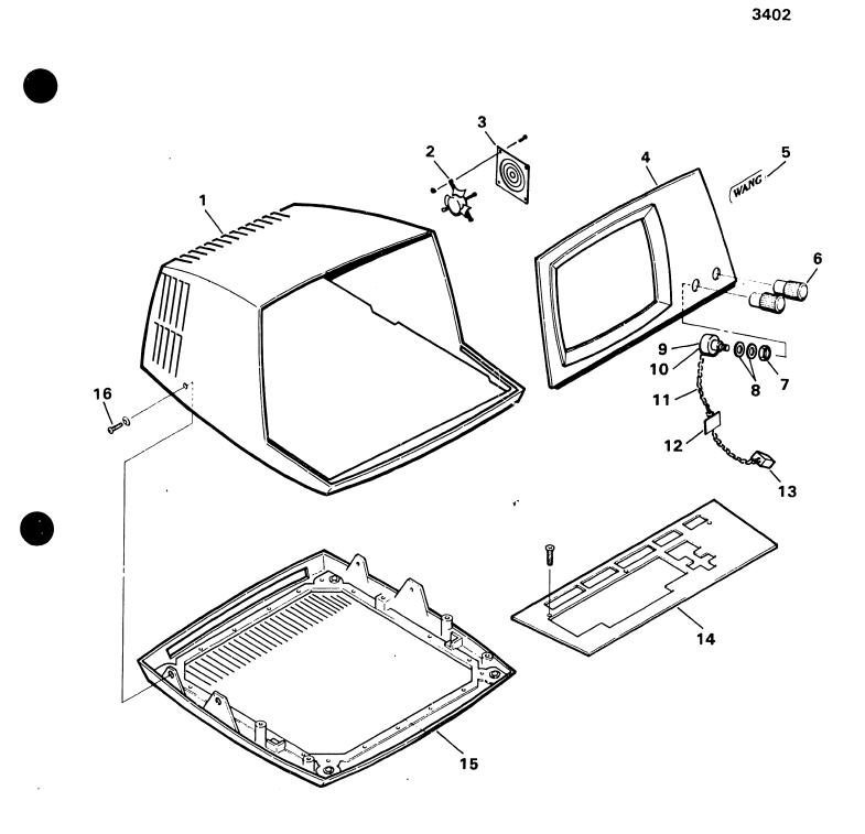
FIGURE 7-1 EXTERNAL COVERS ASSEMBLY (ASSEMBLY PART NO. 279-4128)
