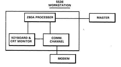
Figure 2-9. 5536 Workstation with TC Configuration
