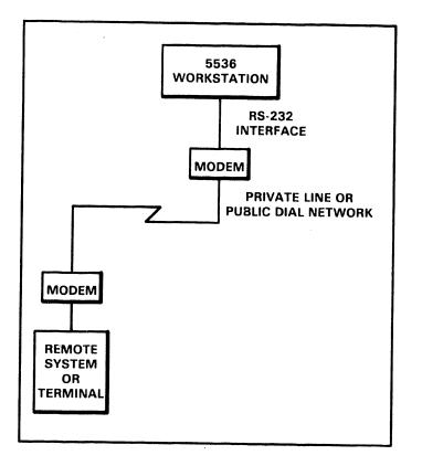
Figure 2-10 TC Connection Diagram
