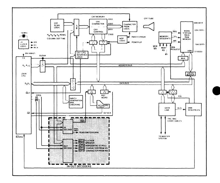
Figure 2-5. I/O Decoding
