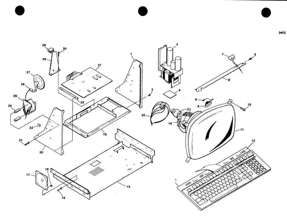
FIGURE 7-2 12" MONITOR ASSEMBLY (ASSEMBLY PART NO. 270-0372)
