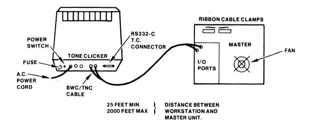
Figure 4-2. Workstation Cable Interconnections
