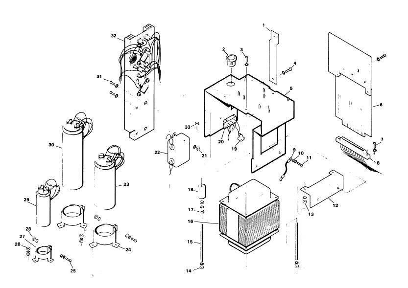
FIGURE 7-4 POWER SUPPLY ASSEMBLY (ASSEMBLY PART NO. 279-0526) or 270-0879 (FCC)
