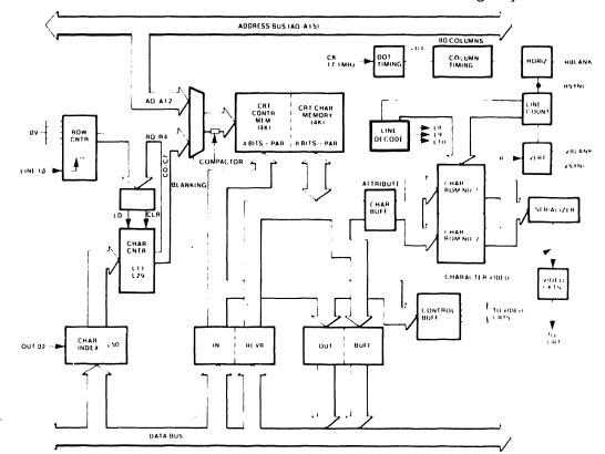
Figure 2-2. Video Display and Control Block Diagram
