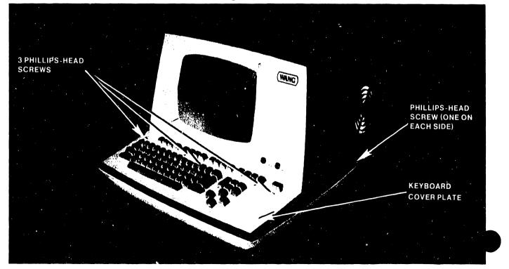
Figure 5-4. Cover Removal/Replacement
