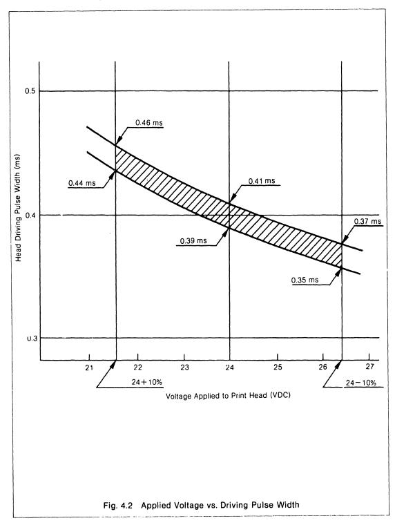
The method of determining such a head driving pulse width as that assures the relationship shown in Fig. 4.2 is as follows.
