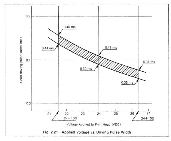
The Printer has been adjusted so that the head driving pulse width becomes 0.4 msec when +24VDC is applied to the print head.
