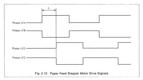
As shown in Figs. 2.9 and 2.10, the respective stepper motors are driven by two twophase excitation signals. However, the driving pulse width  $t_1$  of the carriage stepper motor differs depending on the type of character to be printed, as shown below.
