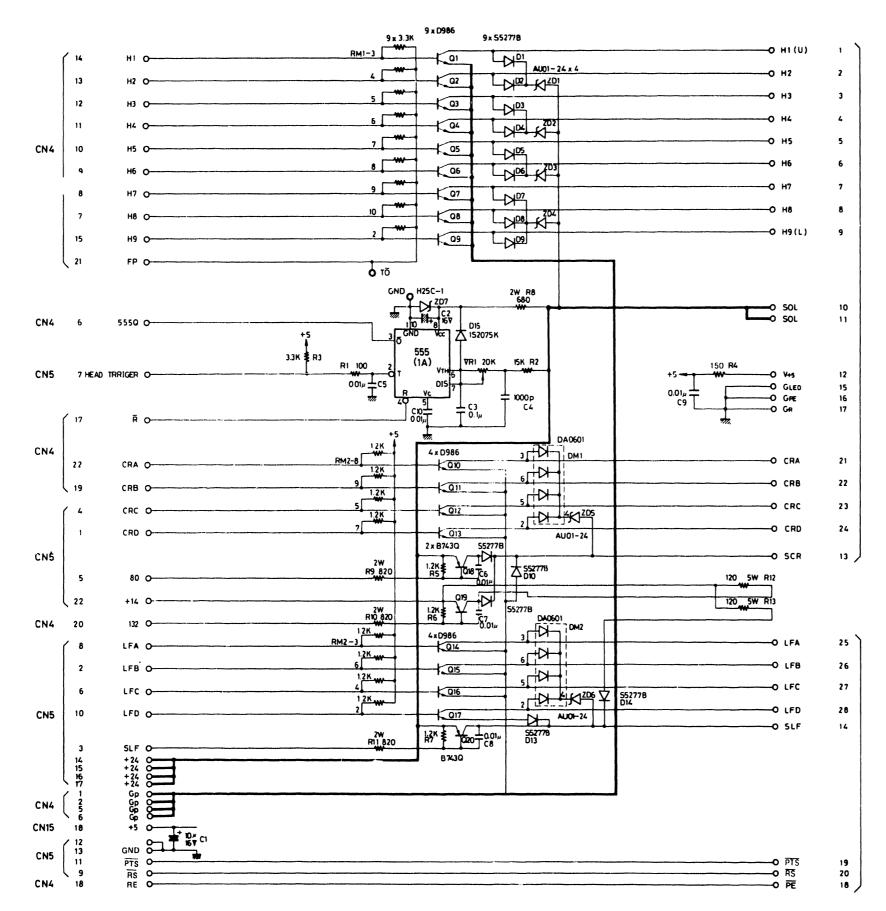
Fig. 5.2 Connection Diagram of Driver Circuit
