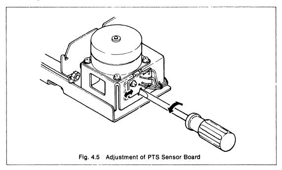
4.3.3 Adjustment of phase relationship between timing signal and reset signal Shift the home position sensor assembly to the right or left so that the phase relationship between timing signal PTS and reset signal RS becomes as shown in Fig. 4.6.
