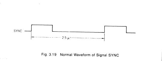
If signal SYNC is not properly output, replace the 8041 with a new one. (3) Trouble with 8155
