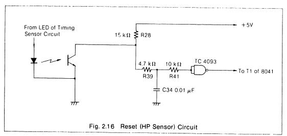
The output signal from the phototransistor used as the photocoupler is integrated and input to the Schmitt circuit which prevents the waveform of the output signal from being disturbed due to noise or mechanical vibrations.
