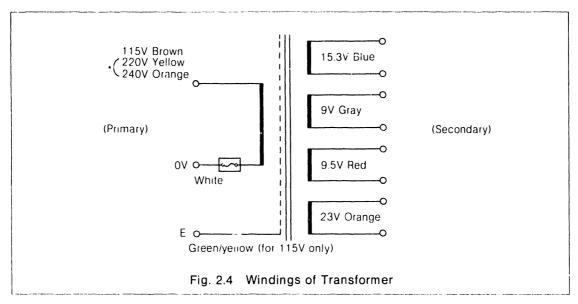
NOTE: The fourth pin (marked with "2") of the 5-pin connector on the primary side is used for selection of 220/240V. For 220V, insert the yellow wire into the fourth pin and the orange wire (240V) not used into the fifth pin (marked with "3").
