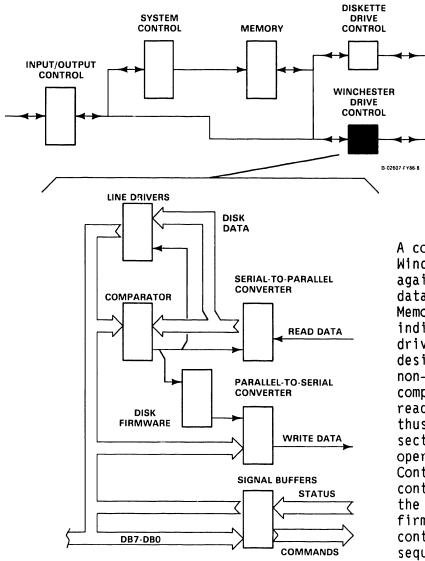
A comparator checks Winchester header data against updated header data stored in DPU Memory. A compare indicates that the drive head is over the desired sector. A non-compare causes the comparator to disable read/write circuits thus blocking invalid sector read/write operations. System Control issues disk control commands via the data bus. A disk firmware microprogram controls write sequencing.
