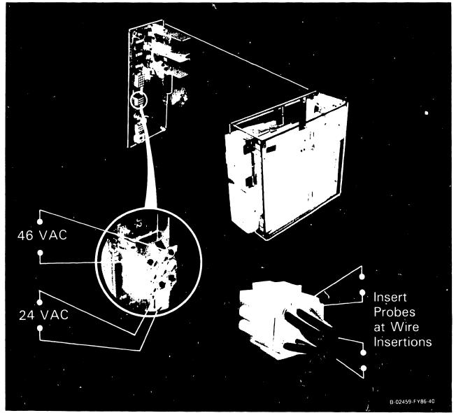
If ac voltages check OK, replace rectifier board. Should either .ac voltage fail, replace ftransformer.
