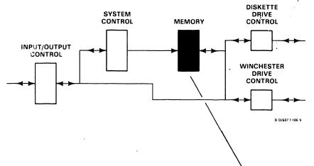
The addressing of 64 K-bytes requires 16 address bits. Two memory-address strobes, Row Address Strobe and Column Address Strobe, multiplex an 8-bit row address and an 8-bit column address into each chip to form, internally, a 16-bit address. The location thus selected either stores data bits DB7-DB0 from the data bus (memory write) or places the bits on the bus (memory read).
