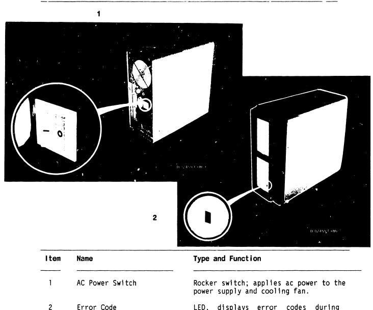
LED, displays error codes during power-up diagnostic.
