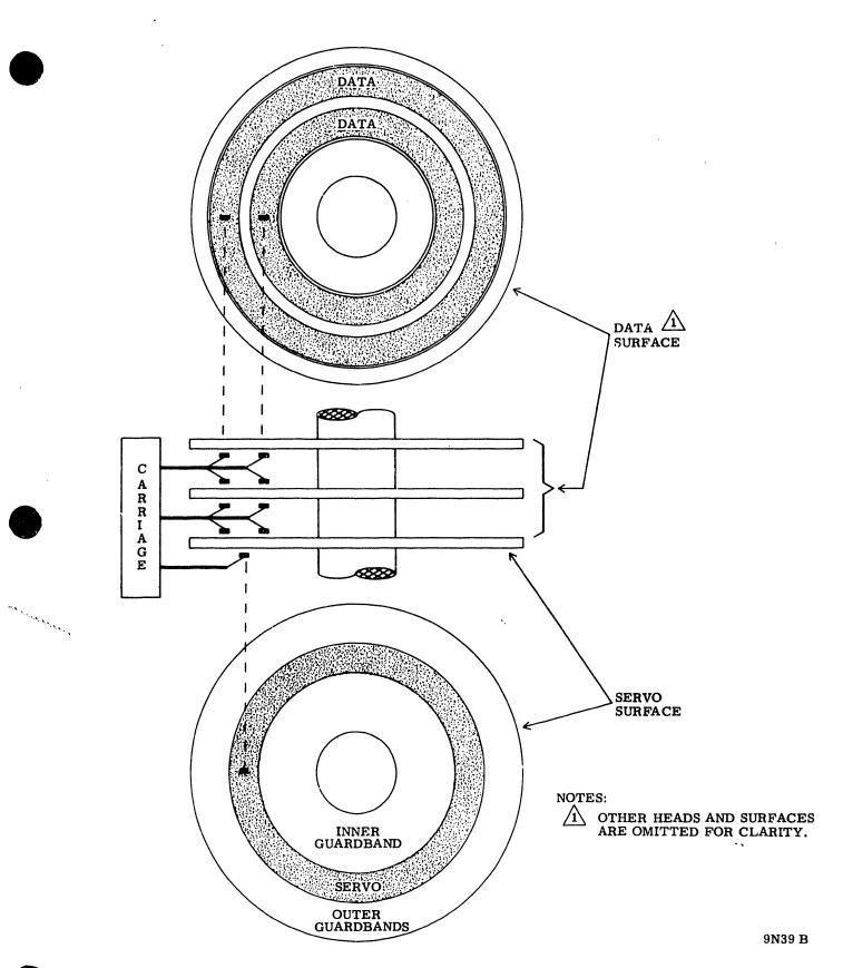
Figure 3-10. Servo to Data Surface Correlation
