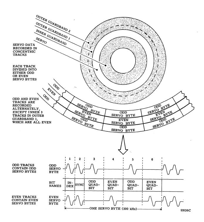
Figure 3-11. Servo Tracks and Bytes
