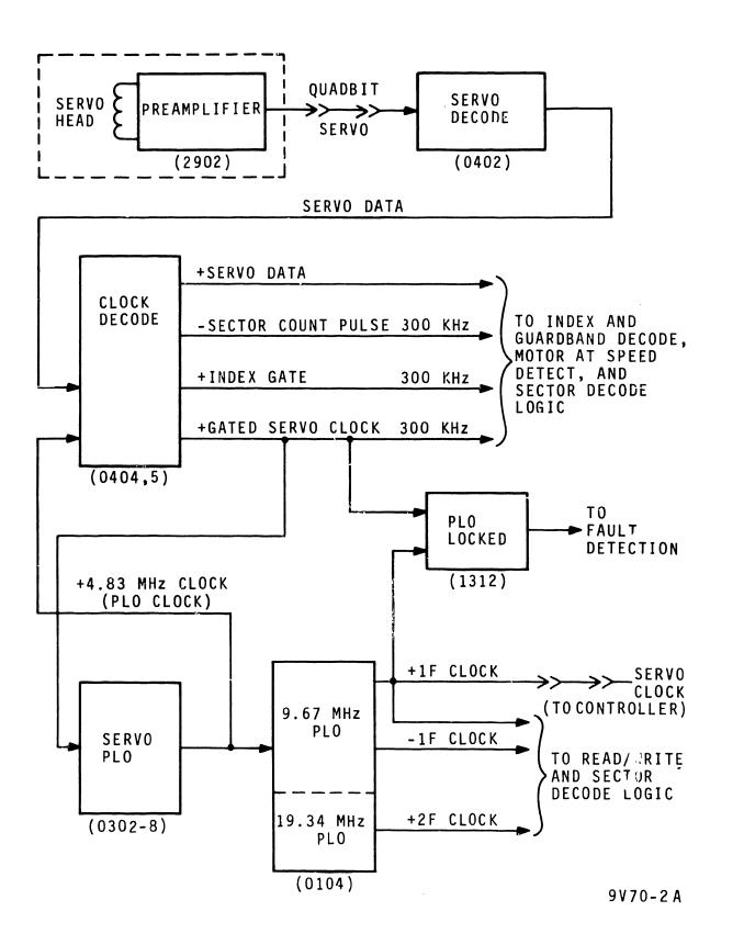
Figure 3-15. Servo Decode and Machine Clocks Locic
