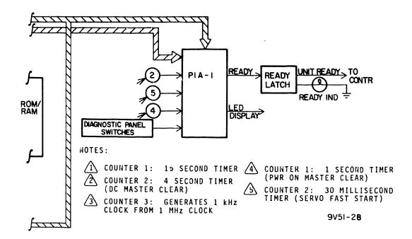
Figure 3-2. Power Sequencing Logic (Sheet 2)
