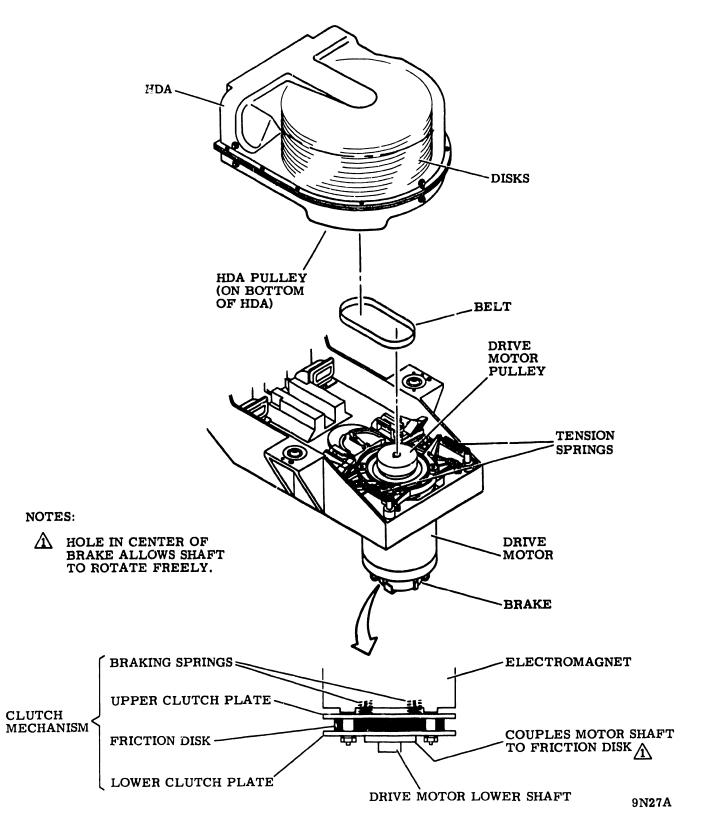
Figure 3-3. Disk Rotation Mechanism
