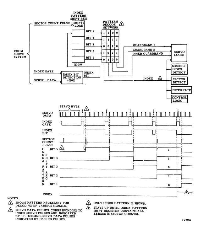
Figure 3-21. Guardband and Index Detection
