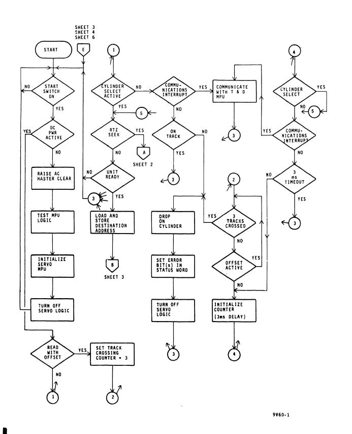
Figure 3-20. Servo Microprogram (Sheet 1 of 6)
