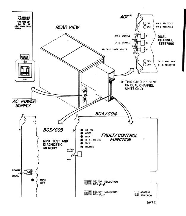
Figure 2-2. Switches and Indicators (Rear View)
