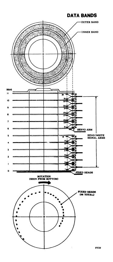
Figure 1-3. Head and Disk Assembly
