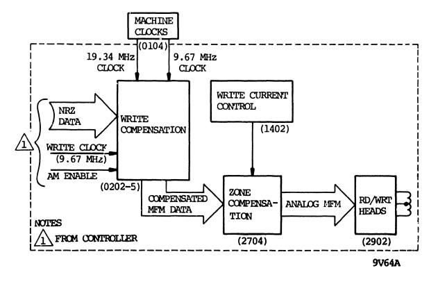
Figure 3-29. Write Logic
