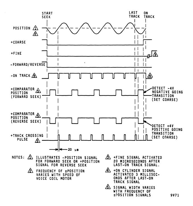
Figure 3-19. Servo System Timing
