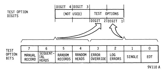
Figure A-1. Test Option Bits
