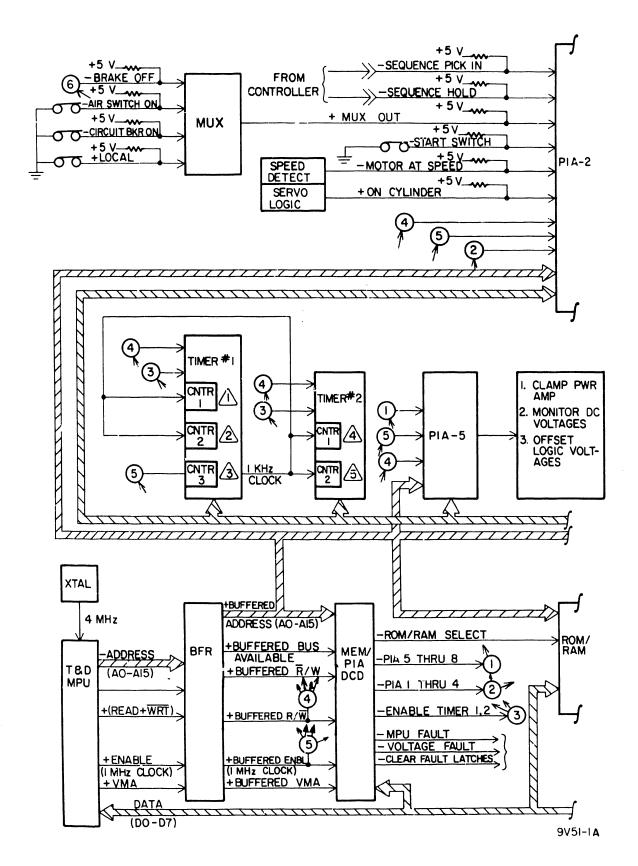
Figure 3-2. Power Sequencing Logic (Shect 1 of 2)
