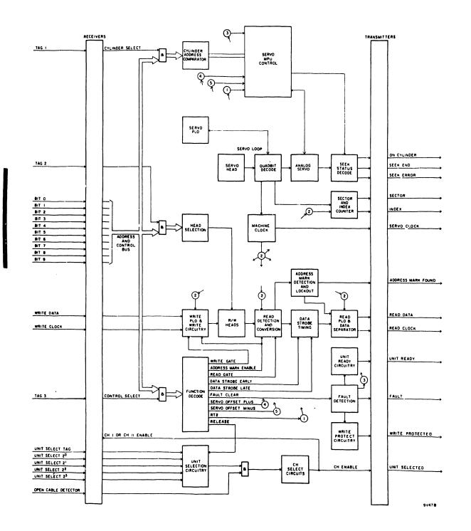
Figure 3-6. Signal Processing Block Diagram
