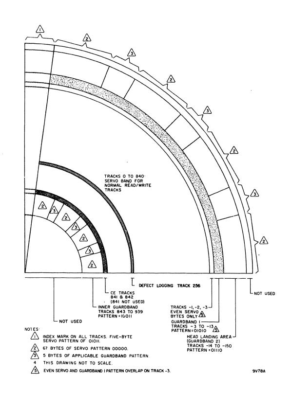
Figure 3-12. Servo Bands, Byte Layout
