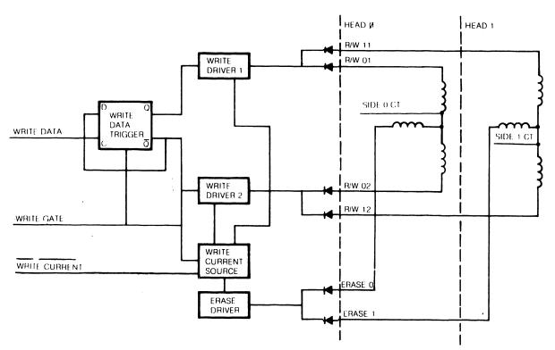
FIGURE 32. WRITE CIRCUIT FUNCTIONAL DIAGRAM
