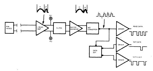
FIGURE 33. READ CIRCUIT FUNCTIONAL DIAGRAM
