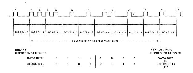
FIGURE 14. DELETED DATA ADDRESS MARK FM
