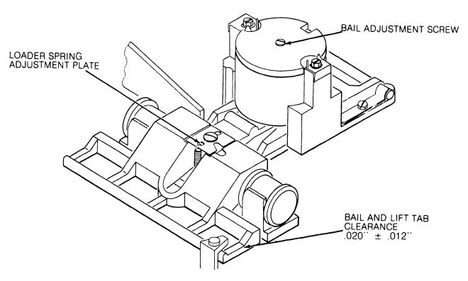
FIGURE 37. HEAD LOAD MECHANISM ADJUSTMENT
