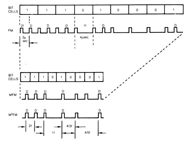
FIGURE 7. FM. MFM AND M<sup>2</sup>FM ENCODING
