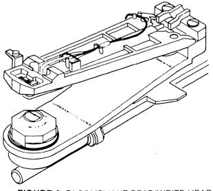
FIGURE 2. BI-COMPLIANT READ/WRITE HEAD
