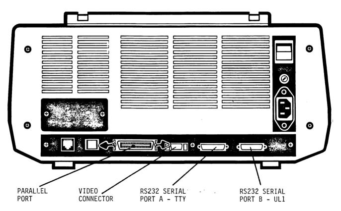
Figure 1 Victor 9000 Parallel and Serial Ports
