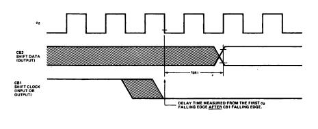
Figure H-5g: Timing for Shift In with Internal or External Shift Clocking
