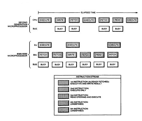
**Execution Unit** All registers and data paths in the EU are 16 bits wide, providing for fast internal transfers. CPU status and control flags are maintained in the EU by a 16-bit arithmetic/logic unit (ALU) that manipulates the general registers and the instruction operands (Figure 4).
