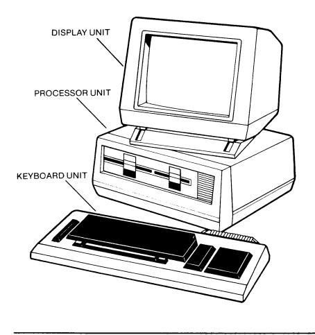
The system can be connected to a wide variety of peripherals and accommodates local and long distance communications. Standard interfaces include a parallel port (Centronics or IEEE-488), programmable RS-232(V-24) channels, an internal control port, and an audio controller for digitized voice and tone output.
