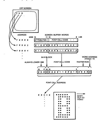
**FONT POINTER** The words in the screen buffer are broken into two pieces. The lower 11 bits comprise the font pointer. The upper five bits are attribute bits. The font pointer contains binary address information. Up to 2048 characters, or font cells, can be displayed on the screen.
