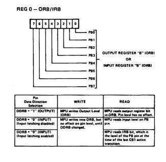
Figure H-9: Output Register B (ORB), input Register B (IRB)
