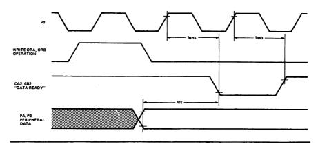
Figure H-5d: CA2, CB2 Timing for Write Handshake, Handshake Mode
