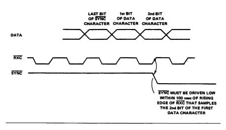
Figure G-2.3 SYNC Output, External Synchronization
