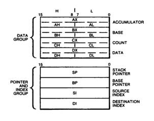
The data registers are unique in that their upper (high) and lower halves are separately addressable. Each data register can be used interchangeably as a 16-bit register or as two 8-bit registers. However, the CPU registers are always accessed as 16-bit units. Data registers can be used without constraint in most arithmetic and logic operations. Certain instructions use specified registers implicitly (see Table 1), allowing compact, powerful encoding.
