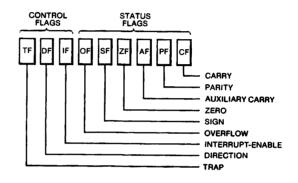
8080/8085 Register and Flag Correspondence The registers, the flags, and the program counter in the 8080/8085 CPUs have counterparts in the 8088 CPU (see Figure 8). The A register (accumulator) in the 8080/8085 corresponds to the AL register in the 8088. The 8080/8085 H&L, B&C, and D&E registers correspond to registers BH, BL, CH, CL, DH, and DL, respectively, in the 8088. The 8080/8085 stack pointer (SP) and program counter (PC) correspond to the 8088 SP and IP.
