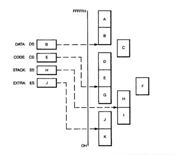
Individual applications define and use segments differently. The currently-addressable segments provide a generous work space: 64K bytes for code, a 64K byte stack, and 128K bytes of data storage. Many applications can be written that simply initialize the segment registers and then forget them. However, large applications should be designed with careful consideration given to segment definition.
