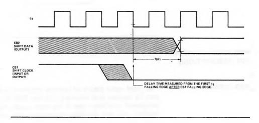
Figure H-5g: Timing for Shift In with Internal or External Shift Clocking
