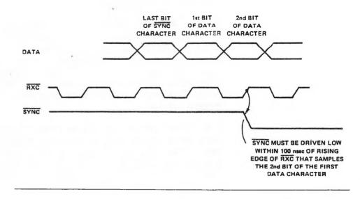
Figure G-2.4 SYNC Output, Internal Synchronization
