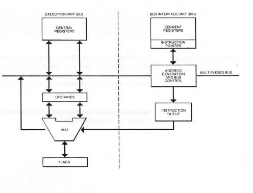
The EU is not connected to the outside world via the system bus. It obtains instructions from a queue maintained by the BIU. When an instruction requires access to memory or to a peripheral device, the EU sends a request to the BIU to store or obtain the data. The BIU performs an address relocation that gives the EU access to a full megabyte of memory space.
