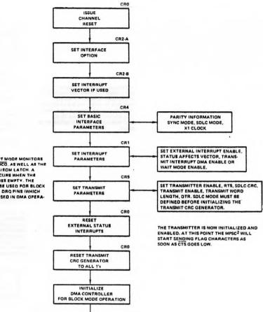
THE EXTERNAL INTERRUPT MODE MONITORS THE STATUS OF CTS AND OCO. AS WELL AS THE STATUS OF IX UNDERRUNFOM LATCH A TRANSMIT NUTFRUPT OCCURS WHEN THE TRANSMIT BULFFER SECOMES EMPTY. THE EXTERNAL WAIT PIN CAN BE USED FOR BLOCK MODE TRANSFERS ON THE DRO PINSI WHICH ARE EXTERNALI CAN BE USED IN DMA OPERA-TION AS WELL.
