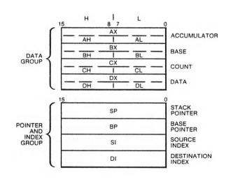
The data registers are unique in that their upper (high) and lower halves are separately addressable. Each data register can be used interchangeably as a 16-bit register or as two 8-bit registers. However, the CPU registers are always accessed as 16-bit units. Data registers can be used without constraint in most arithmetic and logic operations. Certain instructions use specified registers implicitly (see Table 1), allowing compact, powerful encoding.
