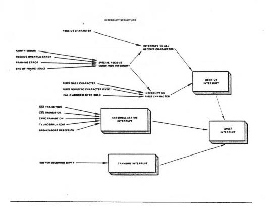
Figure G-4.7 illustrates the action of the interrupt control logic during an interrupt acknowledge sequence.
