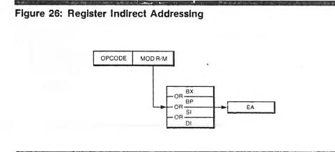
NOTE: Any 16-bit general register can be used for register indirect addressing with the JMP or CALL instructions.
