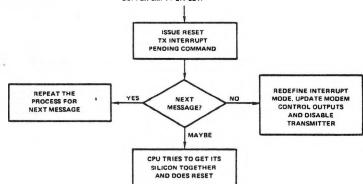
THE FIRST INTERRUPT WILL OCCUR WHEN THE CT3 PIN BECOMES ACTIVE, AT WHICH POINT THE MPSC<sup>2</sup> WILL START TRANS-MITTING FLAG CHARACTERS. THE CPU WILL RESPOND TO THIS INTERRUPT BY ISSUING THE FIRST BYTE (ADDRESS FIELDI TO THE MPSC<sup>2</sup>.
