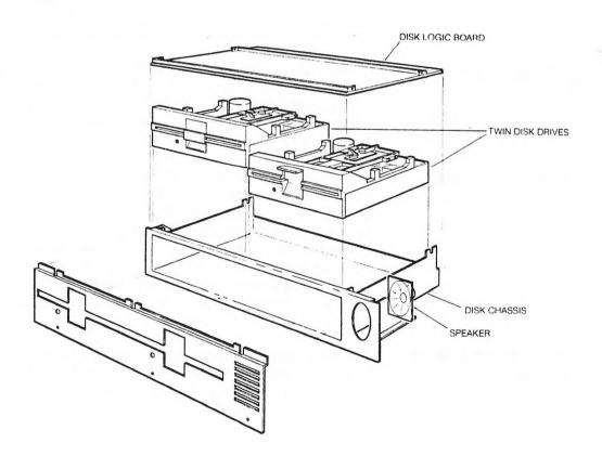
The standard drive units are 5-1/4 inch, 80-track mechanisms, which operate with single-sided media. Track density is 96 tracks per inch, and recording density is maintained at approximately 8000 bits per inch on all tracks.
