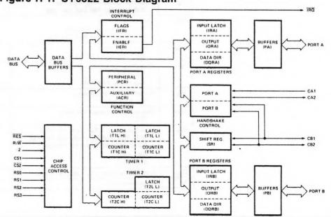
Figure H-1: SY6522 Block Diagram
