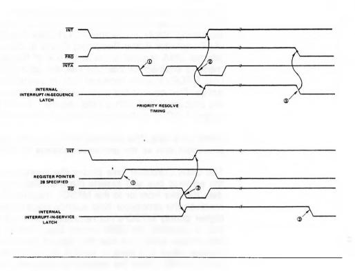
At the beginning of the first Interrupt Acknowledge cycle, the interrupt prioritization logic is frozen to permit any late interrupt requests by higher priority devices to ripple through and resolve internal priorities before the second interrupt pulse.
