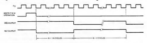
Note: A precaution to take in the use of PB7 as the timer output concerns the Data Direction Register contents for PB7. Both DDRB bit 7 and ACR bit 7 must be 1 for PB7 to function as the timer output. If one is 1 and the other is 0, then PB7 functions as a normal output pin, controlled by ORB bit 7.
