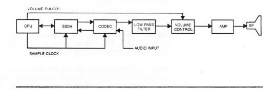
The synchronous serial data adapter (SSDA) is the major interface between the CPU and the audio section. The main function of the SSDA in playback mode is the buffering and conversion of 8-bit bytes into a serial bit stream for the Codec. In the record mode, the SSDA also converts a serial bit stream from the Codec into bytes for the CPU.
