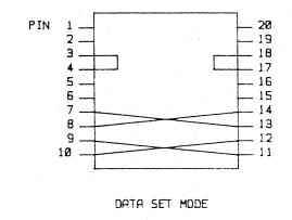
Figure 5.6 : SBX Header Configuration
